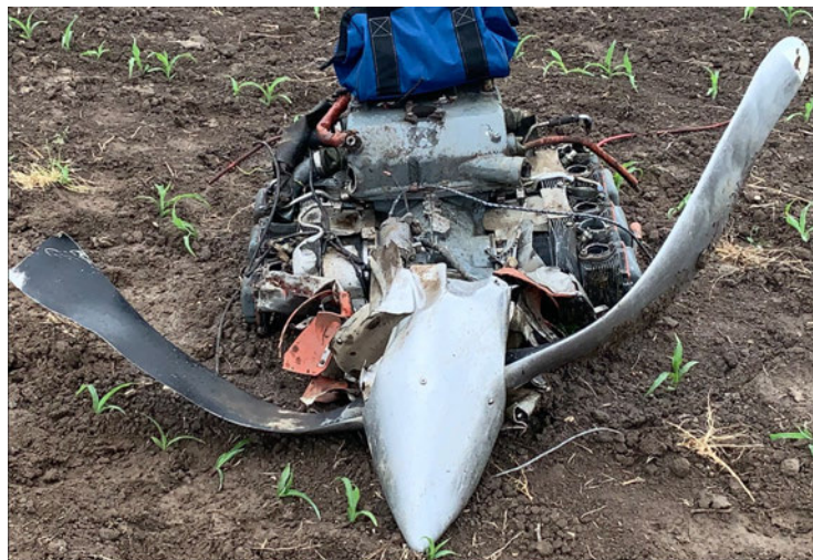
Figure 5 Hartzell propeller exhibiting signs of s bending and polishing.
