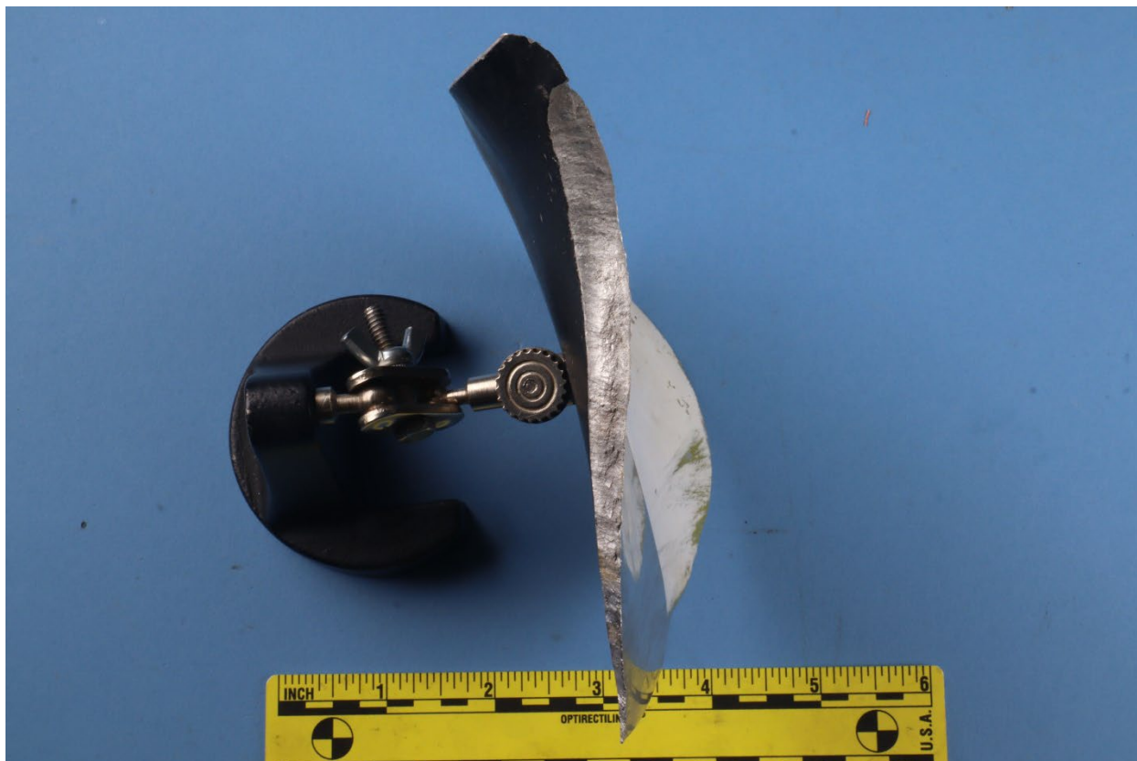
Figure 2. Fracture surface of separated propeller tip.
