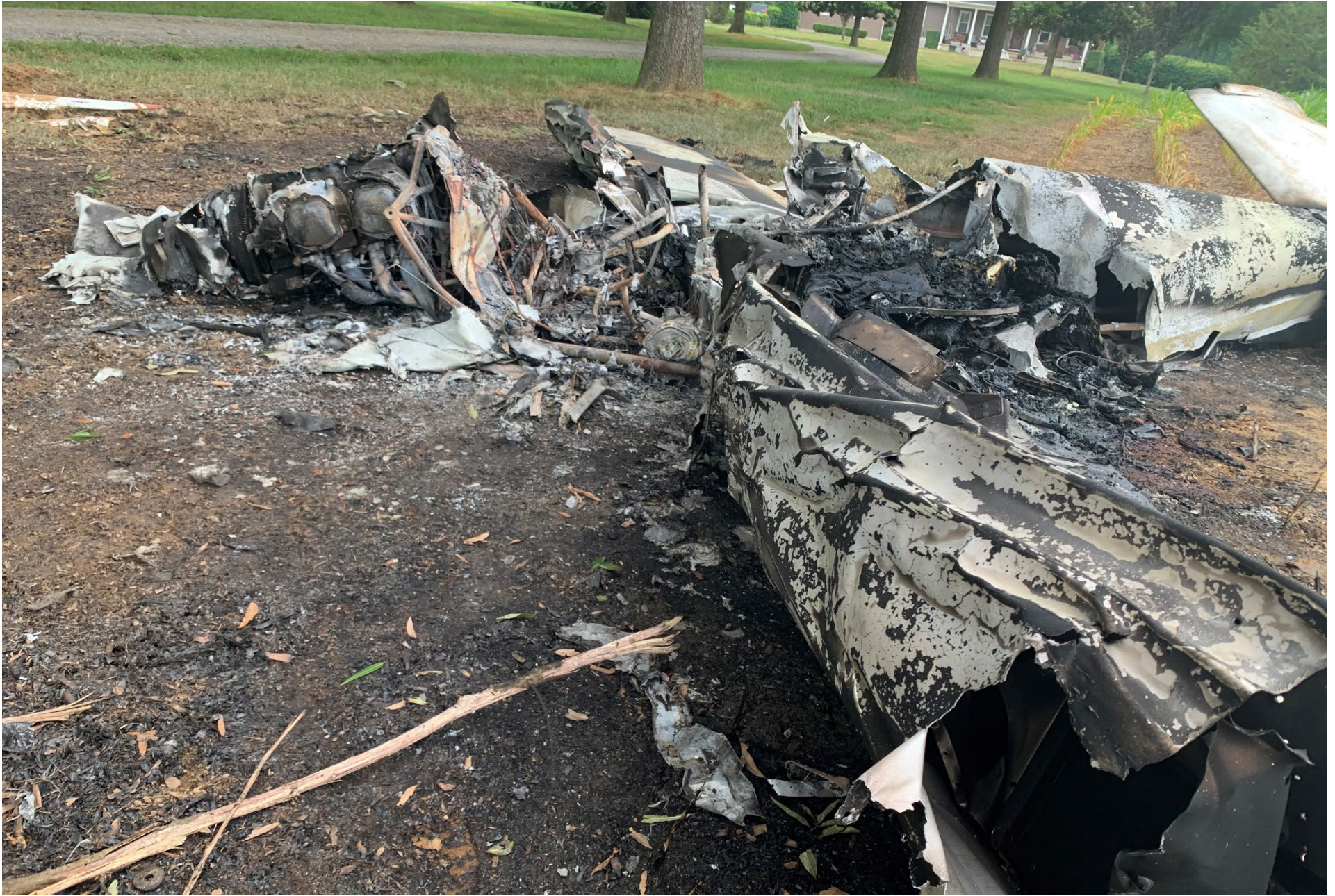
Photo 3 – Main wreckage, view from left wing, note accordion crushing on leading edge
