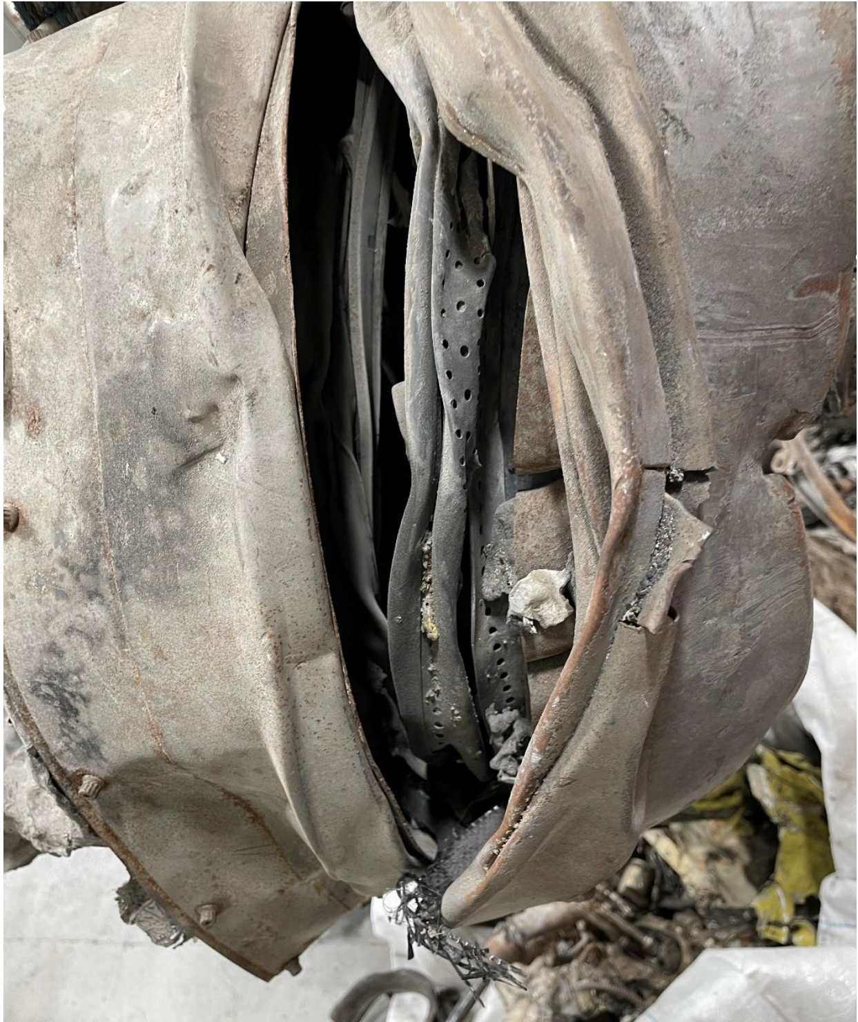
Figure 32. Photo of engine B case separation.
