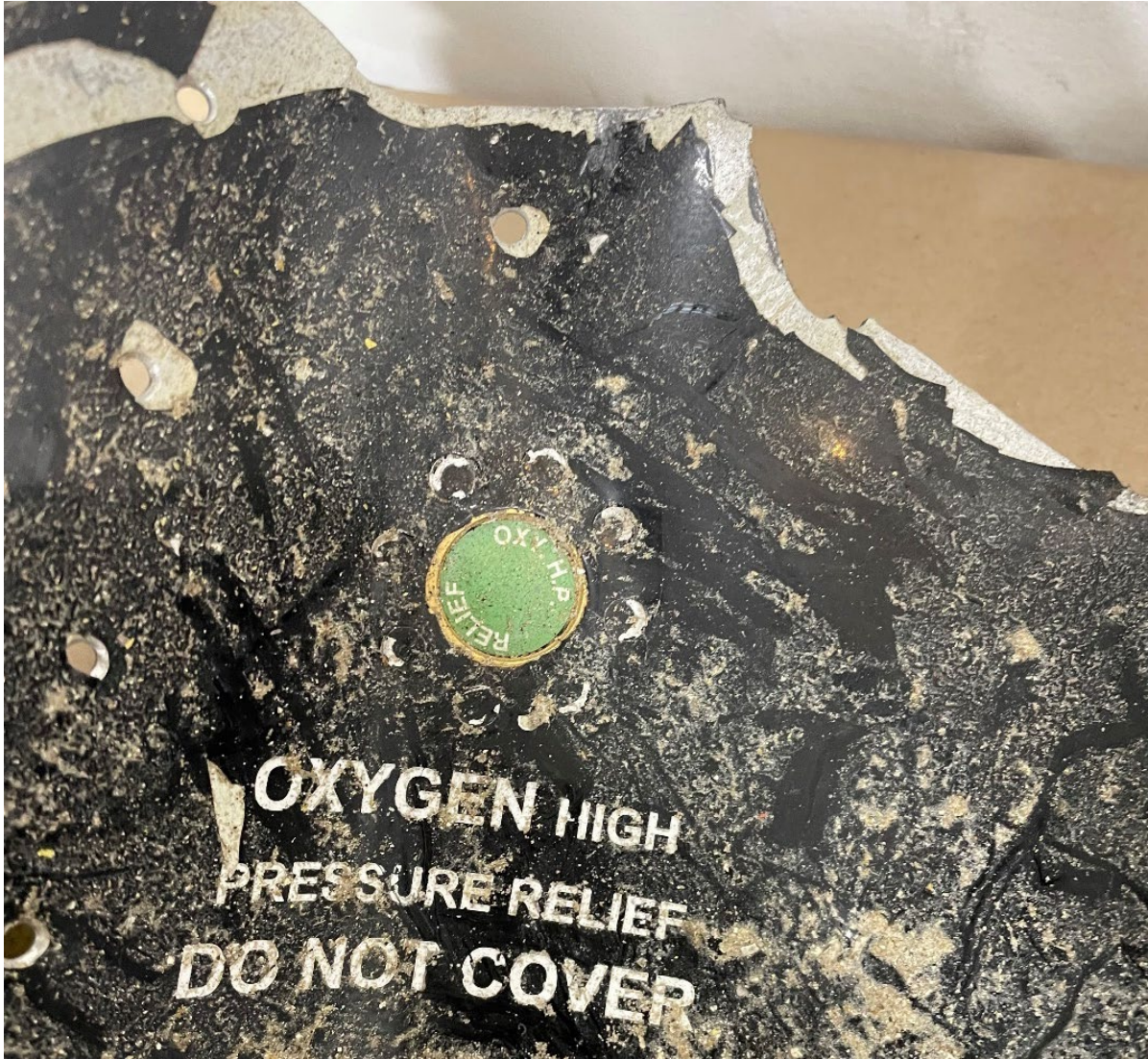
Figure 20. Photo of oxygen high pressure relief valve overboard discharge indicator.
