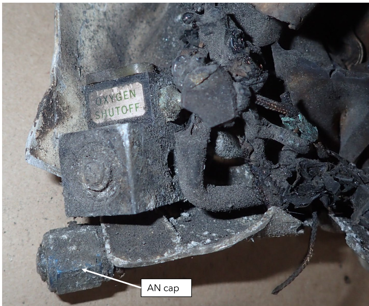
Figure 22. Photo of passenger oxygen mask stowage/dropout box assembly with AN cap installed.
