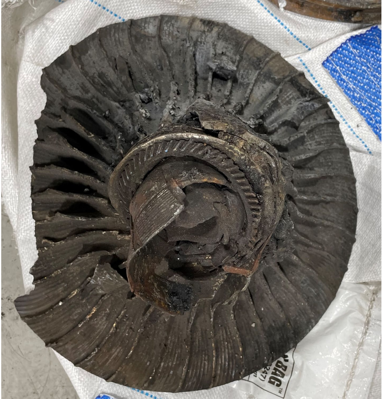
Figure 26. Photo of engine A compressor impeller.
