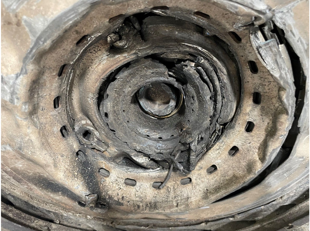
Figure 25. Photo of engine A compressor diffuser.
