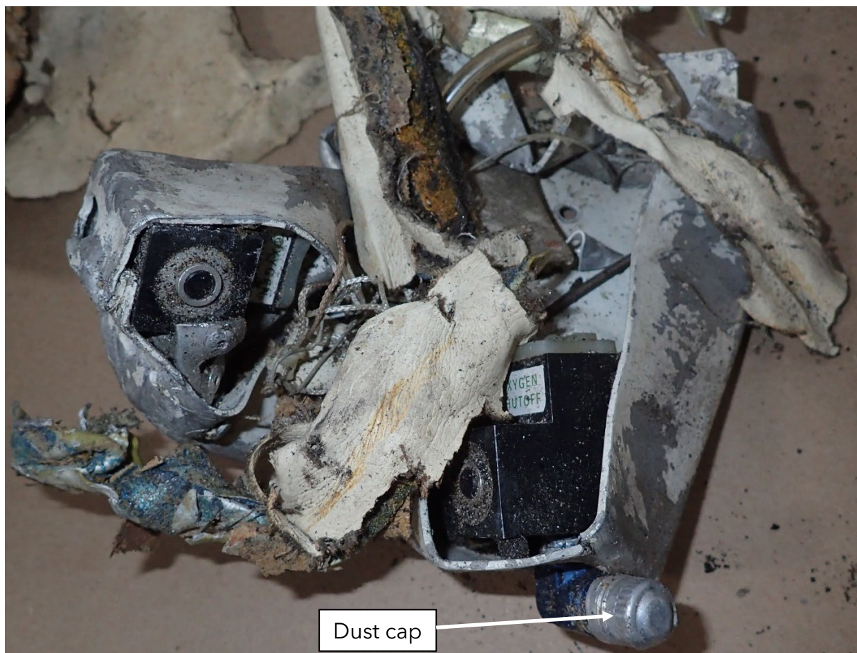
Figure 21. Photo of passenger oxygen mask stowage/dropout box assembly with dust cap installed.
