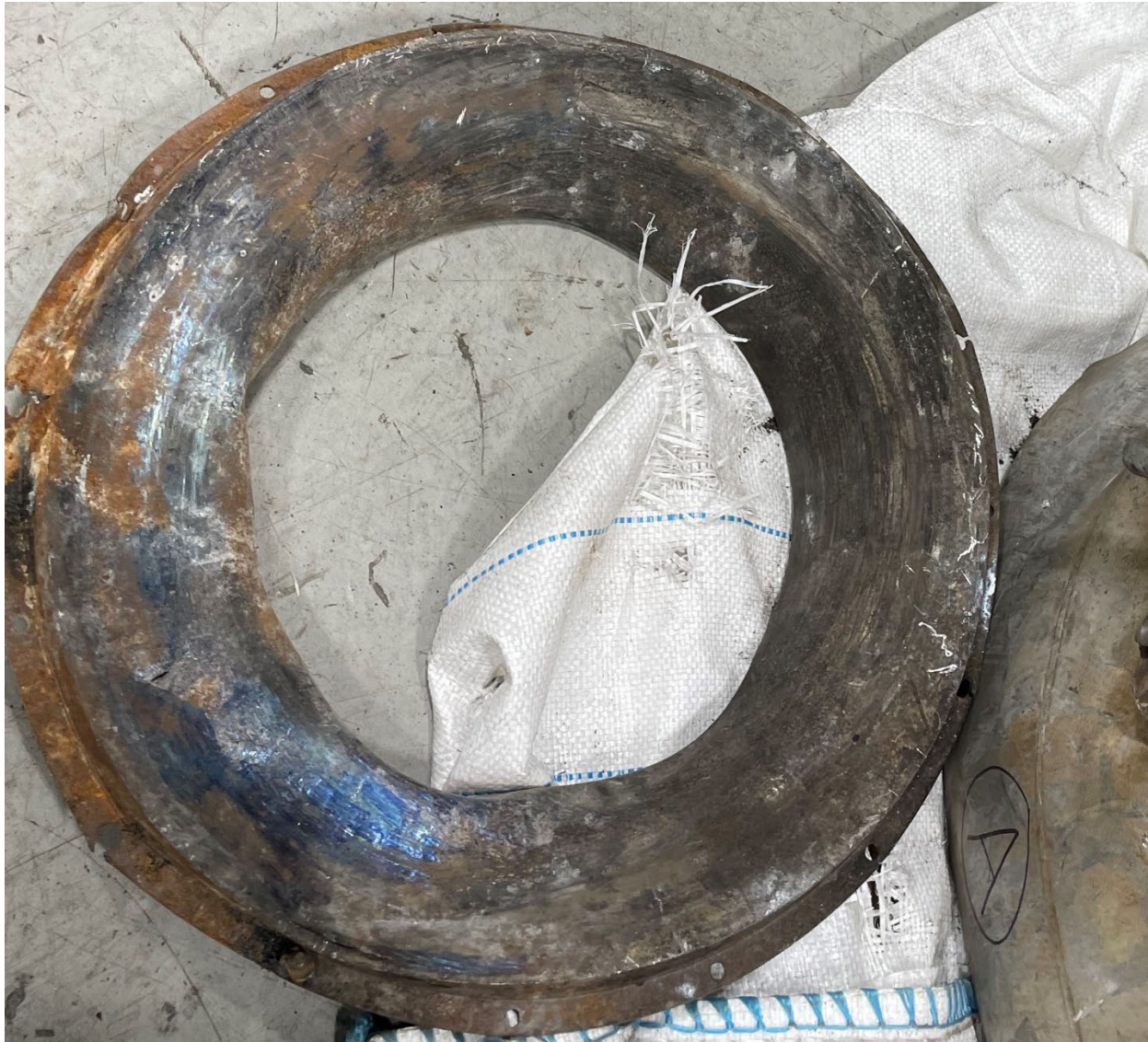
Figure 27. Photo of engine A HPC impeller shroud.
