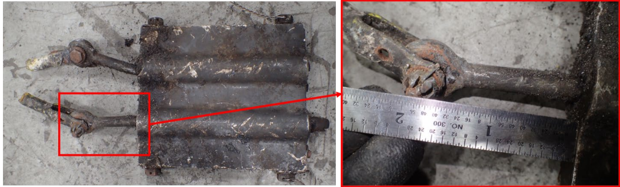
Figure 17. Photo of rudder trim actuator.
