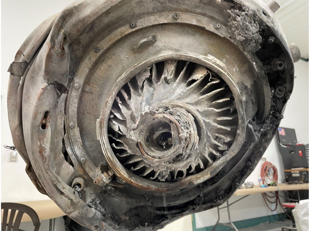
Figure 31. Photo of engine B compressor impeller.
