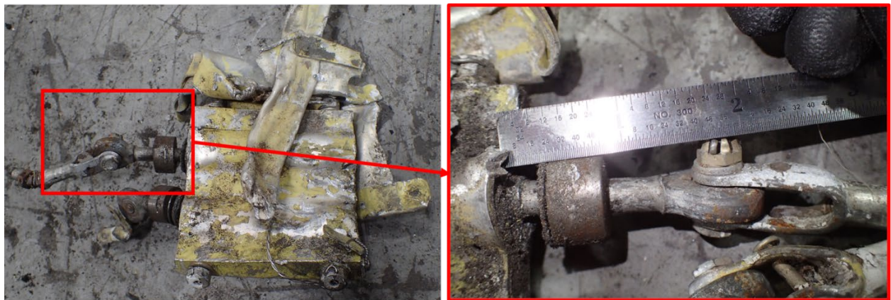
Figure 18. Photo of aileron trim actuator.
