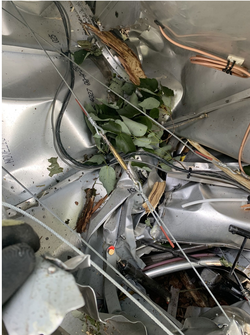
Photograph 6 - View of flight control cables and turnbuckles. (NTSB)
