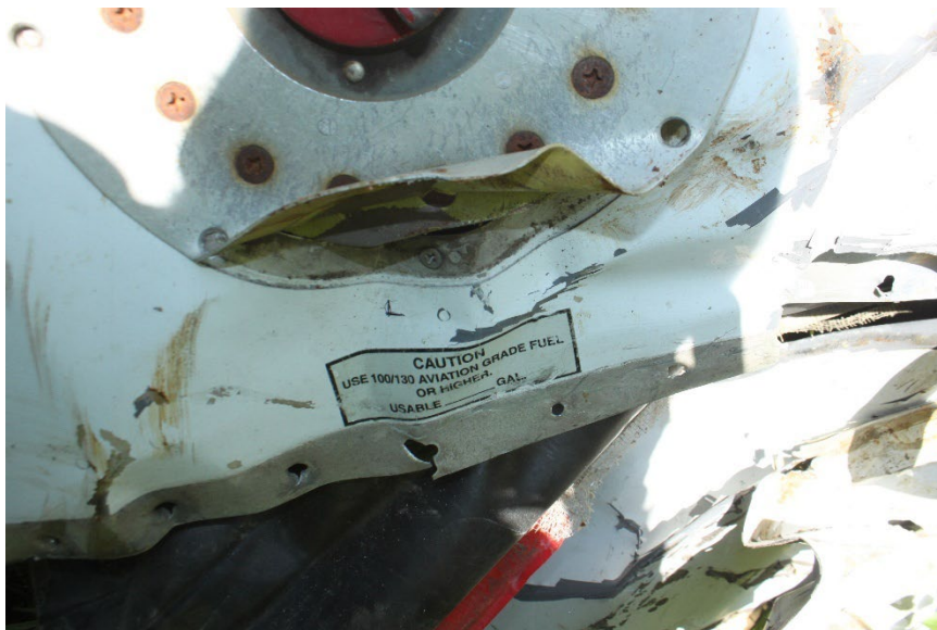
Figure 5 View of the Placard Adjacent to the Left Fuel Filler Cap
