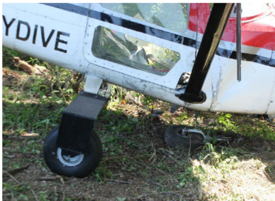
Figure 8 View of Right Main Landing Gear and Separated Nose Wheel Assembly and lower Strut
