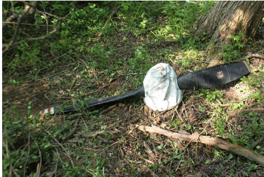
Figure 17 View of the Separated Propeller with Attached Crankshaft Flange
