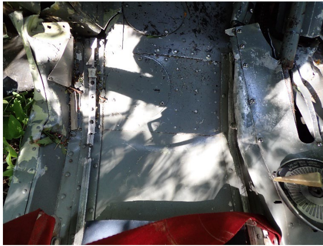
Figure 10 View of Pilot's Floor and Seat Tracks
