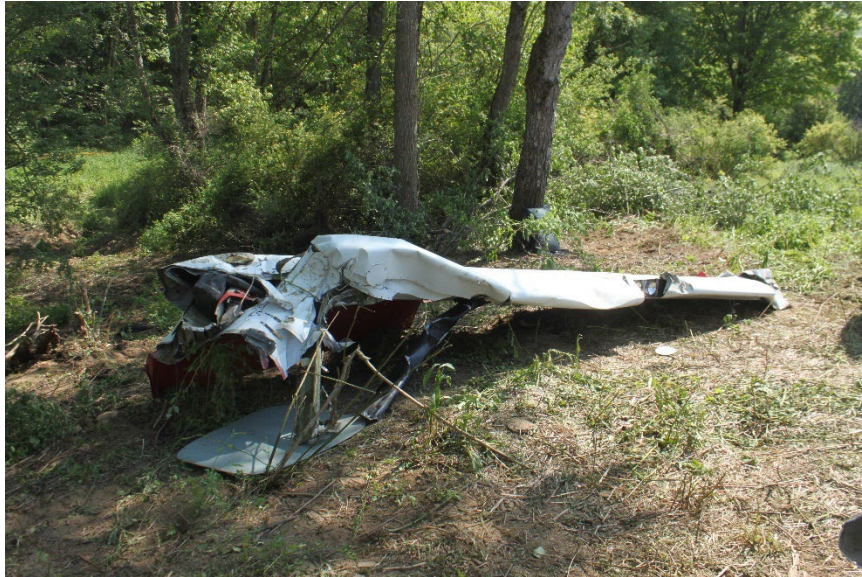
Figure 4 Frontal View of the Separated Left Wing Following Extraction From The Resting Position
