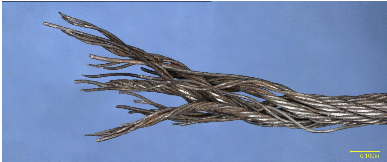
Figure 4 End 2 S (20X). View Showing Flat Areas on Cable Strands
