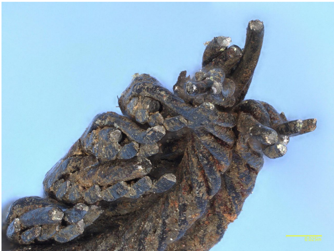
Figure 5 End 1 Fracture Surfaces S (50X). View of thinning of Cable Strands Adjacent to Area with External Rub
