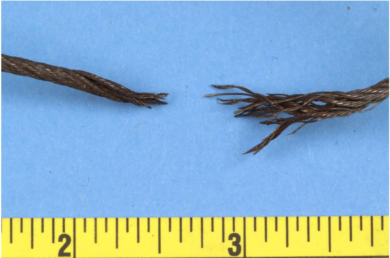
Figure 2 IMG_0032. View Showing the Condition of each Fractured End of the Cable
