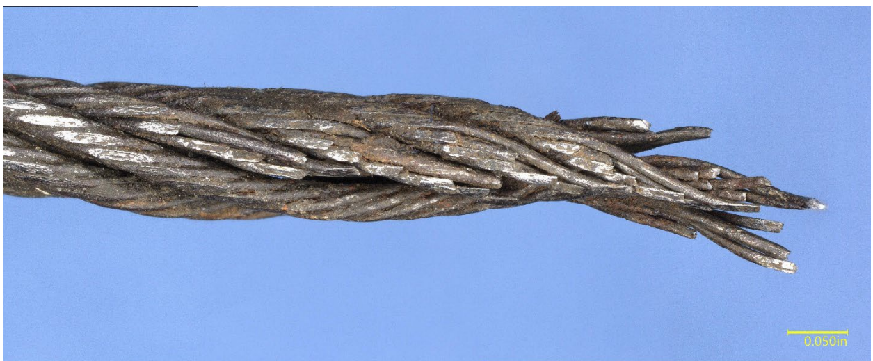
Figure 3 End 1 S (30X) View Showing Flat Areas on Cable Strands
