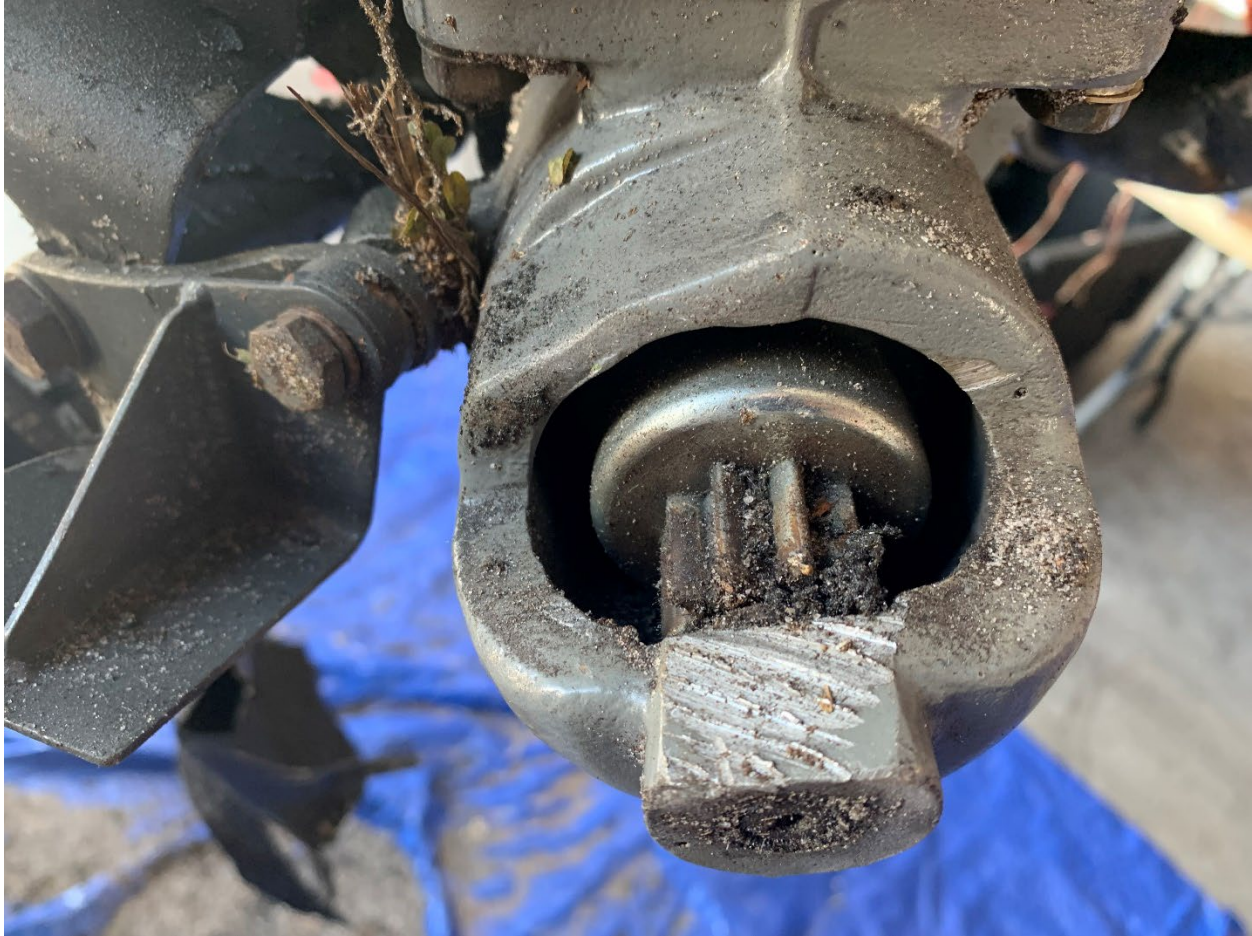
Figure 11. Engine starter. Note rotational scoring.
