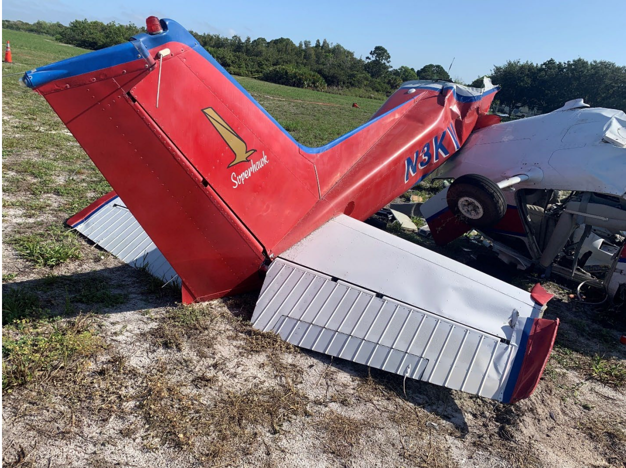
Figure 3. View of right horizontal stabilizer, right elevator, rudder, and vertical stabilizer.
