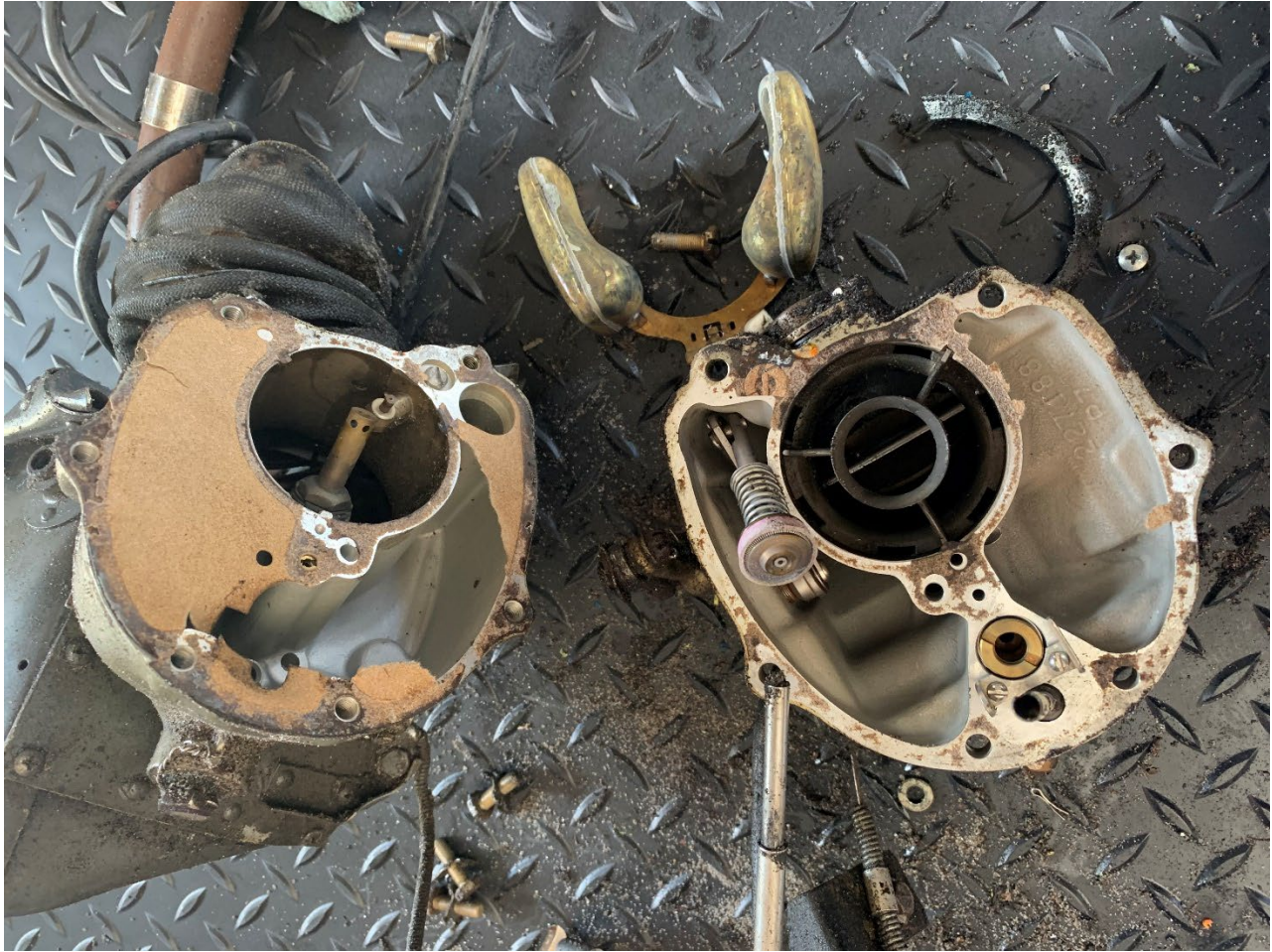
Figure 13. View of disassembled carburetor.
