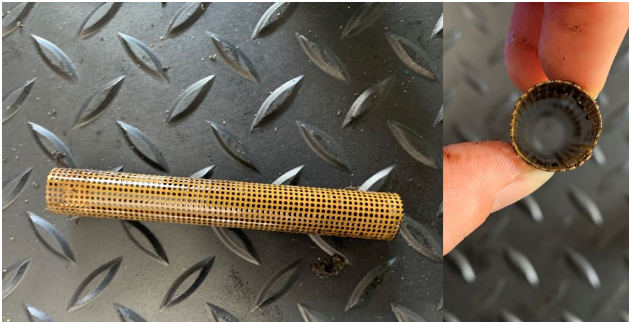
Figure 15. View of oil pickup screen.
