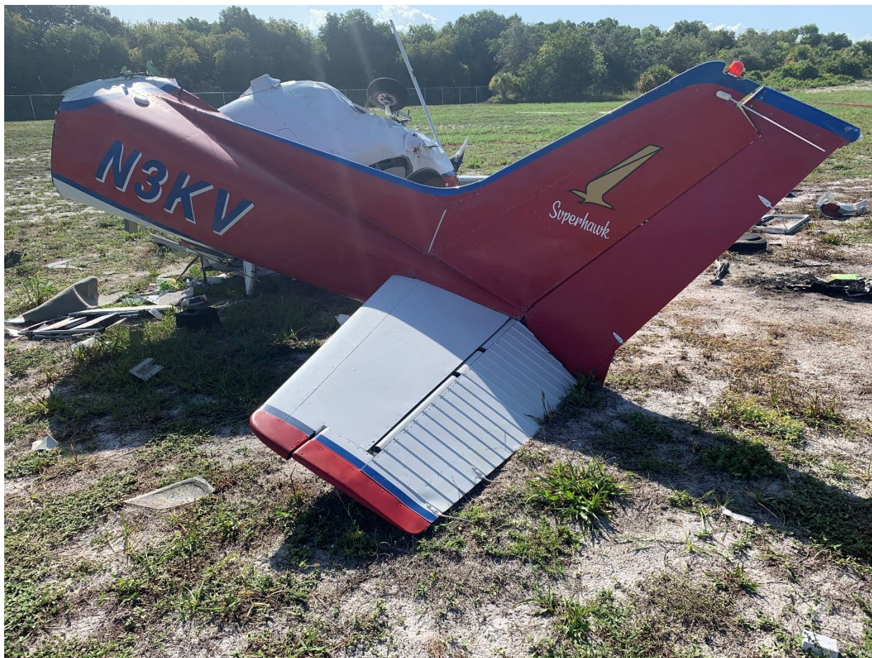
Figure 4. View of left horizontal stabilizer and left elevator along with the left side of the rudder and vertical stabilizer.
