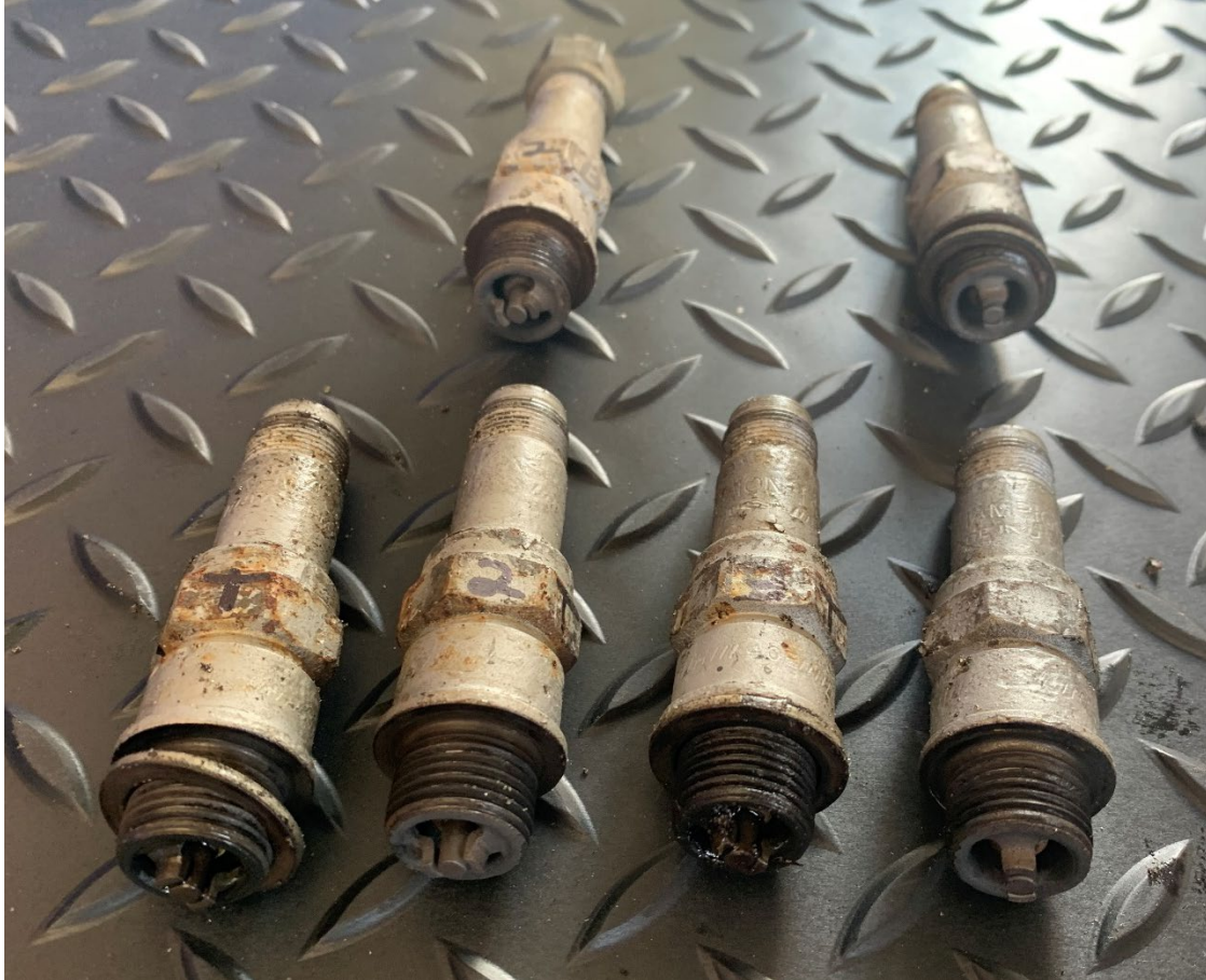
Figure 12. Spark plugs removed from engine.
