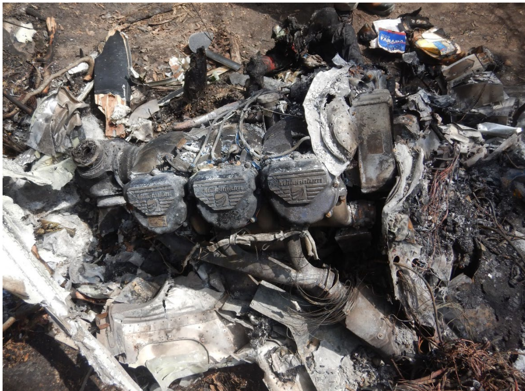
Photo 9 - View of engine, propeller hub, and fractured propeller blade
