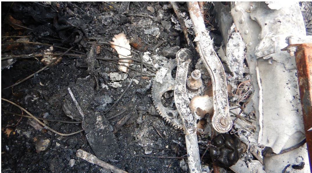
Photo 7 - View of landing gear mechanism indicating that gear were in the UP position
