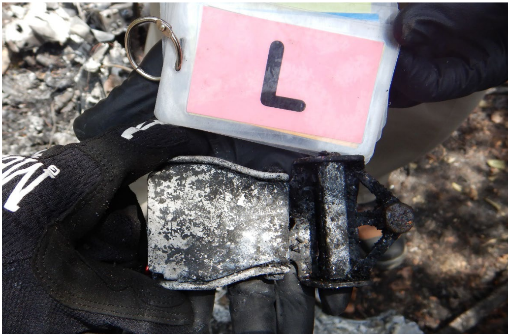
Photo 13 - View of left front seatbelt latch
