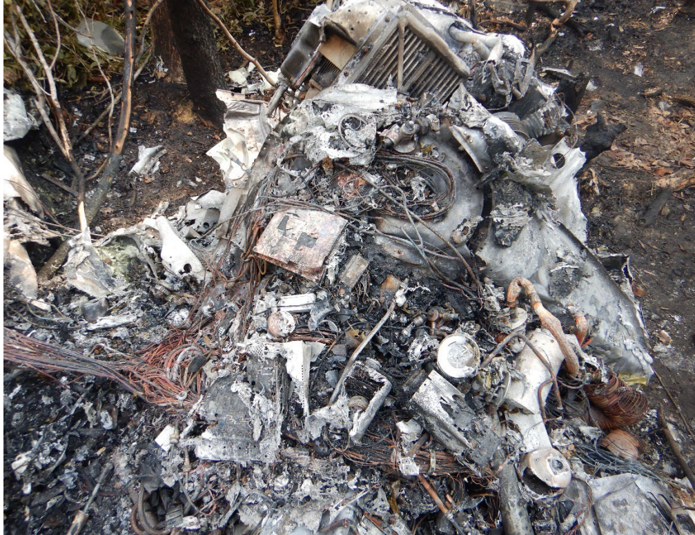
Photo 12 - View of thermally damaged cockpit and instruments
