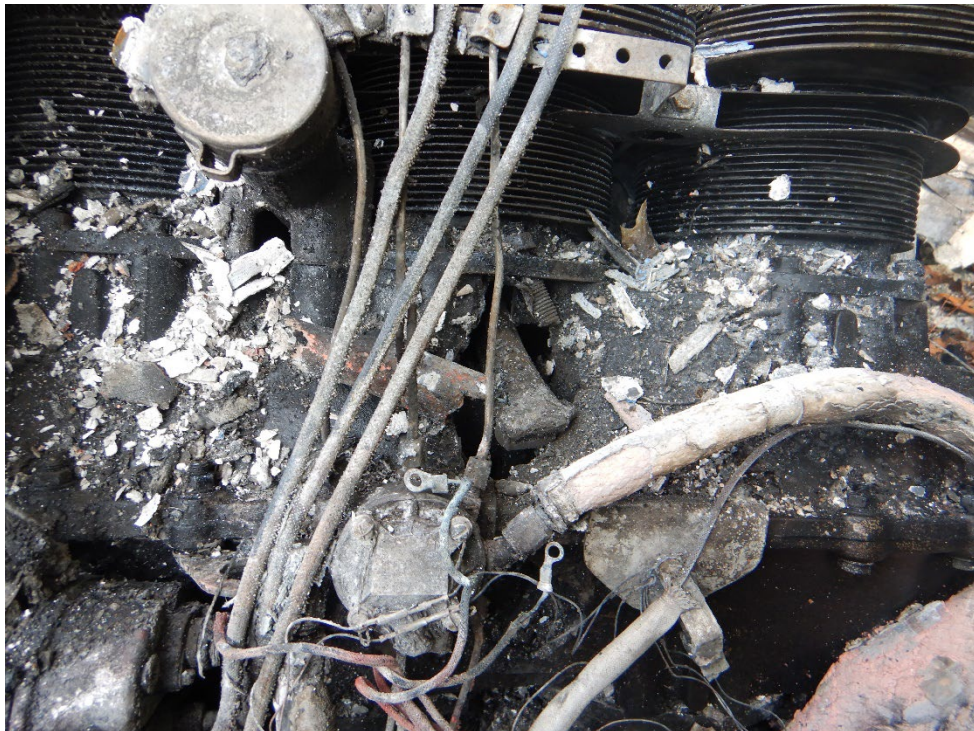
Photo 11 - View of hole of crankcase at cylinder No. 4 with connecting rod exposed
