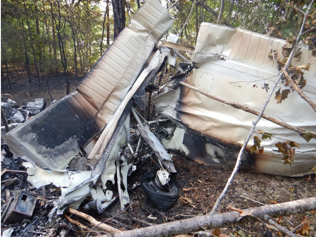
Photo 6 - View of fractured right wing with thermal damage
