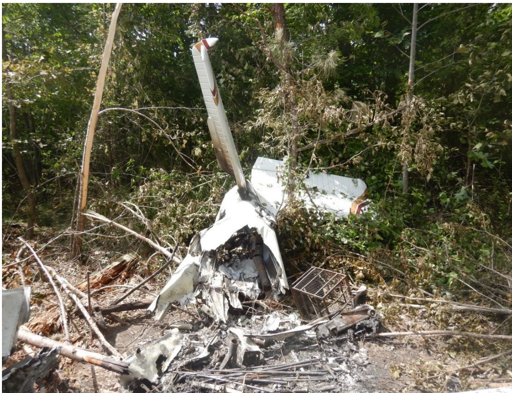
Photo 5 - View of the empennage and burned fuselage.
