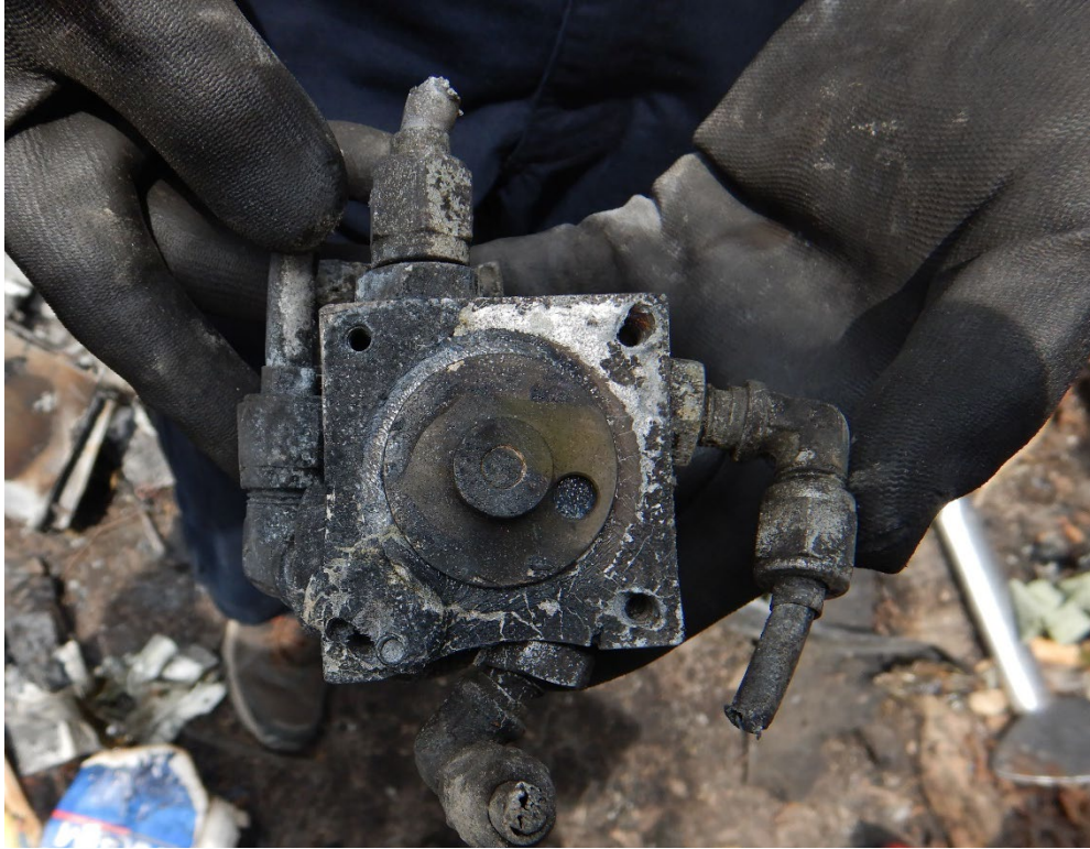
Photo 8 - View of fuel selector valve in closed position
