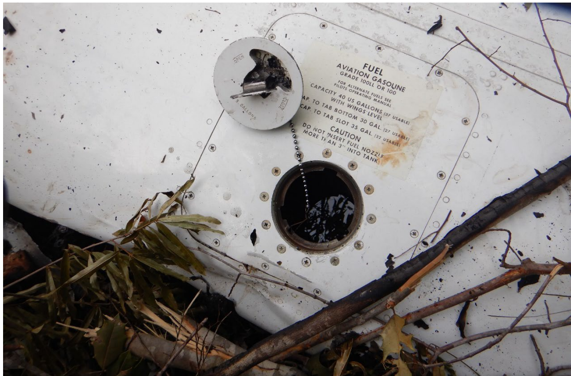
Photo 4 - View of left wing fuel tank with fuel cap removed.
