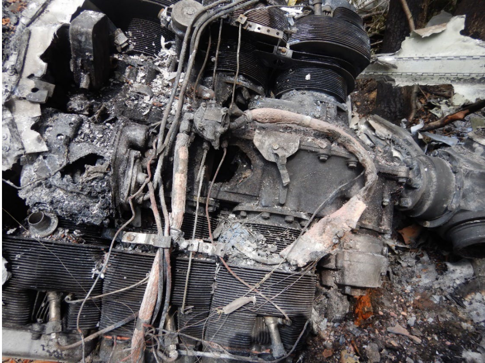
Photo 10 - View of top of engine with holes in crankcase above cylinder Nos. 3 and 4
