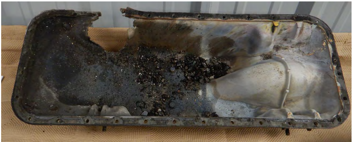
Photo 4 - Metal debris in impact damaged oil sump pan.
