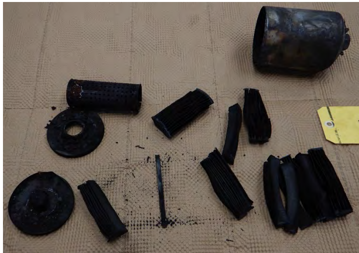
Photo 12 - Disassembled thermally damaged oil filter.
