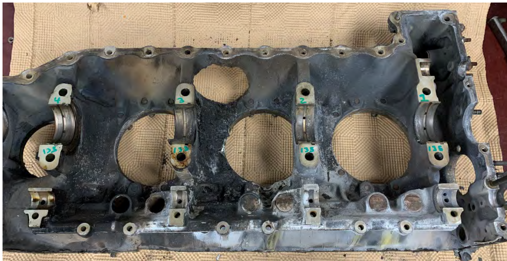
Photo 17 - View of open crankcase and main bearings for cylinder Nos. 5,3 and 1(left to right), note lifters that could not be removed.
