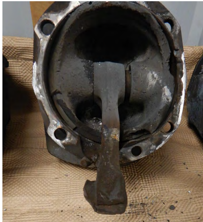
Photo 20 - Cylinder No. 4 with piston and connecting rod (note fracture at the piston skirt).
