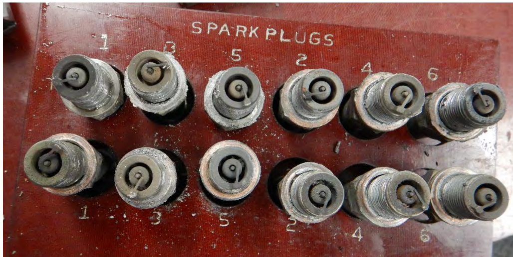
Photo 13 - Spark plugs with no evidence of detonation.
