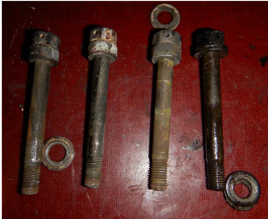
Photo 9 - Lower crankcase splitline bolts unapproved parts and spacers.
