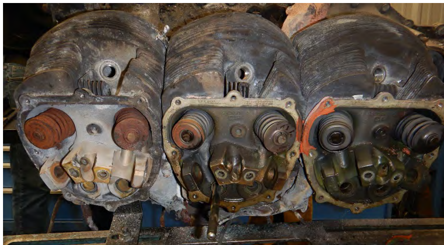
Photo 14 - Cylinder Nos. 1,3, 5 with rocker arms and covers removed.
