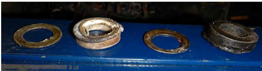
Photo 10 - Unapproved pushrod housing seals for cylinder No. 4
