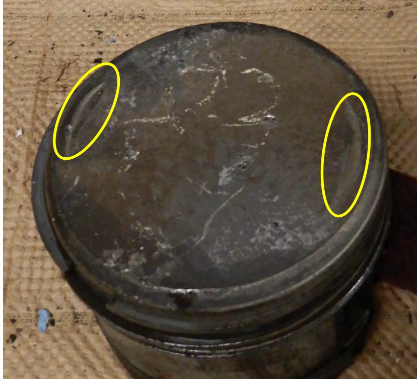
Photo 21 - Cylinder No. 4 piston with valve strike marks (circled in yellow).
