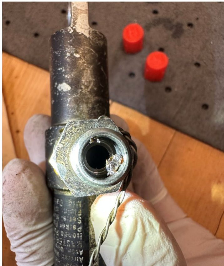
Figure 23: FOD in outlet port fitting of the pilot right master cylinder. Picture courtesy of Honda.
