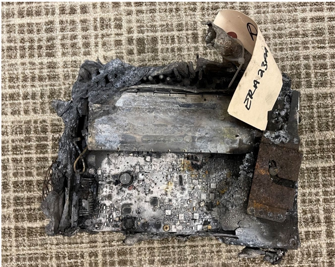
Figure 12: Right side integrated avionics computer
