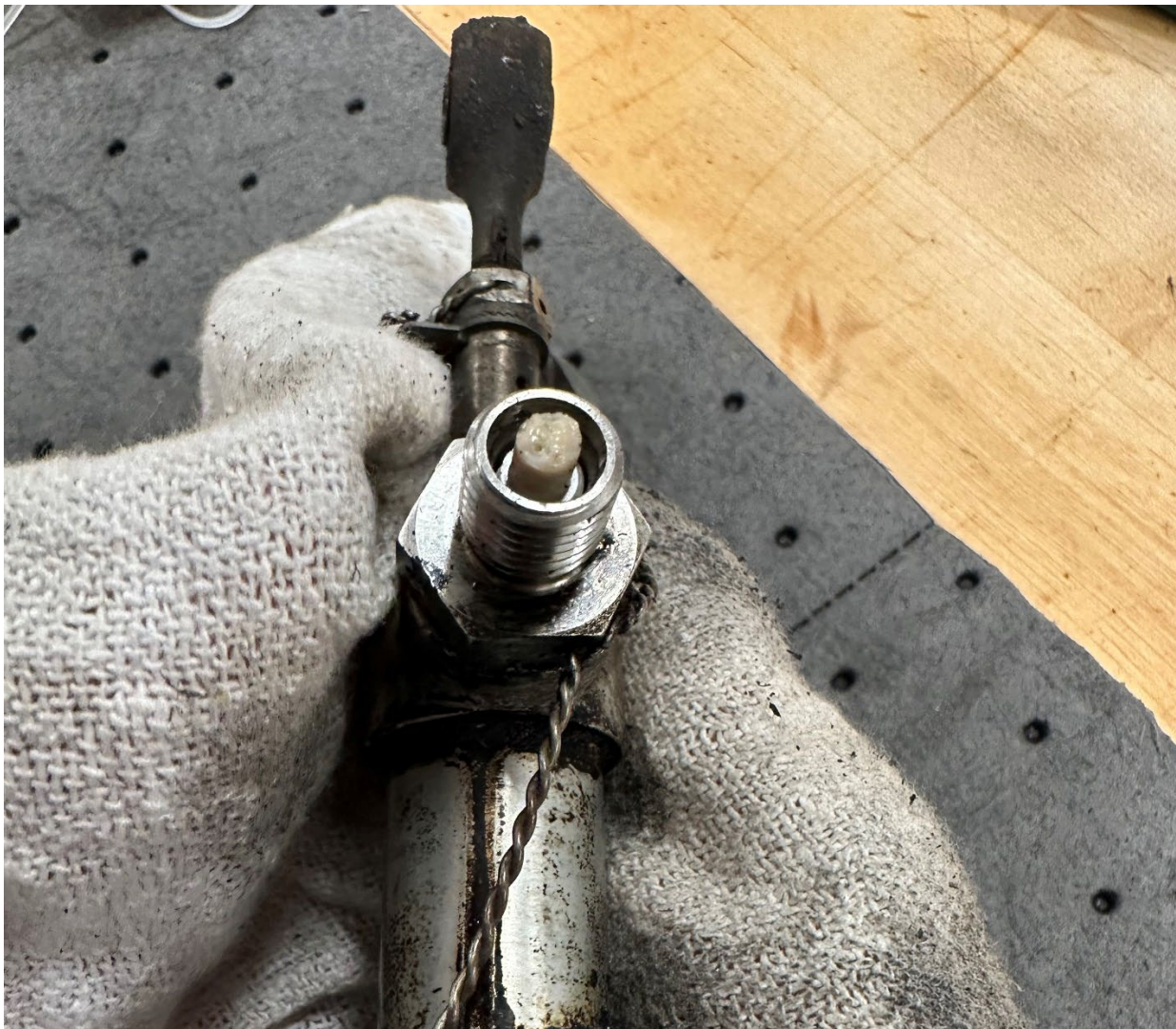
Figure 25: Piston extrusion from the first officer left brake master cylinder inlet port fitting. Picture courtesy of Honda.
