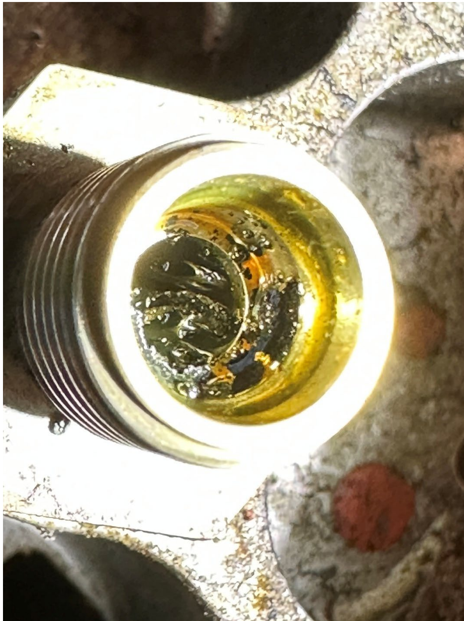
Figure 14: FOD observed in the brake right port fitting of the power brake and antiskid valve. Photo courtesy of Honda.
