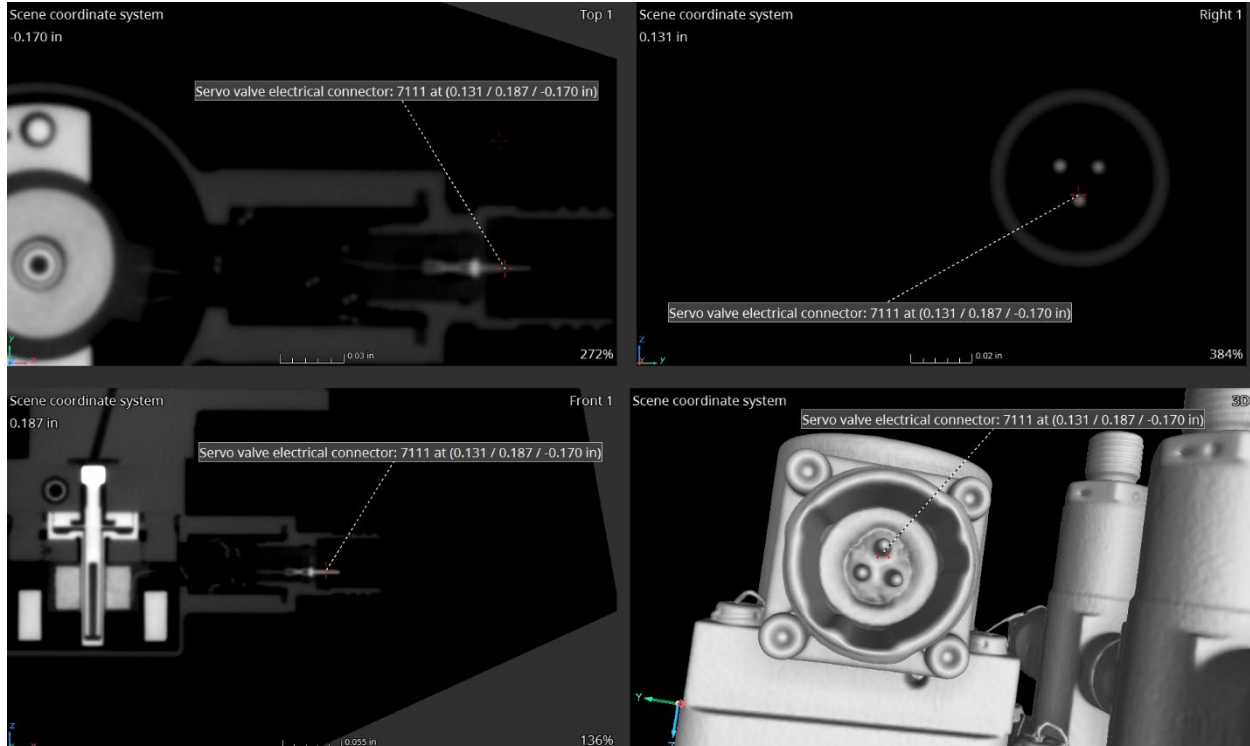
Figure 48. Power brake and antiskid valve assembly – servo valve electrical connector.
