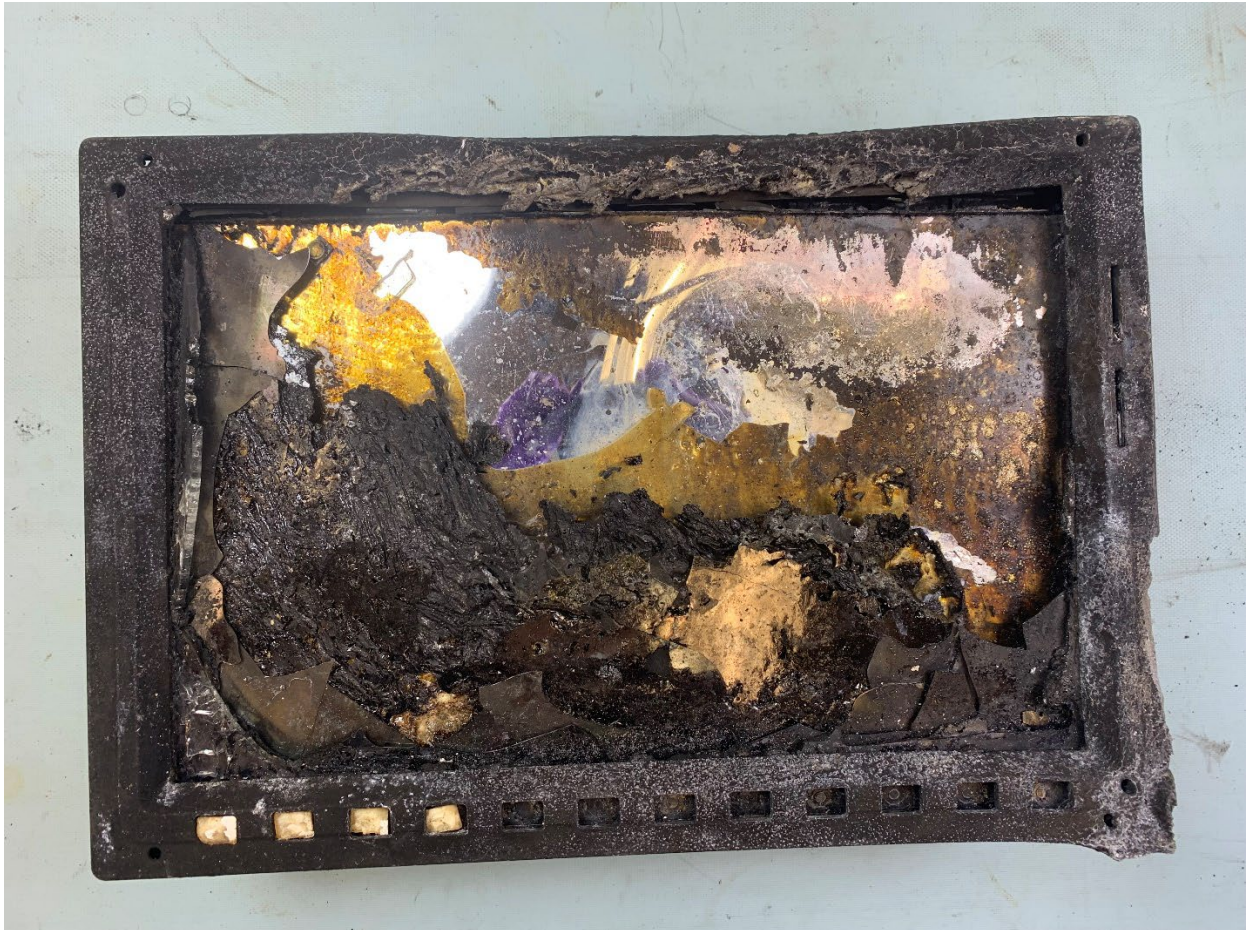
Figure 1. Damaged exterior of GDU MFD display.
