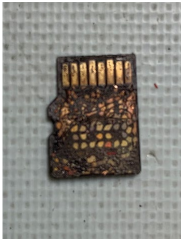
Figure 4. Bottom of microSD card from right PFD display.
