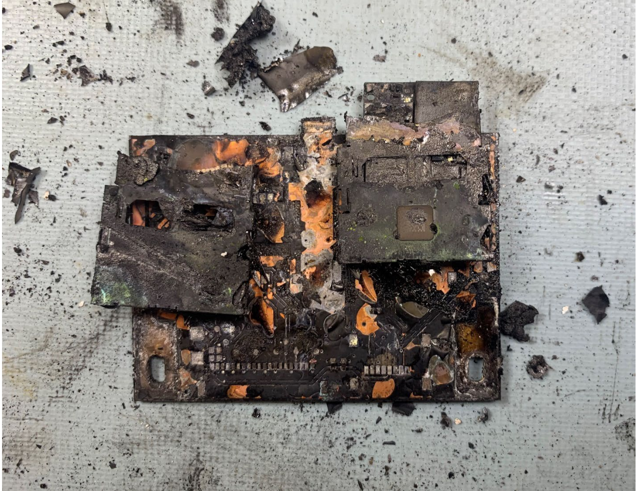
Figure 2. Memory module removed from the GDU MFD display.
