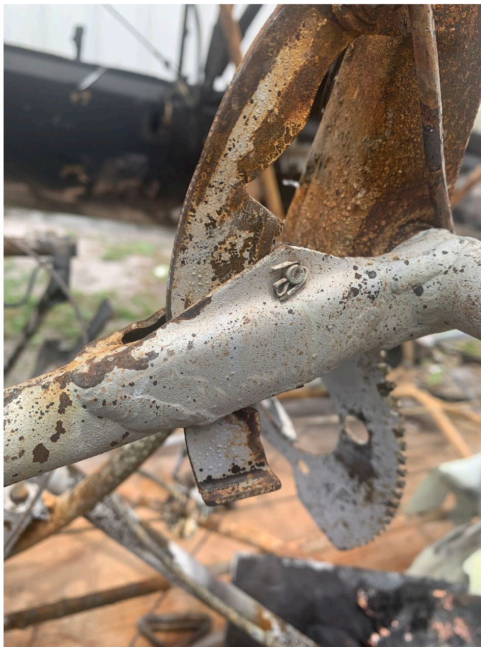
Photo 2 – Flap Handle Secure in First Notch (10 degrees) of Flaps as Found (FAA)
