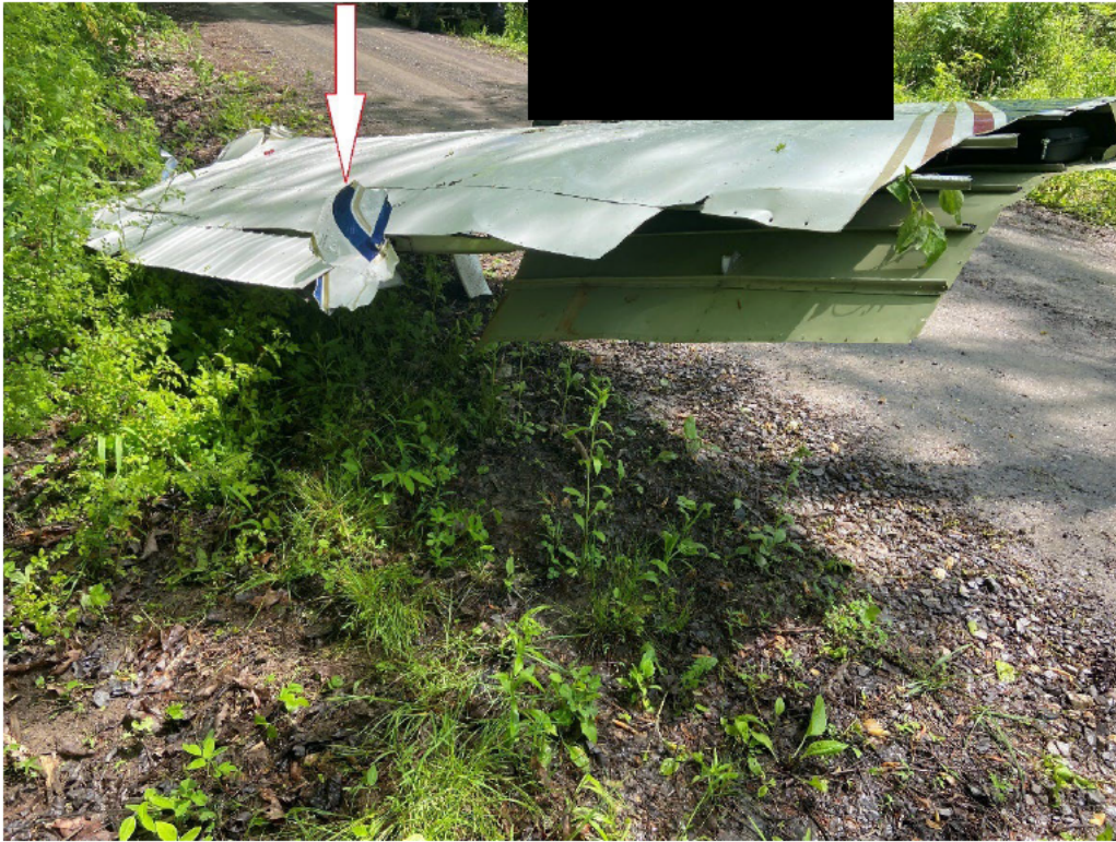
Figure 2: View of the Right Wing On a Logging Road As Observed By FAA Before the Wing was Stolen. Arrow Points to Left Side Fuselage Skin Normally Located Between Fuselage Stations 156.0 and 172.0.
