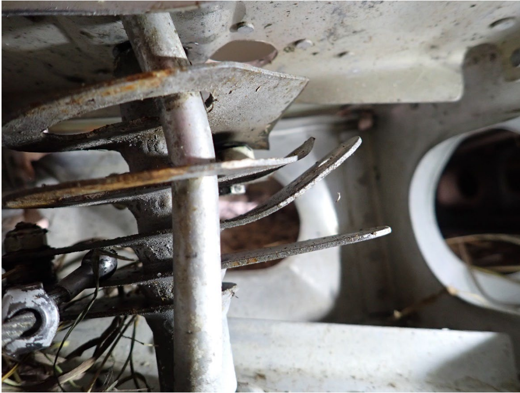
Figure 6: View of Deformed Forward Aileron Bellcrank.
