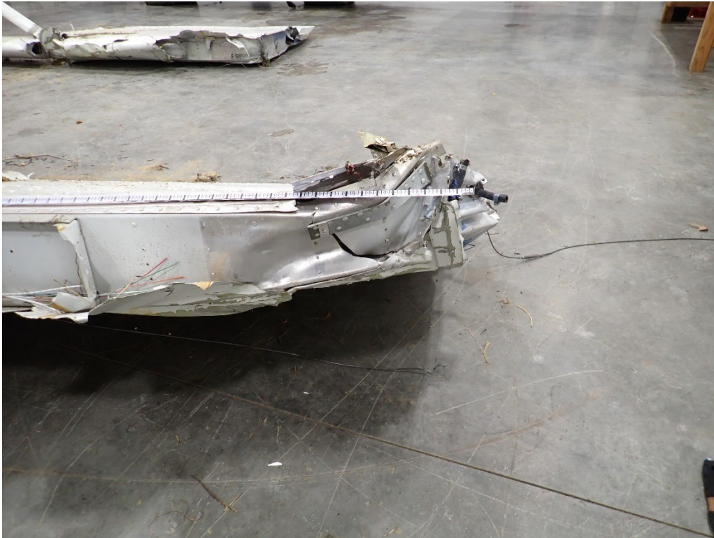
Figure 10: View Showing the Up and Aft Deformation of the Main Spar at The Wing Root.
