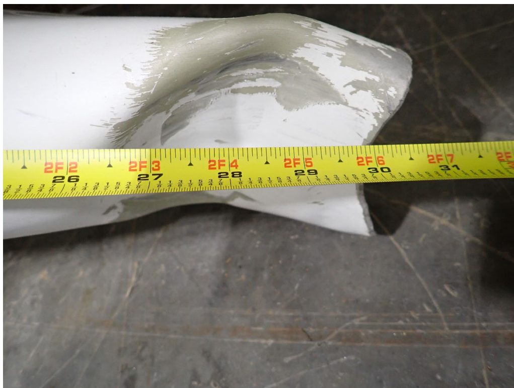
Figure 9: View of the Impact Damage on the Leading Edge of the Left Strut.
