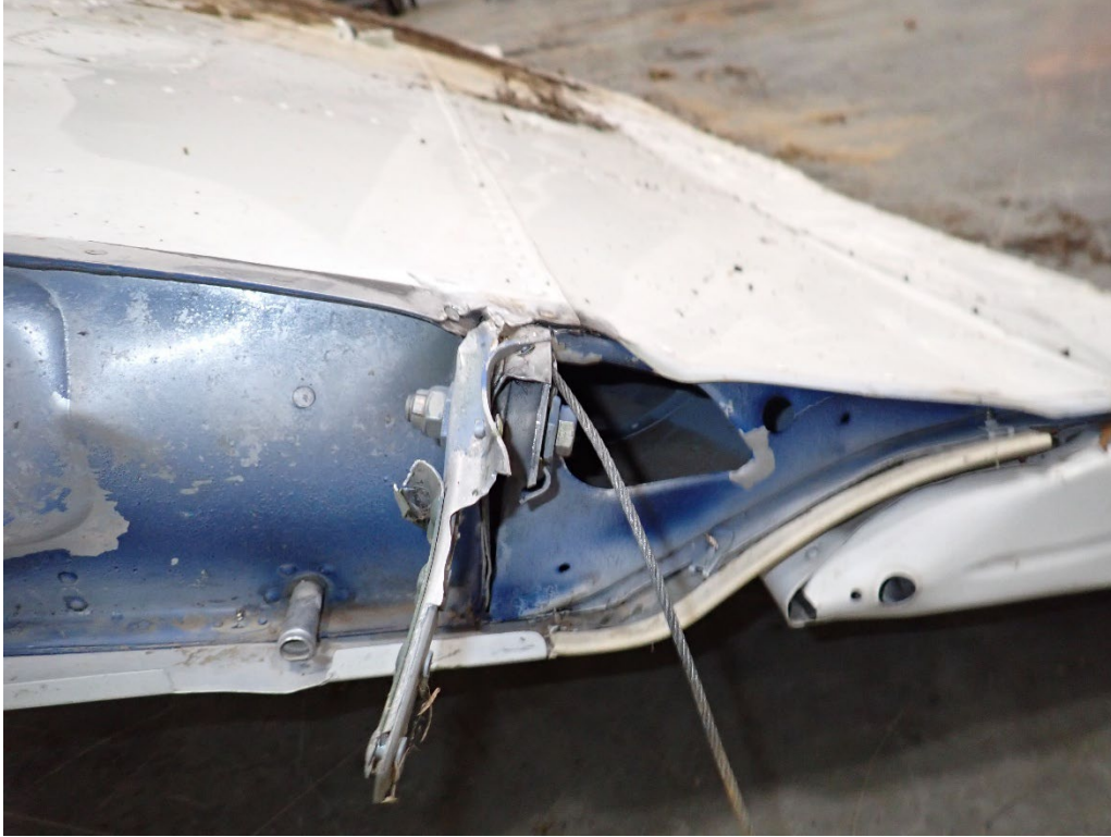
Figure 11 View Showing the Aft Spar of the Right Wing with Attached Fractured Section of Rear Fuselage Spar
