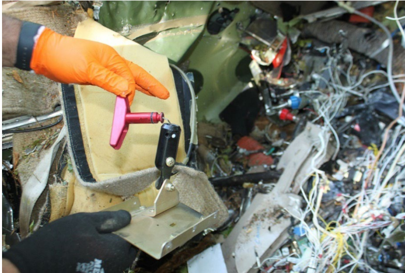
Figure 10 View of the BRS Activation Handle
