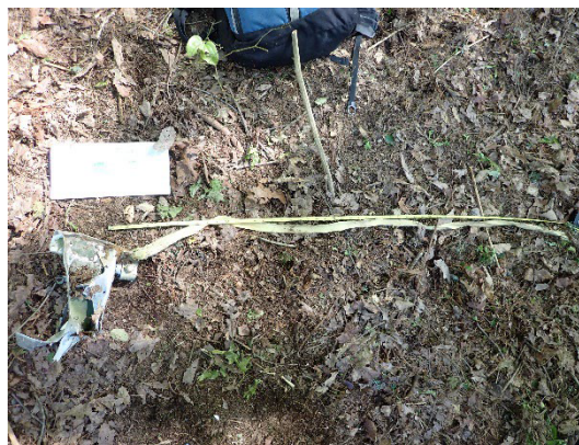
Figure 15 Figure 12 View Depicting Length of Fractured Right Forward Harness
