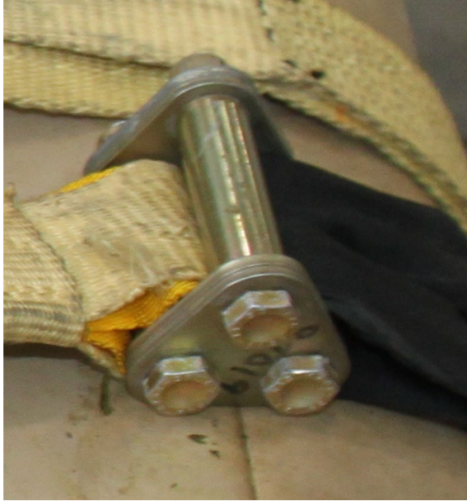
Figure 18 View of the 3 Pt. Shackle The bolt/bushing on top is Where the Parachute Riser Would Attach
