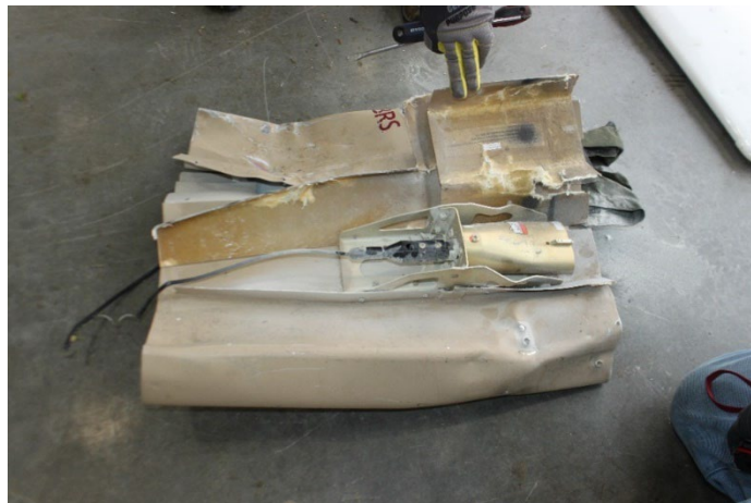
Figure 11 View of the BRS-182 Canister and the remaining parts of the activated rocket
