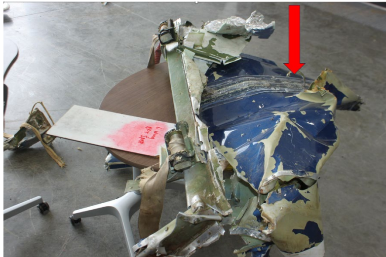
Figure 12 Upper Skin Aft of Aft Spar Arrow Points to Area of Separated Fiberglass Cover For Front Harness
