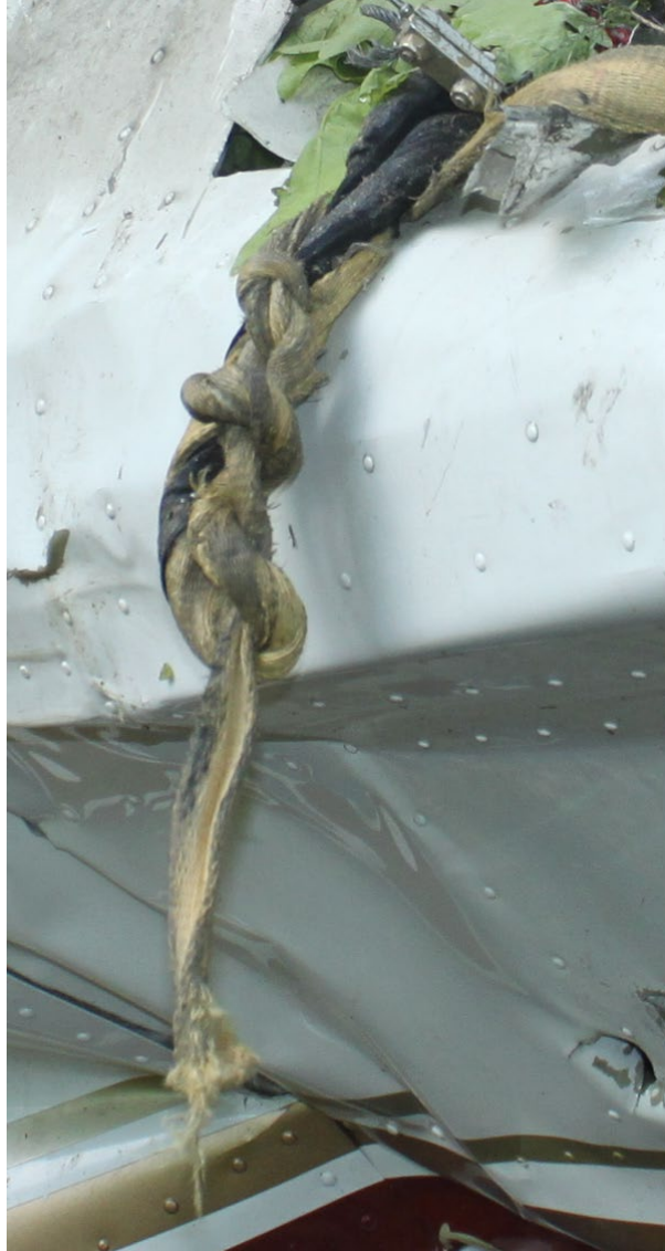
Figure 19 View of the Entanglement of the Front Harness and Fractured Right Forward Harness
