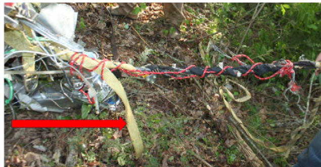
Figure 21 View of the Tangled Front and Rear Harnesses. Arrow Points to Still Sewn Together Portion of Rear Harness
