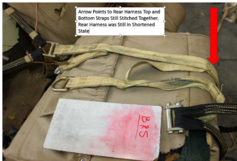
Figure 20 View of Harnesses and 3-Pt. Shackle of BRS System Arrow Points to Section of Rear Harness Still Sewed Together
