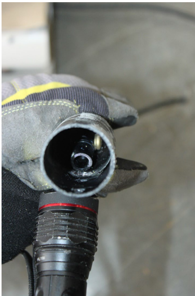
Figure 22 View of the Rocket Cone and Fire Pin Actuator Inside Rocket Cone
