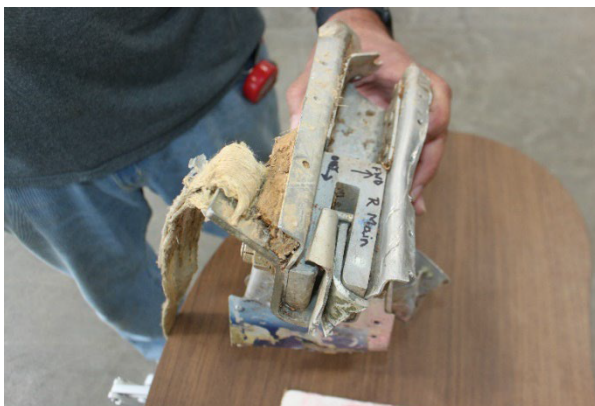
Figure 14 Figure 10 Right Main Spar With Attached BRS Harness
