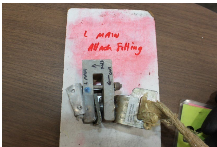
Figure 13 View of the Left Main Spar With Attached BRS Harness
