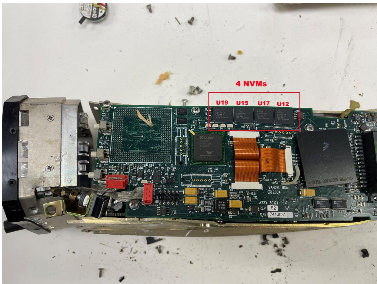
Figure 4. Sandel SN3500 internal circuit board.
