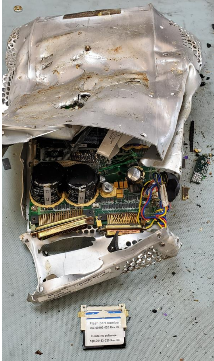
Figure 2. CF card recovered from the Avidyne EX500.
