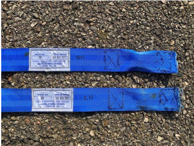
Figure 27. Cessna 172 Skyhawk, N734GB, front seat upper torso harnesses failed stitching.
