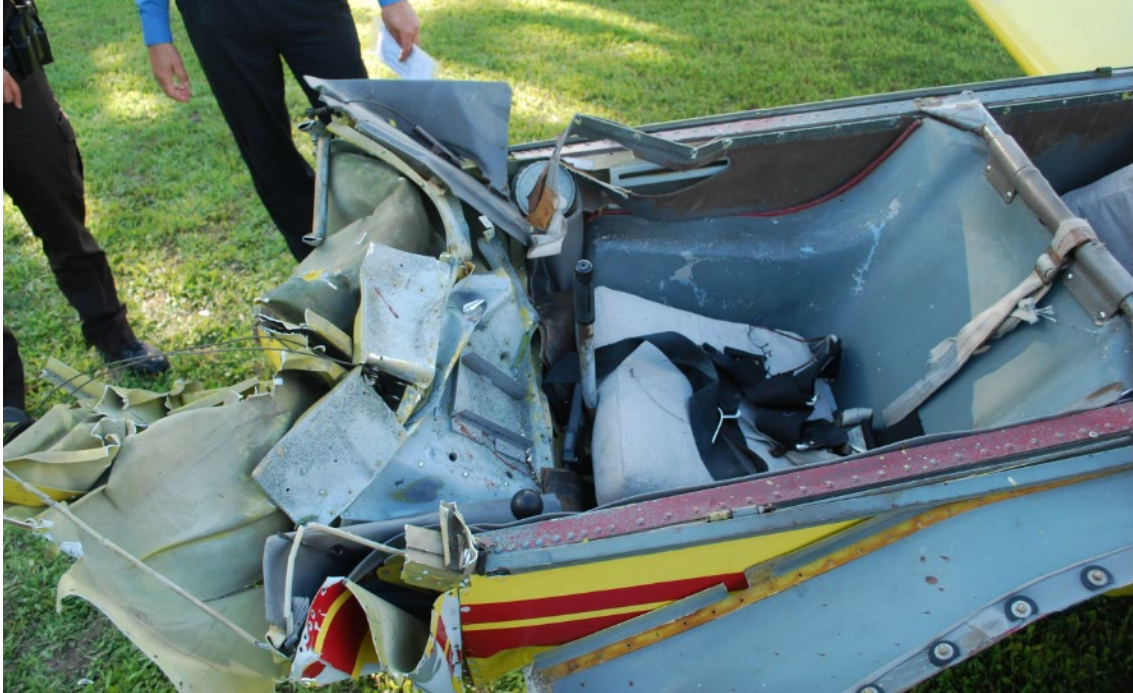
Figure 12. Schweitzer N591CC front seat upper torso harness and attachment point.
