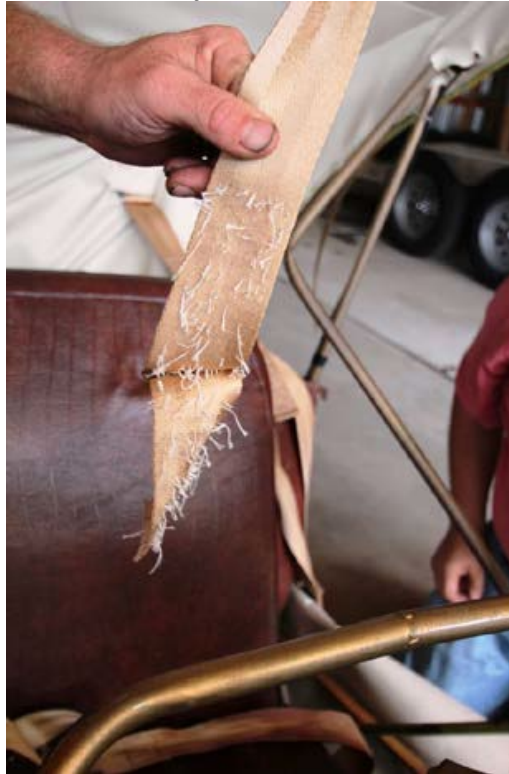
Figure 14. Aeronca N82383 pilot's upper torso harness as found in airplane.
