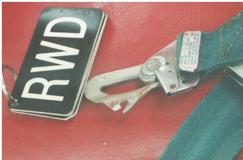
Figure 3. Photograph of rear seat belt attachment hardware failure.
