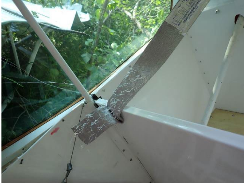
Figure 29. Photograph of the upper torso restraint failure.
