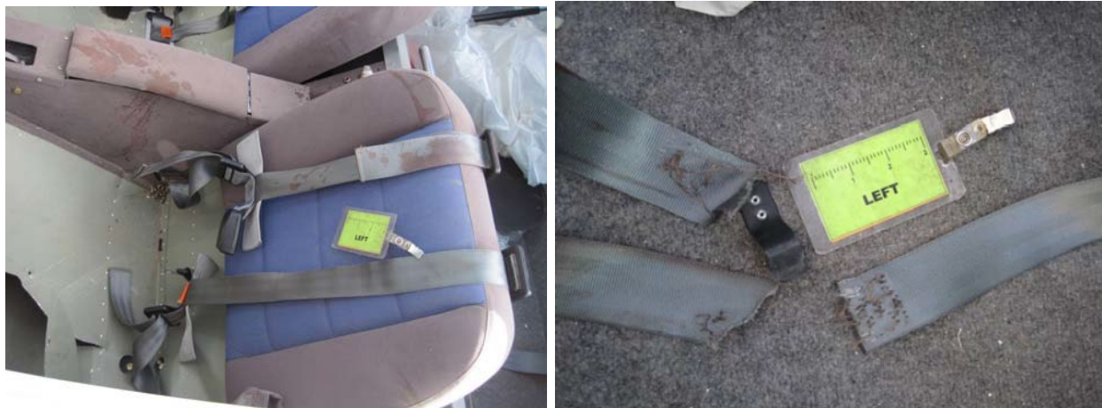
Figure 10. Left seat place with restraints, (right) view of separation point for the restraints.
