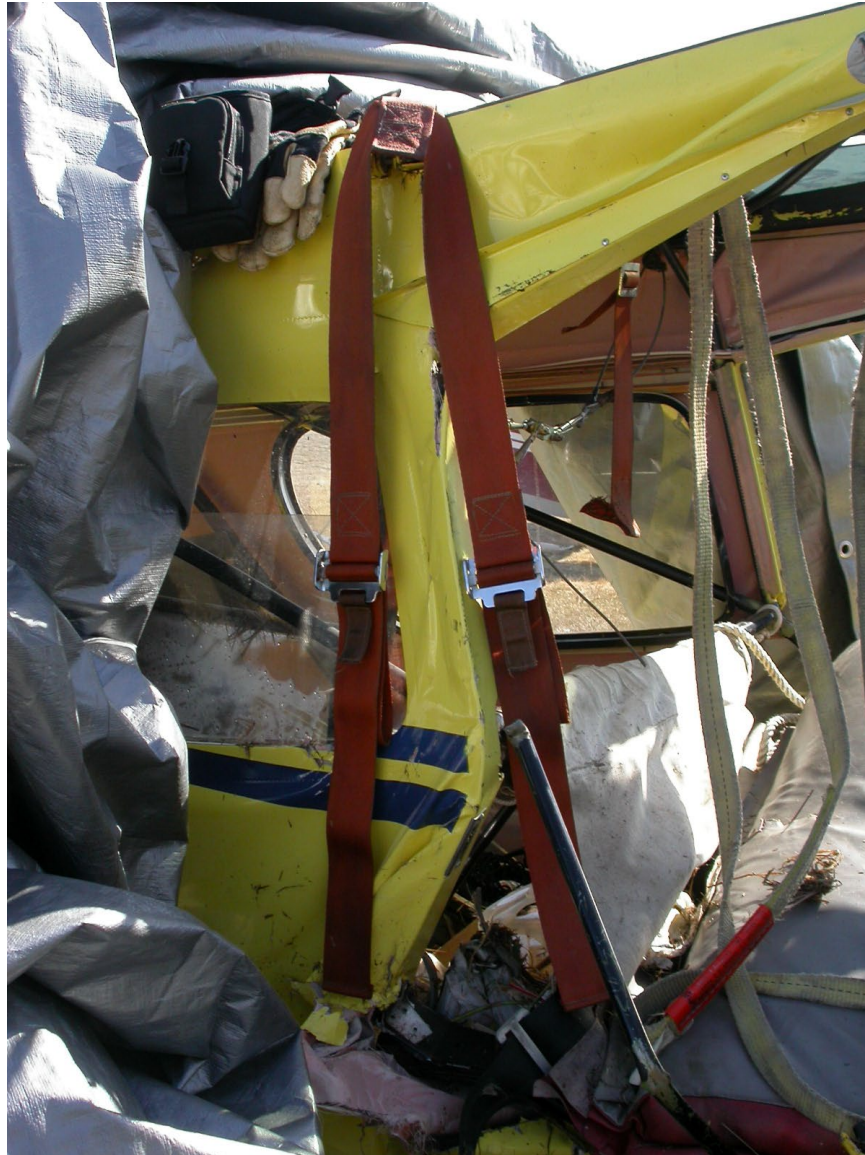
Figure 5. Picture showing intact right side passenger harness, and left side pilot failed upper torso harness.
