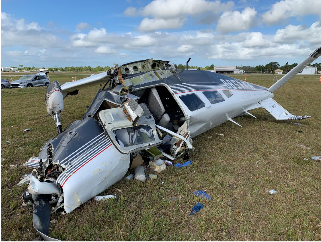
Figure 2 View of entire airplane wreckage looking aft.
