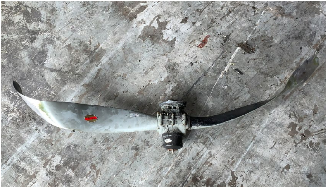
Figure 5 Hartzell propeller exhibiting signs of bending and polishing.
