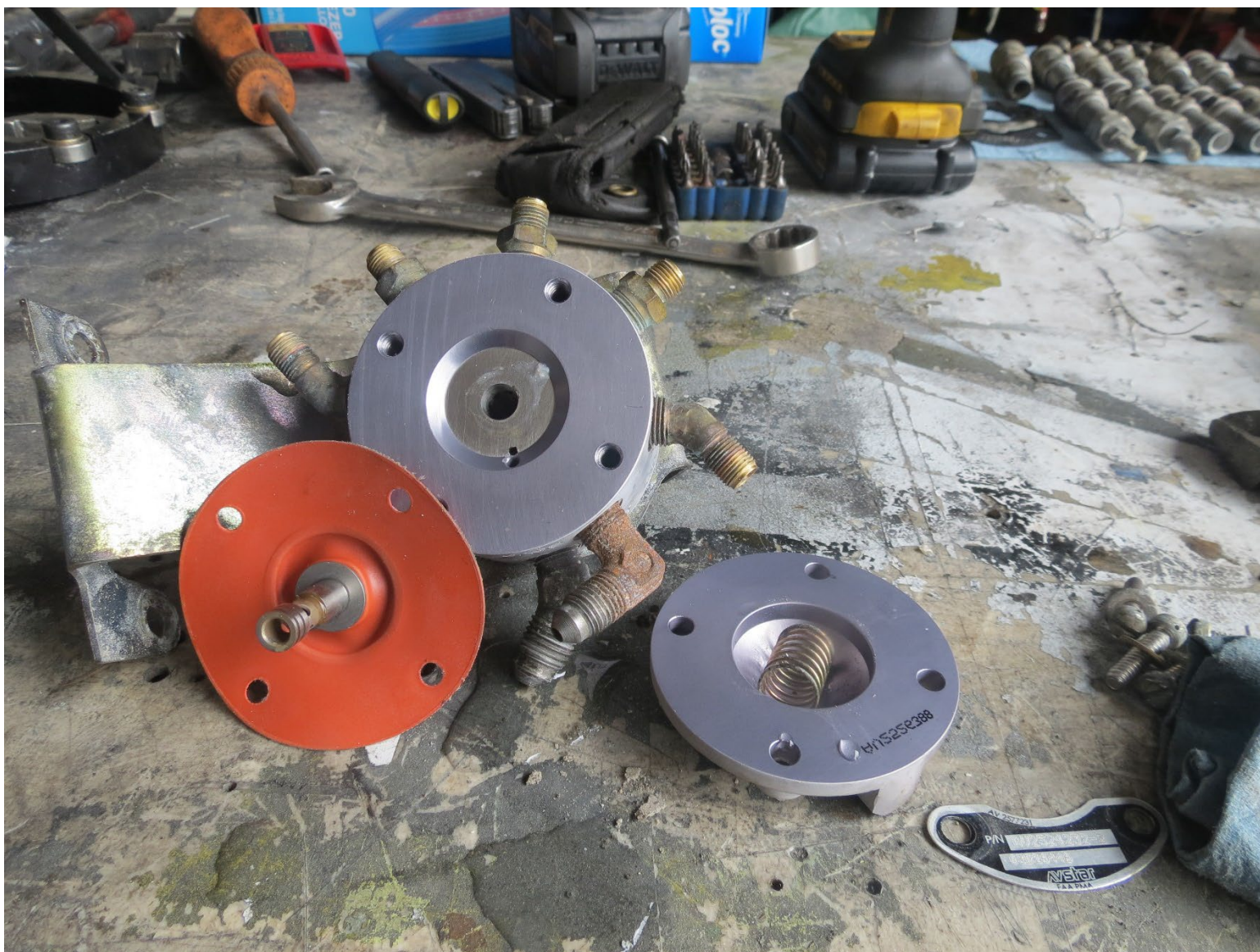
Photograph 26 - Interior of Fuel Distribution Manifold (Courtesy of Lycoming Engines)
