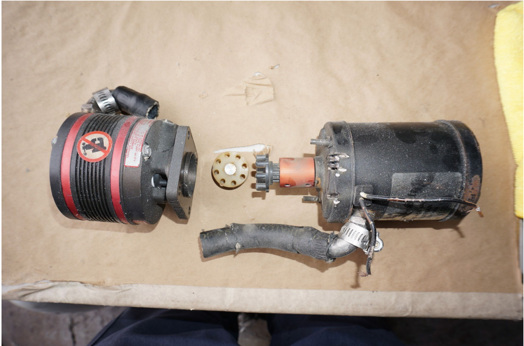
Photograph 10 - Standby (Electric) Vacuum Pump
