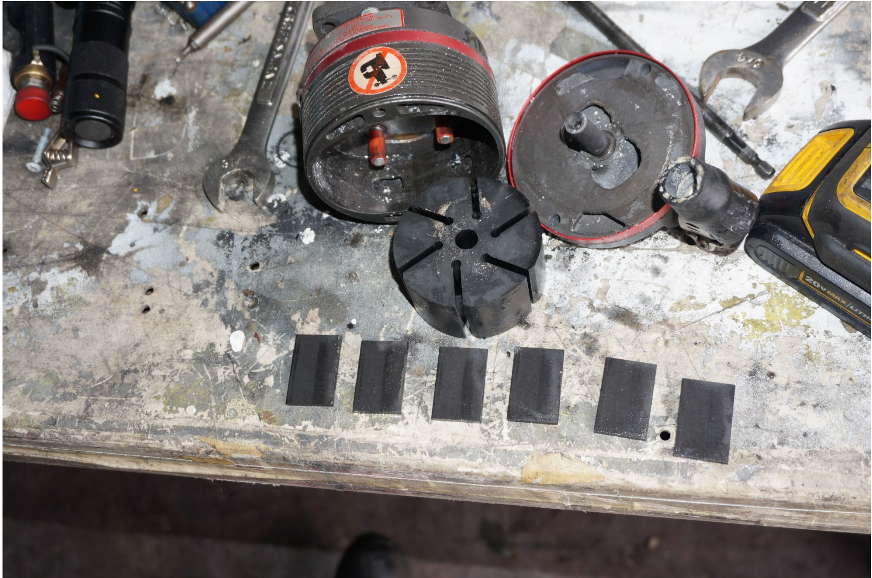
Photograph 11 - Interior of Standby (Electric) Vacuum Pump
