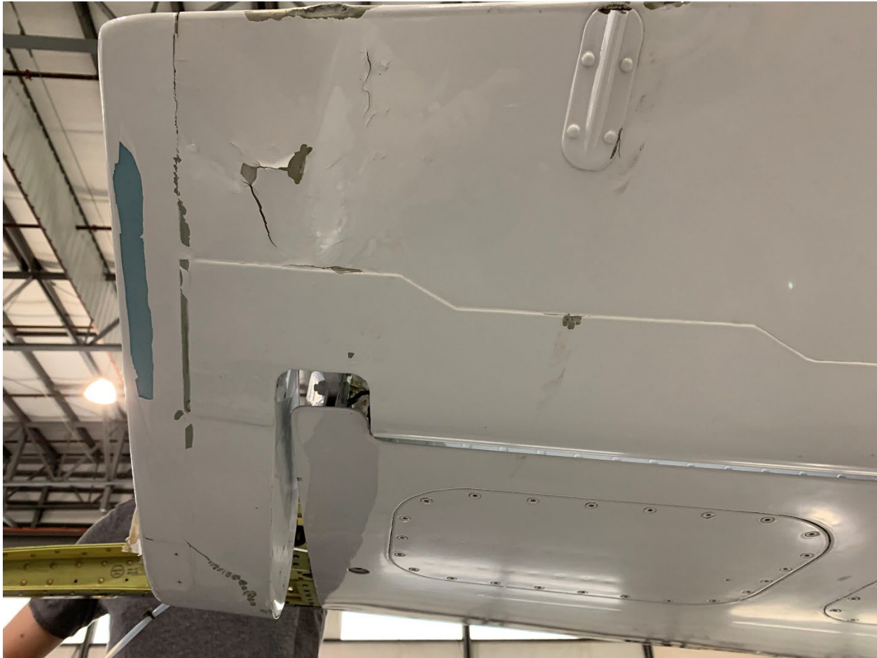
Figure 8. Damage to the bottom side of the aileron and wing
