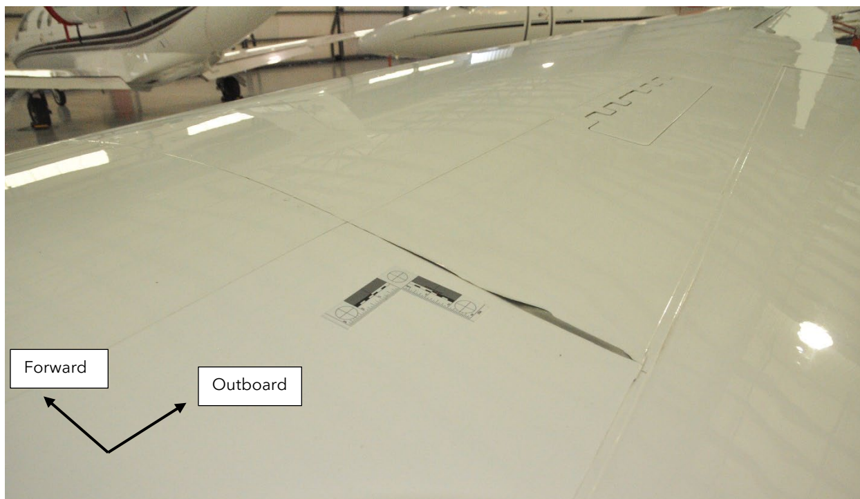
Figure 12. Chipped/peeling paint found on top side of right wing (courtesy of Tamarack).
