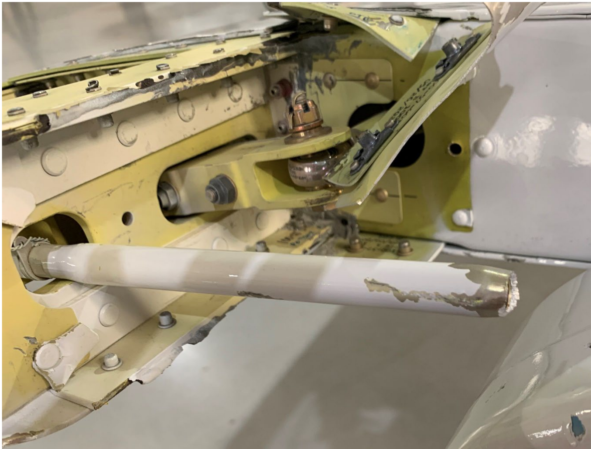
Figure 10. Picture of the "long push rod" with missing rod end and scraped paint.
