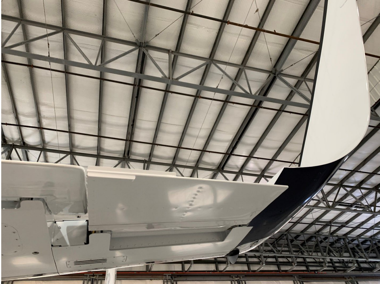
Figure 11. Right wing with intact wing extension, winglet, and TACS. TACS is near the full down position.
