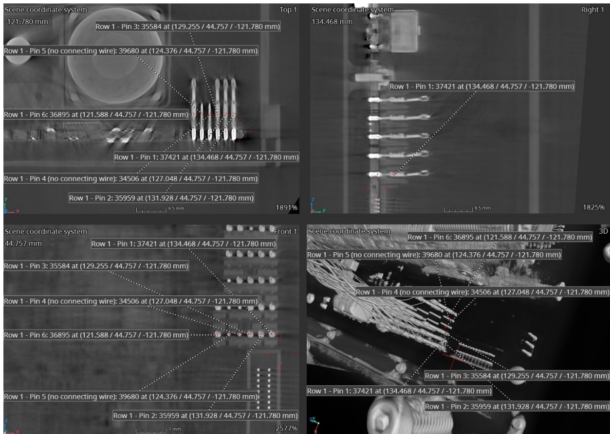
Figure 19. Left TACS control unit – printed circuit board (PCB) connections row 1.
