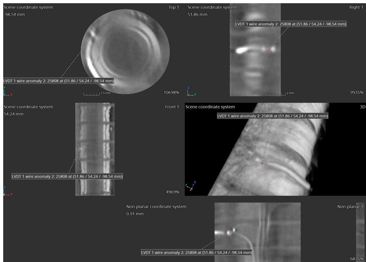
Figure 37. Left TACS control unit - LVDT 1 wire anomaly 2.
