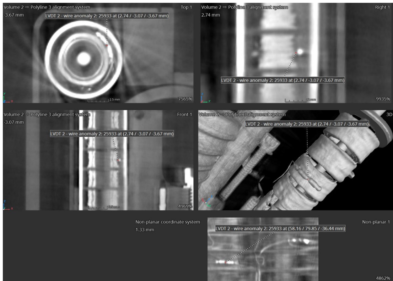
Figure 43. Left TACS control unit - LVDT 2 wire anomaly 2.
