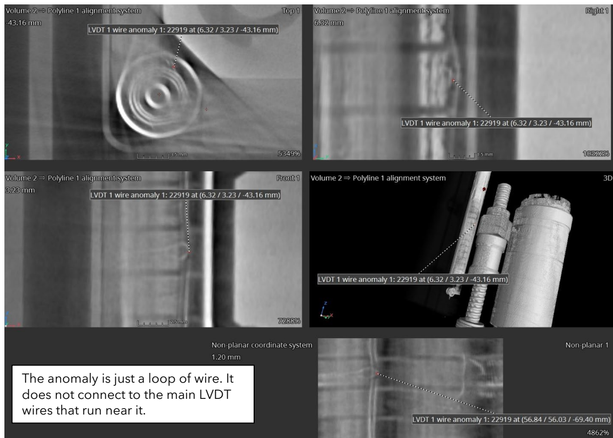
Figure 36. Left TACS control unit – LVDT 1 – wire anomaly 1.
