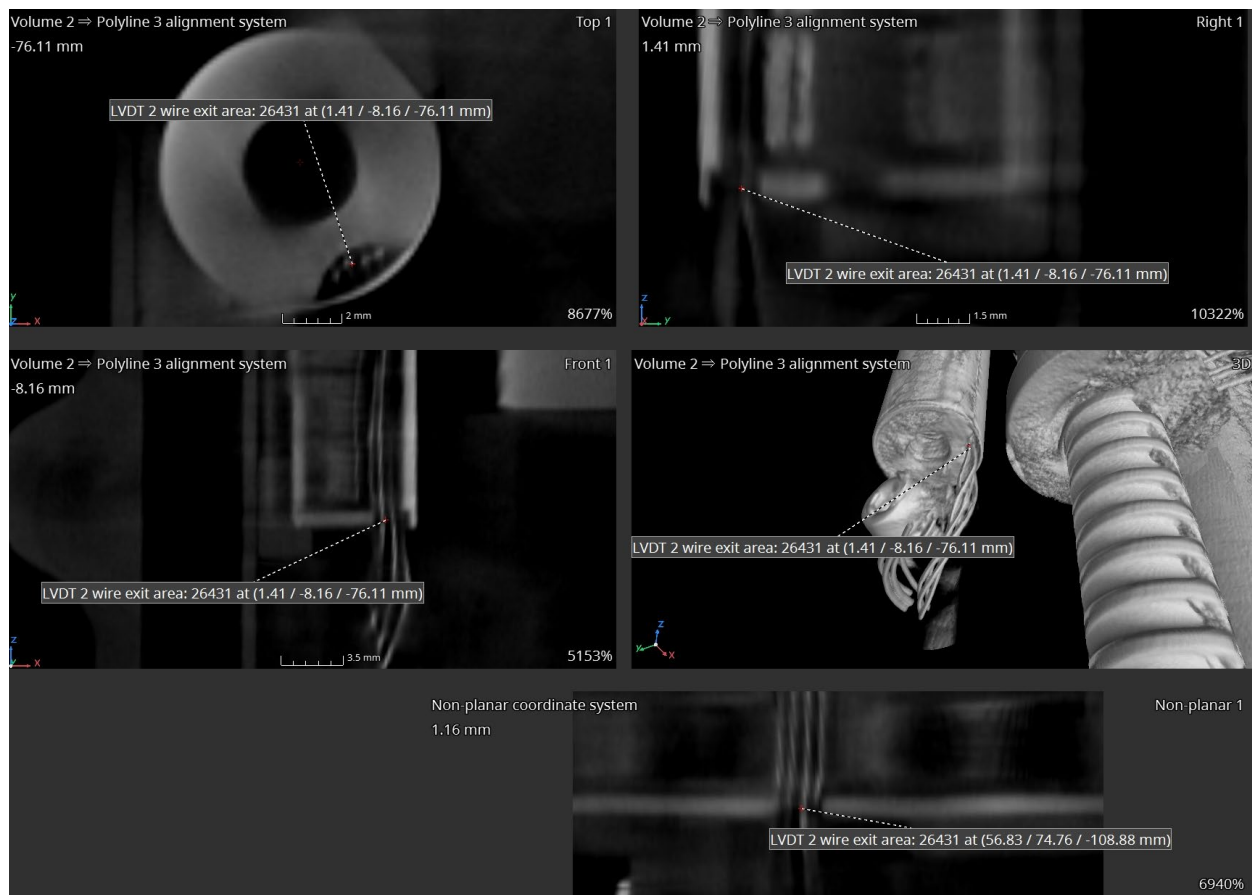
Figure 44. Left TACS control unit – LVDT 2 wire exit area.
