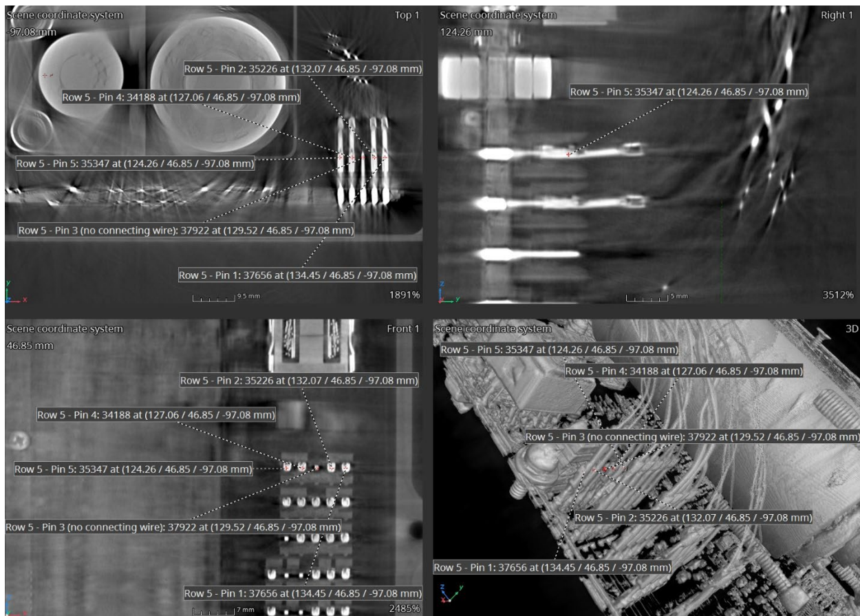
Figure 23. Left TACS control unit – PCB connections row 5.
