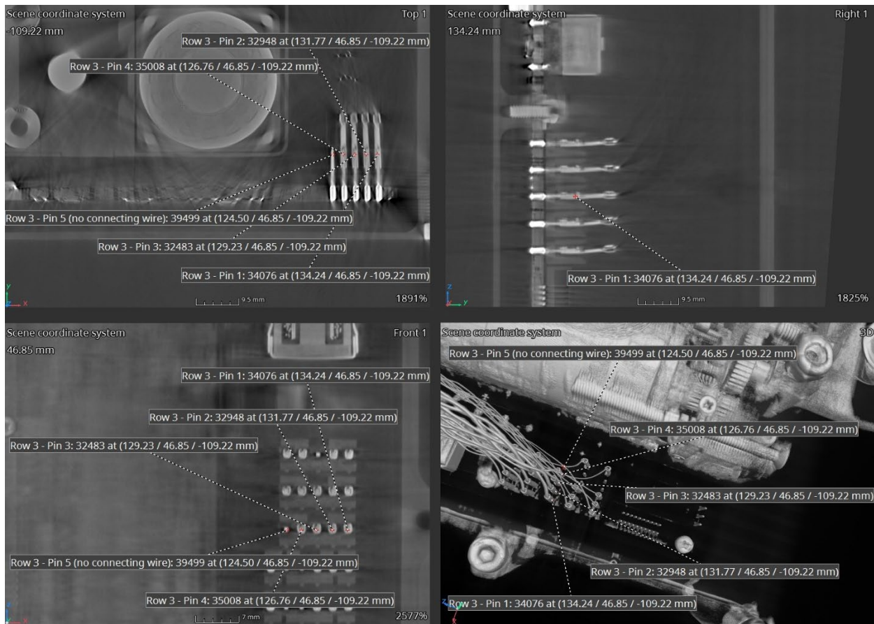
Figure 21. Left TACS control unit – PCB connections row 3.
