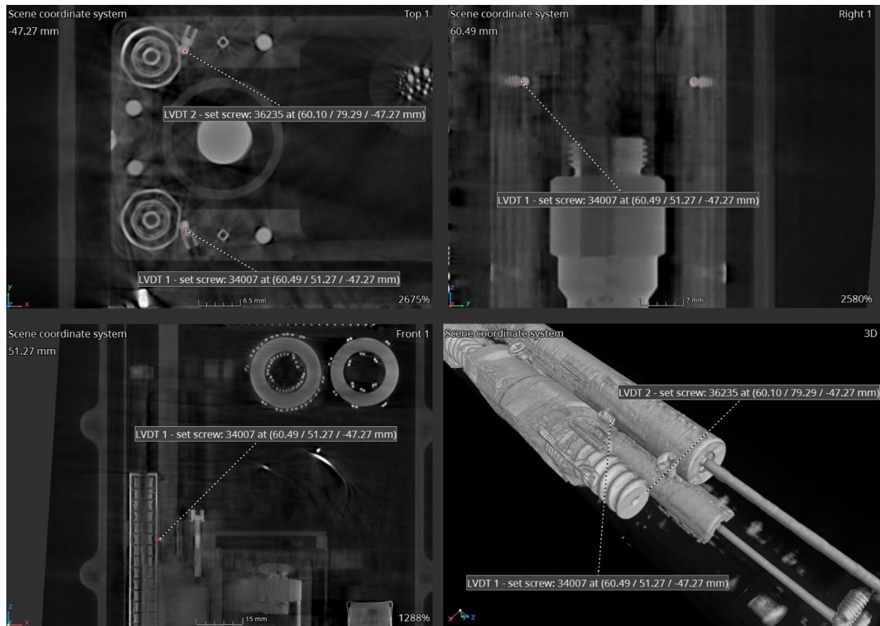
Figure 30. Left TACS control unit - LVDT 1 set screw.
