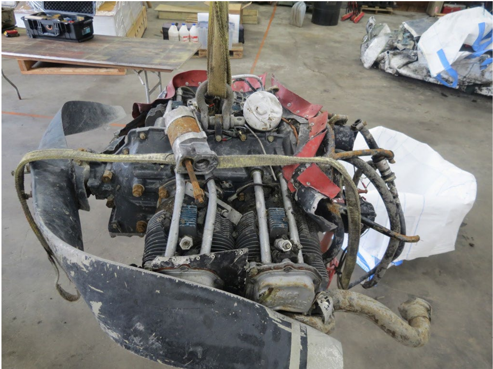
Photo 3 – Overall View of Engine (Lycoming)
