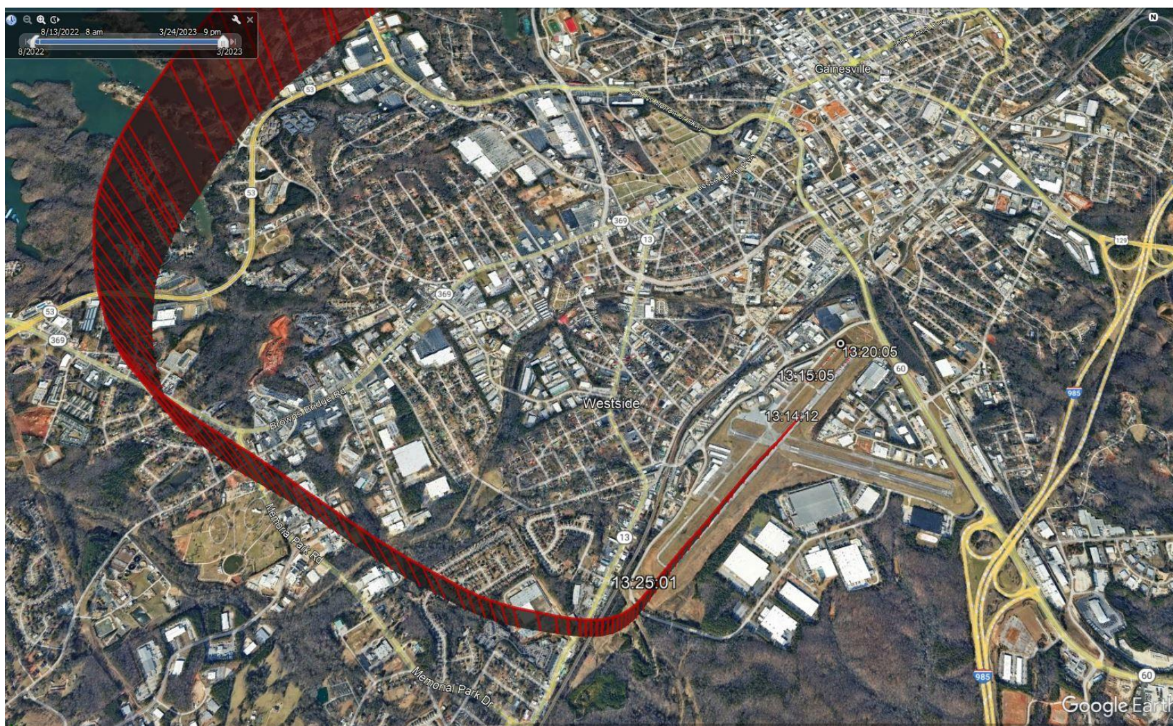
Figure 9. GPS tracklog data associated with the departure portion of the accident flight.
