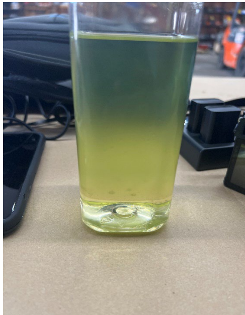
Image of water settled in the bottom of the container
