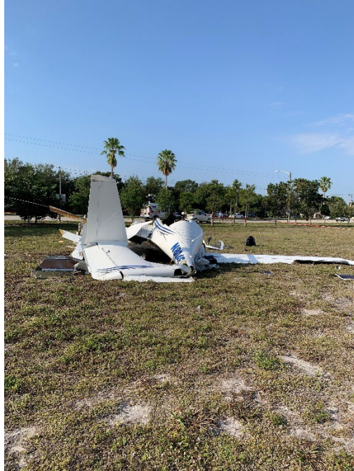
Figure 5: View Showing the Aft Empennage Displaced to the Left.
