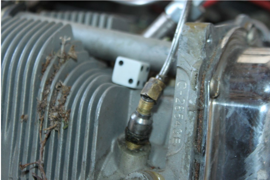
Figure 12: View Showing the Separated Fuel Injector Line From the No. 2 Fuel Injector Nozzle.
