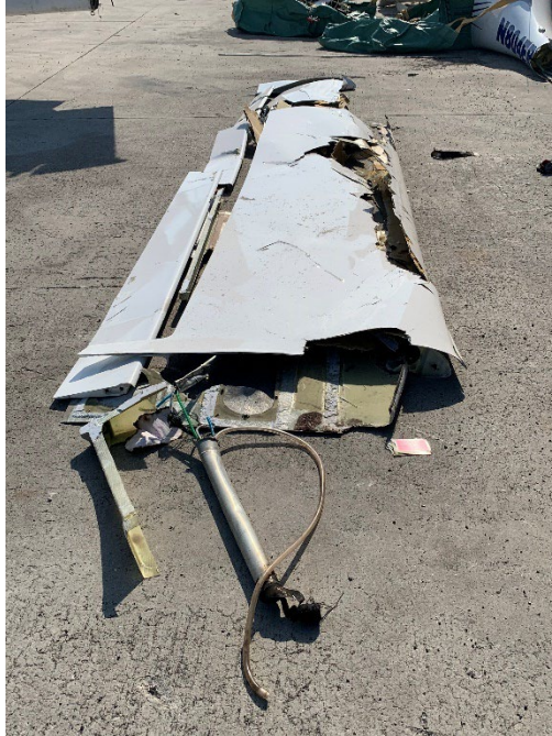
Figure 6: View of the Reconstructed Left Wing.
