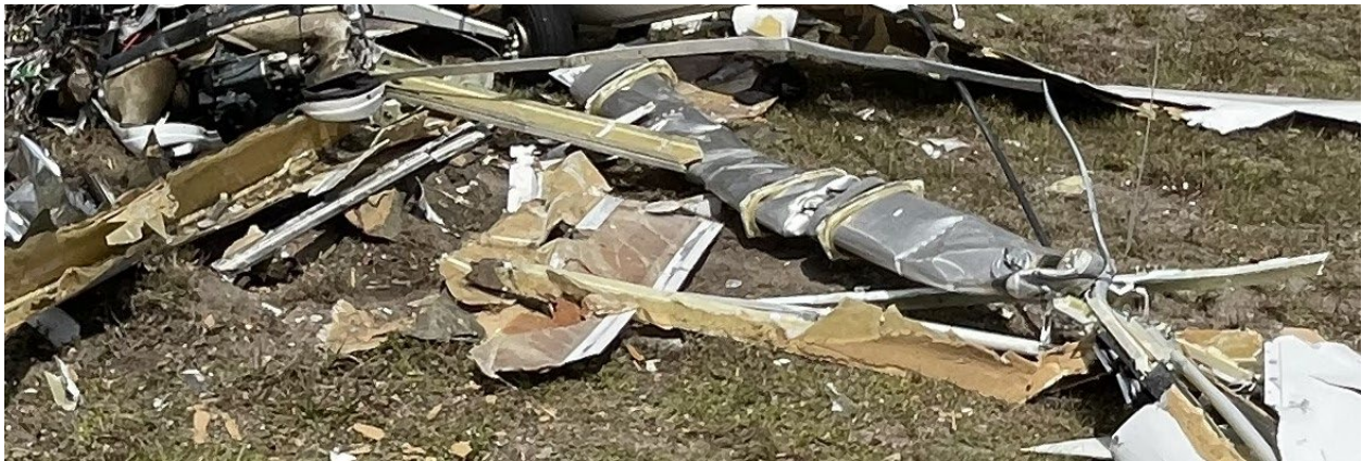
Figure 10: Impact Damaged Left Fuel Tank.
