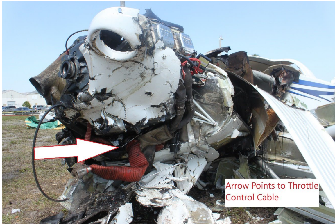
Figure 11: View Showing Separated Throttle Control Cable.
