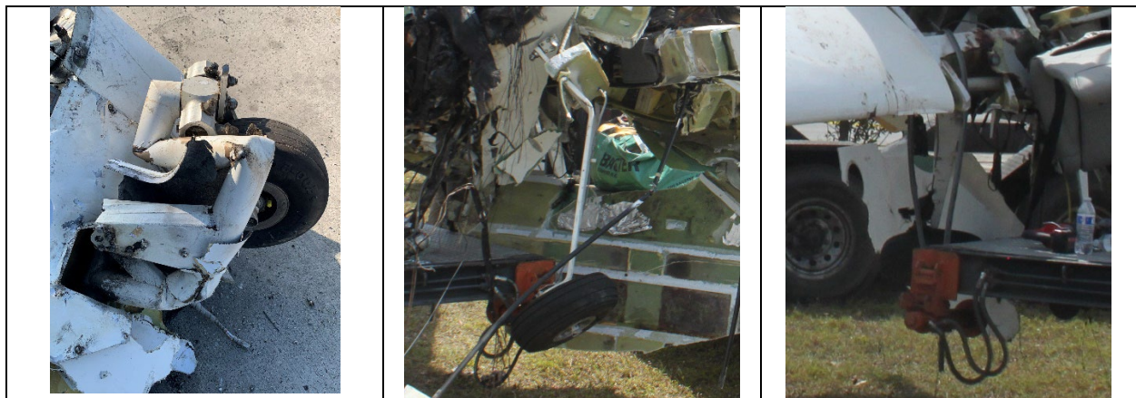
Figure 8: Views of the Landing Gears.
