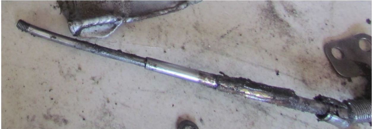
Figure 13: Bent and Fractured Throttle Control Cable.
