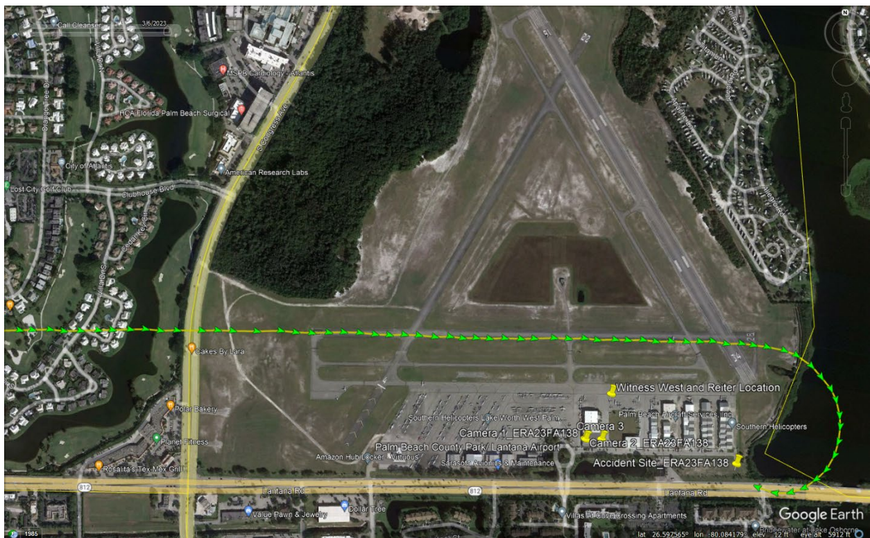
Figure 3: Google Earth Image of ADS-B data of Final Portion of Flight, Witness, Camera, and Accident Site Locations Depicted.
