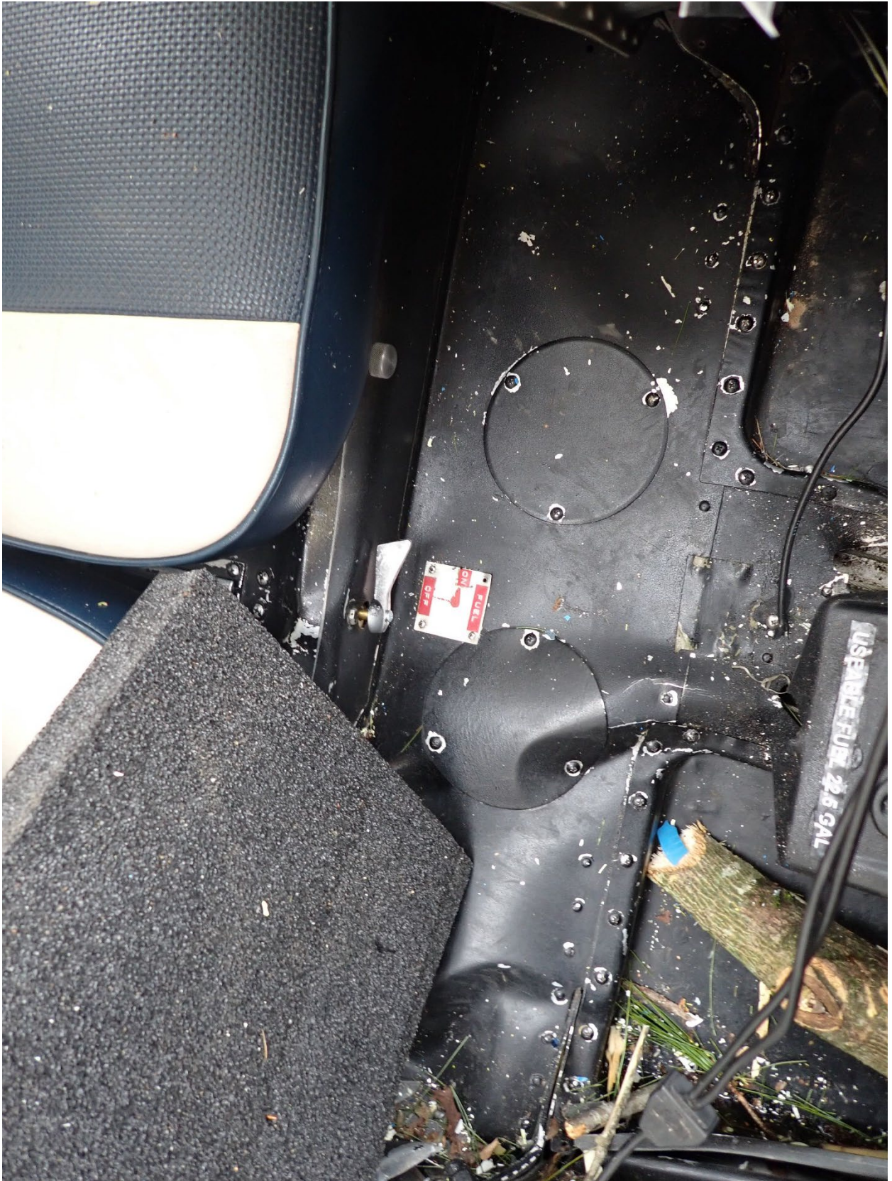
Figure 17: Fuel selector in the on position
