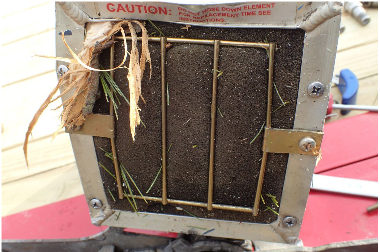
Figure 28: Air inlet filter with tree debris (Textron Photo)
