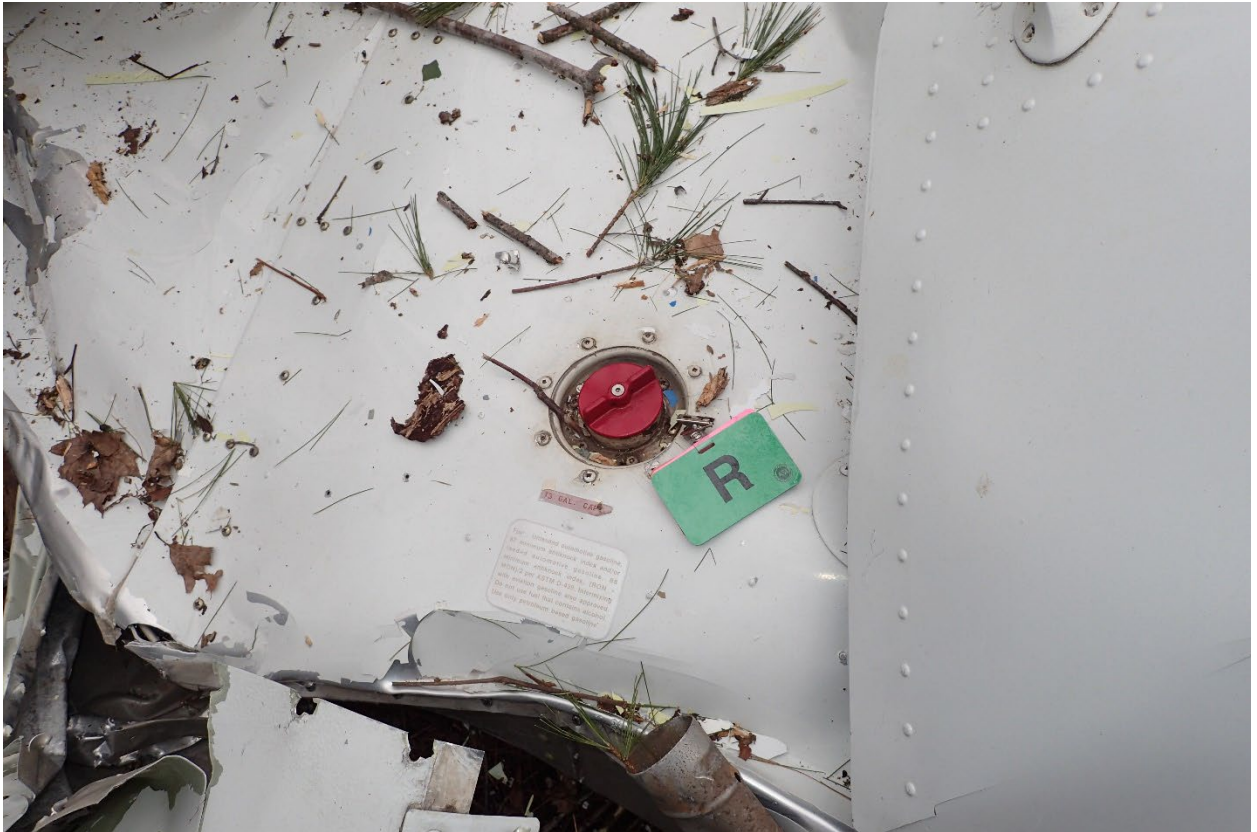
Figure 16: Right fuel cap secured (Textron Photo)
