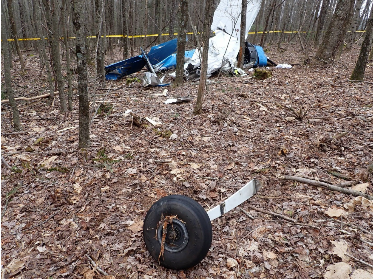
Figure 11: Right main landing gear impact separated
