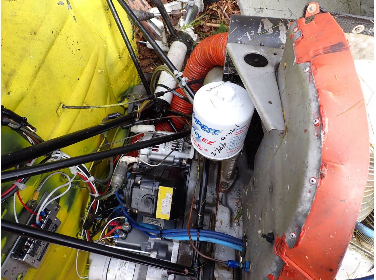
Figure 29: Oil filter attached to engine
