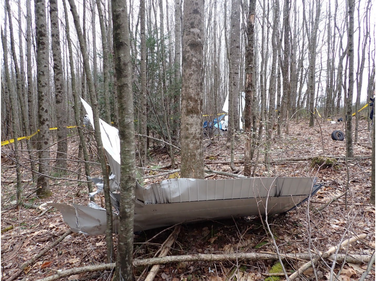
Figure 6: Impact separated section of the left wing
