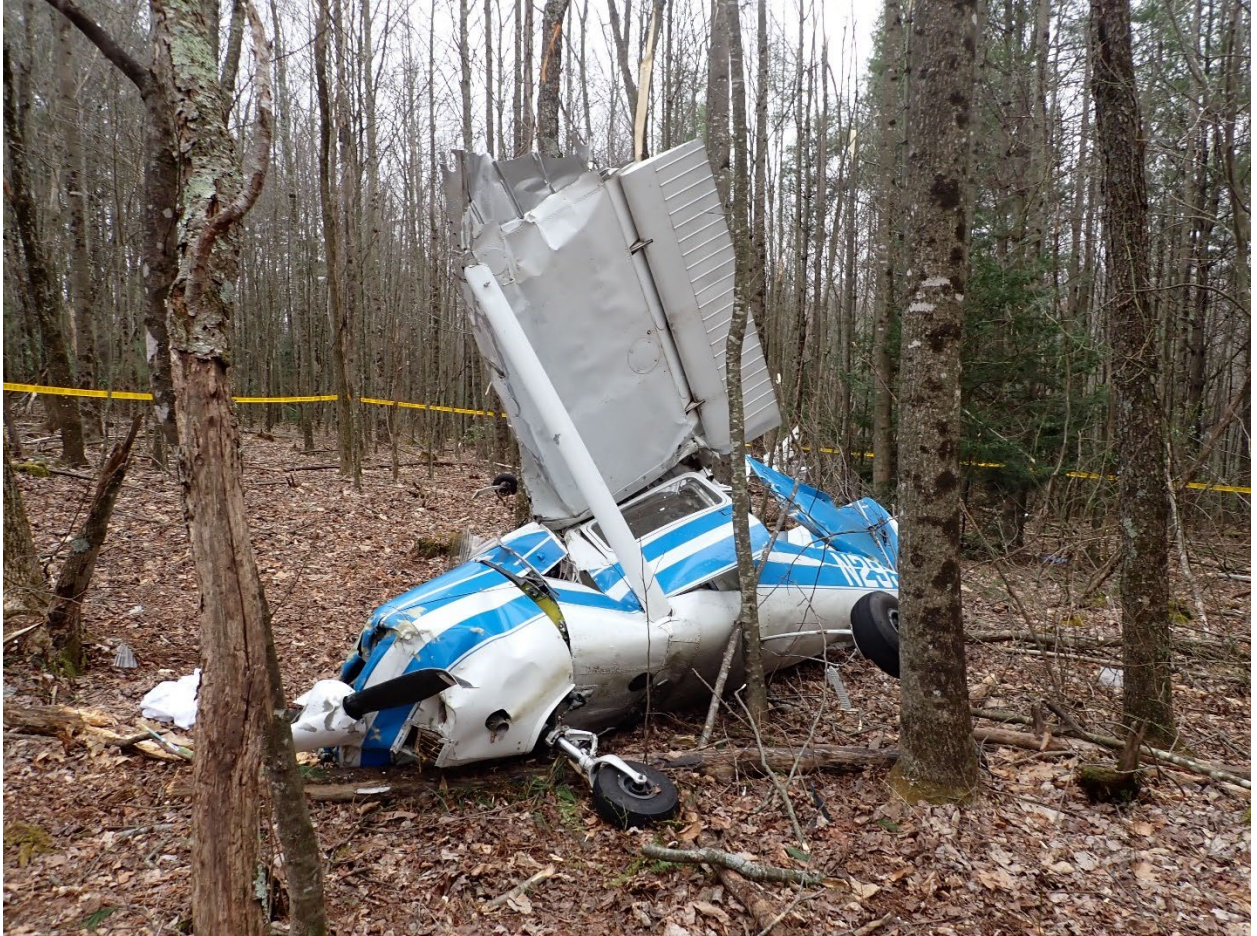
Figure 12: Left main landing gear and nose landing gear
