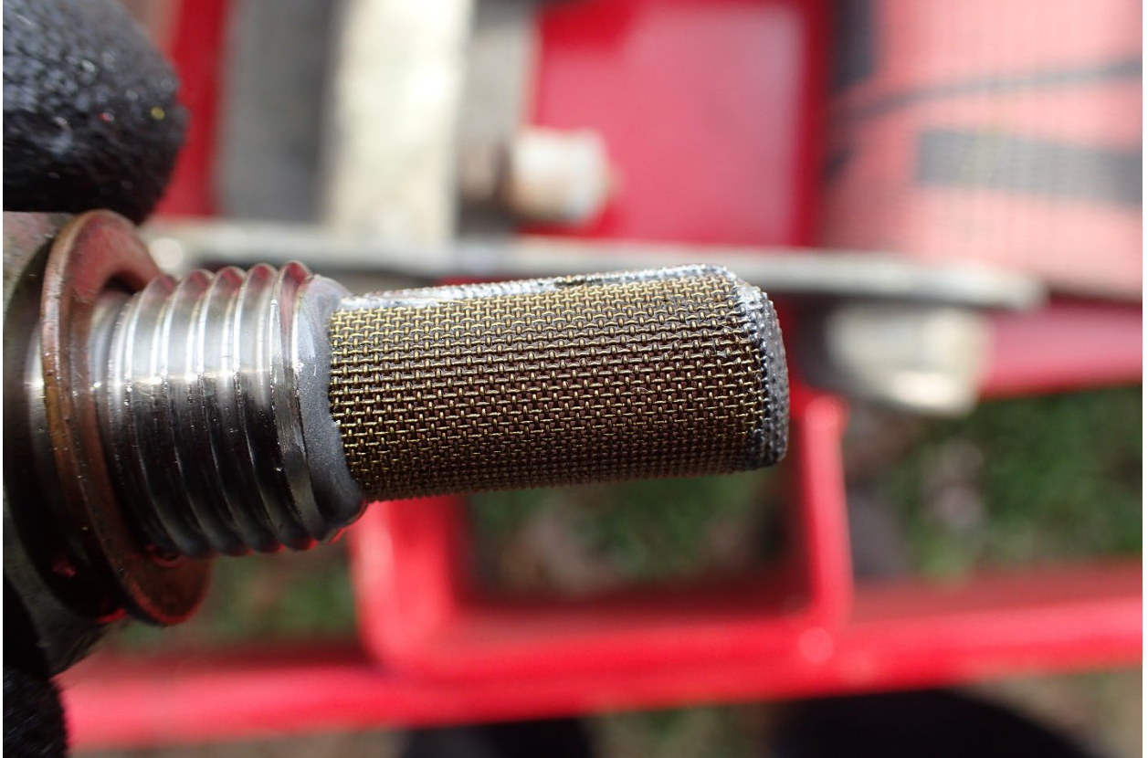
Figure 27: Fuel inlet screen (Textron Photo)
