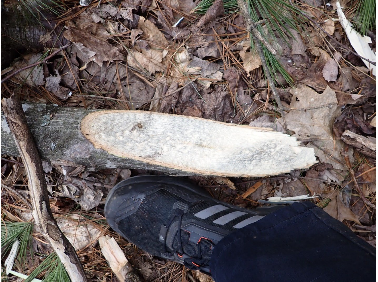
Figure 33: Wood with 45 degree cut and black/grey paint transfer
