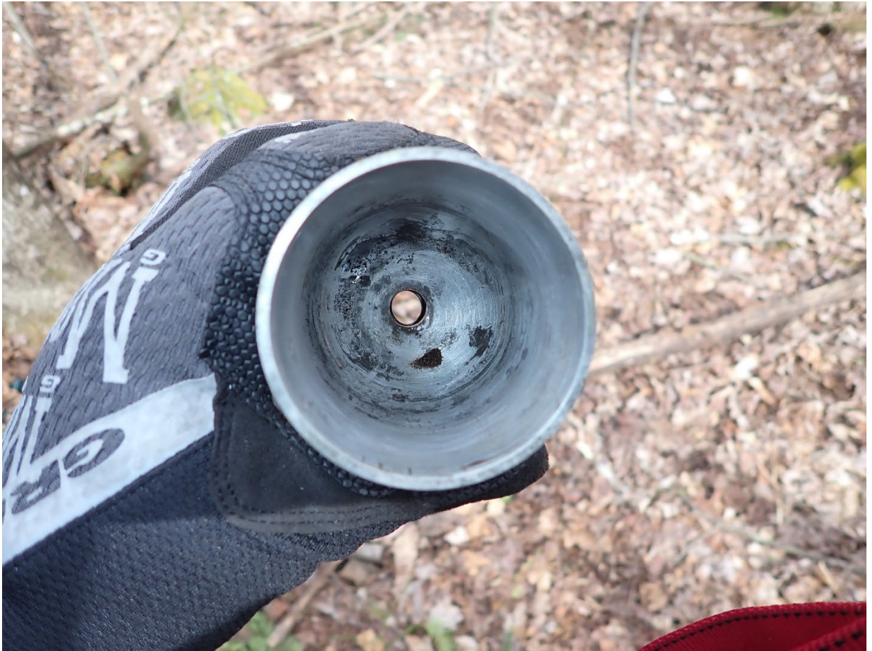
Figure 18: Debris in bowl of fuel strainer
