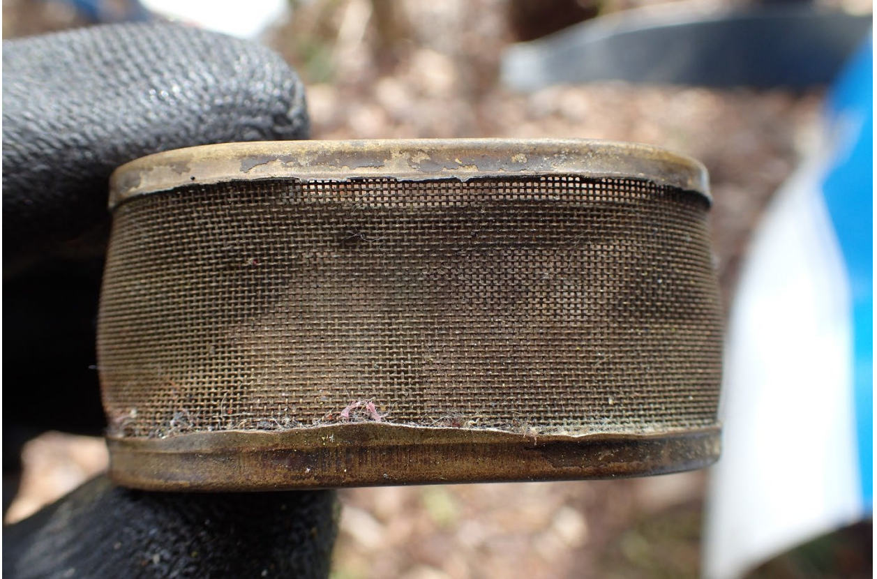
Figure 19: Fuel strainer screen (Textron Photo)
