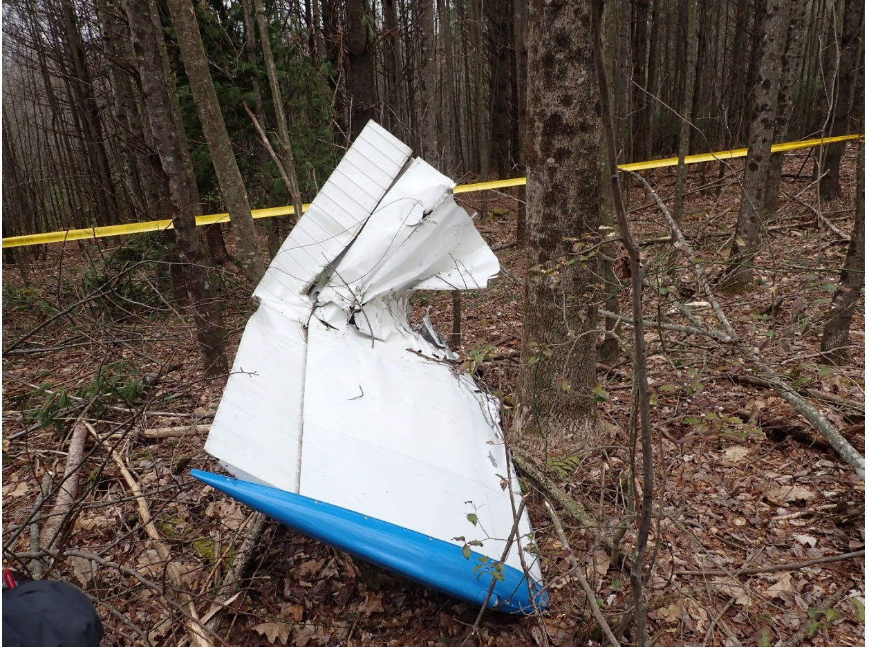
Figure 7: Impact separated left wing section
