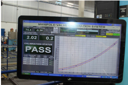
Figure 37 View of the Test Results of the Manifold Valve, Injector Lines and Injector Nozzles Operational Testing
