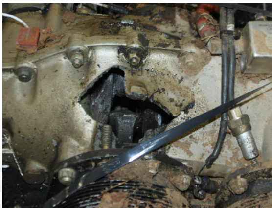
Figure 17 View of Hole in Crankcase
