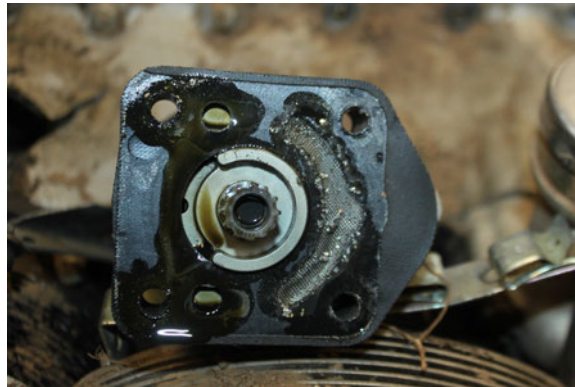
Figure 23 View of the Contamination on the Screen of the Propeller Governor
