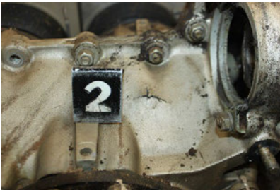
Figure 19 View of the Damage to the Crankcase Above the No. 2 Cylinder
