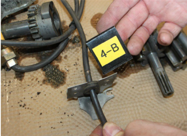
Figure 34 View of the Slight Chafing of the External Insulation of the 4B Ignition Lead.
