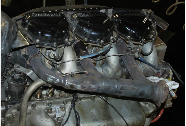
Figure 25 View of the Air Induction and Exhaust Systems of the Nos. 2, 4, and 6 Cylinders
