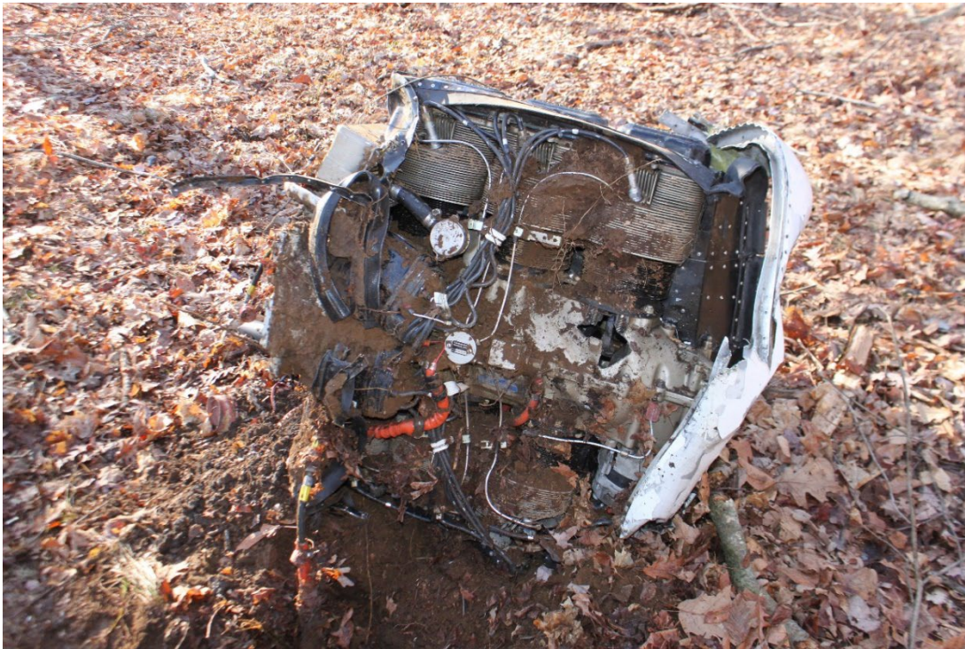
Figure 4: View Depicting the Engine After Rolling Out of its Impact Resting Spot Note the hole in the Crankcase at the No. 6 Cylinder Position.
