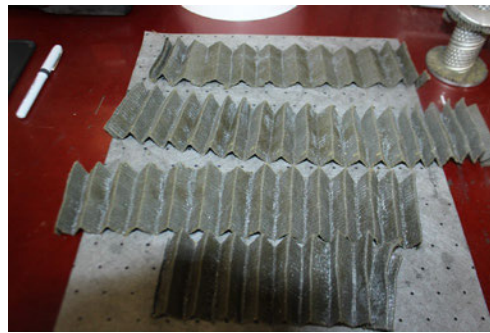
Figure 30 View of the Non-Ferrous Material in the Oil Filter Element
