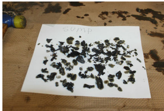
Figure 24 View of the Ferrous and Non-ferrous Material Found in the Oil Sump
