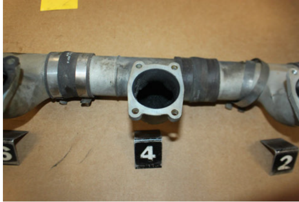
Figure 26 View of the Flange of the No. 4 Cylinder Intake Elbow Note the lack of Discoloration
