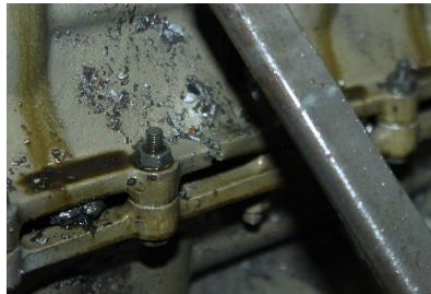
Figure 20 View of the Crack in the Crankcase In-Line with the Nos. 3 and 4 Cylinders
