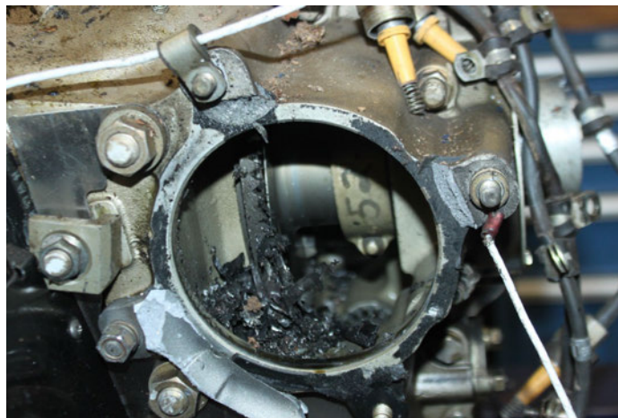
Figure 22 View of the Contamination Inside the Alternator
