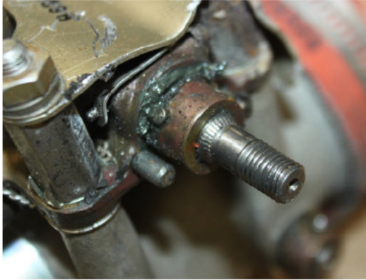
Figure 40 View of the Deformed Serrations of the Mixture Control Shaft
