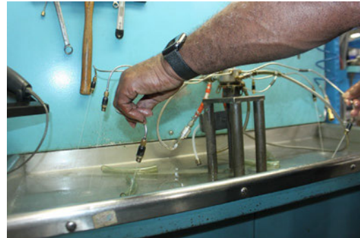
Figure 38 View of the Spray Pattern of the Fuel Injector Nozzles During Operational Testing
