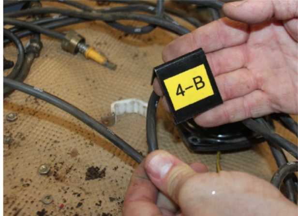
Figure 35 View of the Slight Chafing of the External Insulation of the 4B Ignition Lead.
