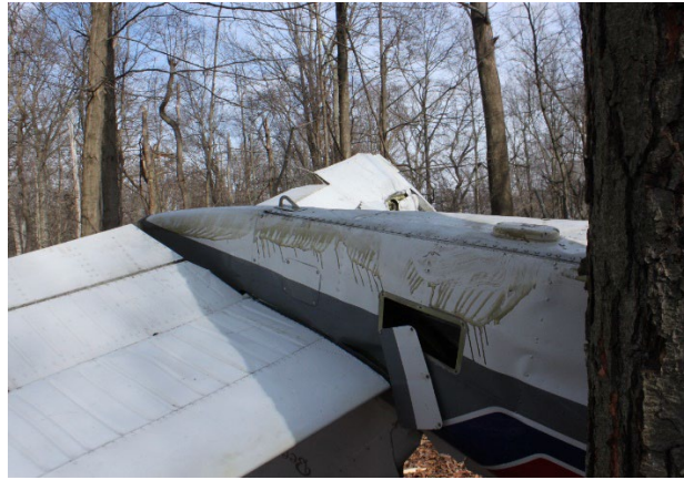
Figure 2 View of the Bottom Portion of the Fuselage Near the Tailcone. Note the Fresh Oil Clinging to the Bottom Fuselage Skin
