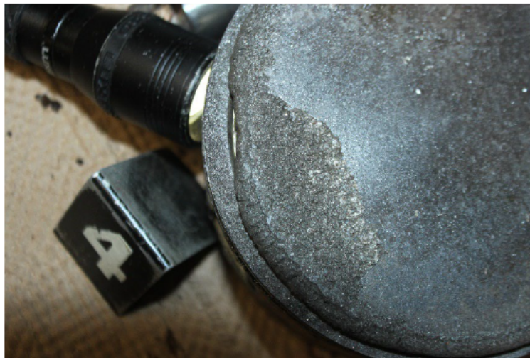
Figure 4 View Showing the Damage to the No. 4 Piston
