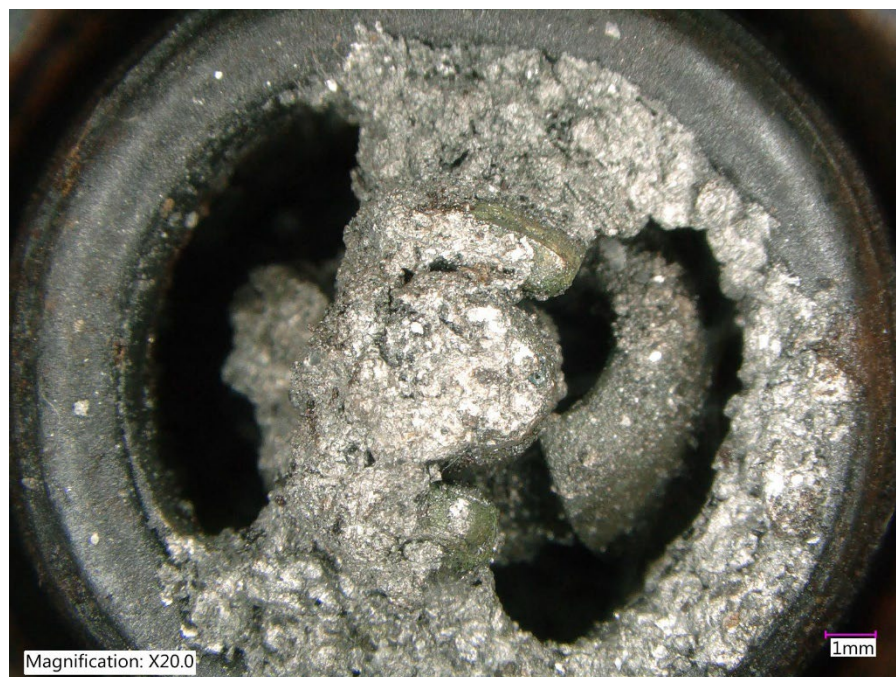
Figure 10 20 Power Magnification of the 4T Spark Plug
