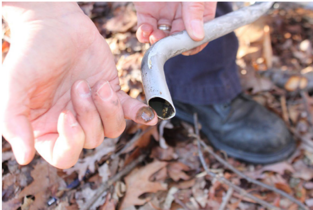
Figure 3 View of the Outlet of the Lower Crankcase Breather Line. Oil on Finger was from the Inner Surface Immediately Adjacent to the Opening. Note the Fresh Oil.
