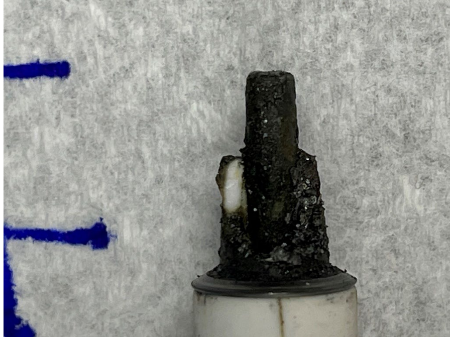
Figure 14 View of the 4T Spark Plug After Disassembly Showing Fractured Core Nose
