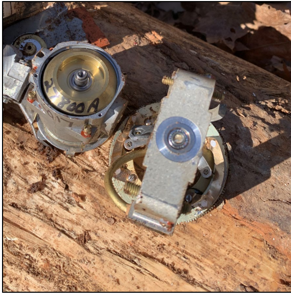
Photo 10: View of the directional gyro during disassembly by the investigation team.
