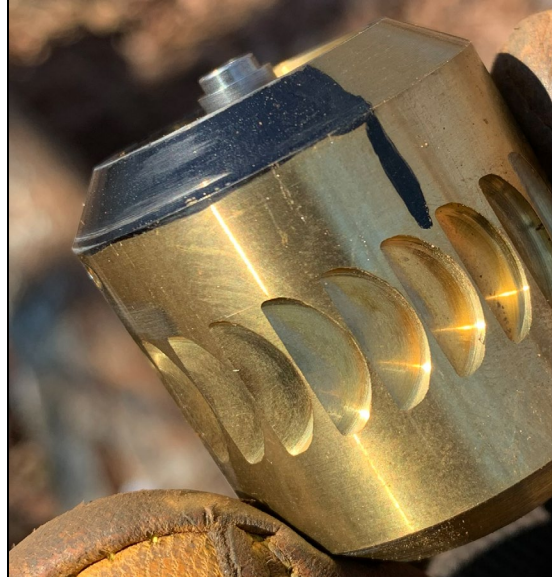
Photo 10: View of the directional gyro during disassembly by the investigation team.
