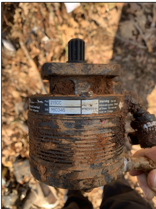
Photo 9: View of the vacuum pump after it had been removed from the engine by the investigative team.
