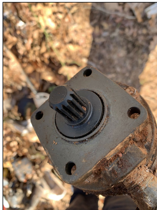
Photo 9: View of the vacuum pump after it had been removed from the engine by the investigative team.
