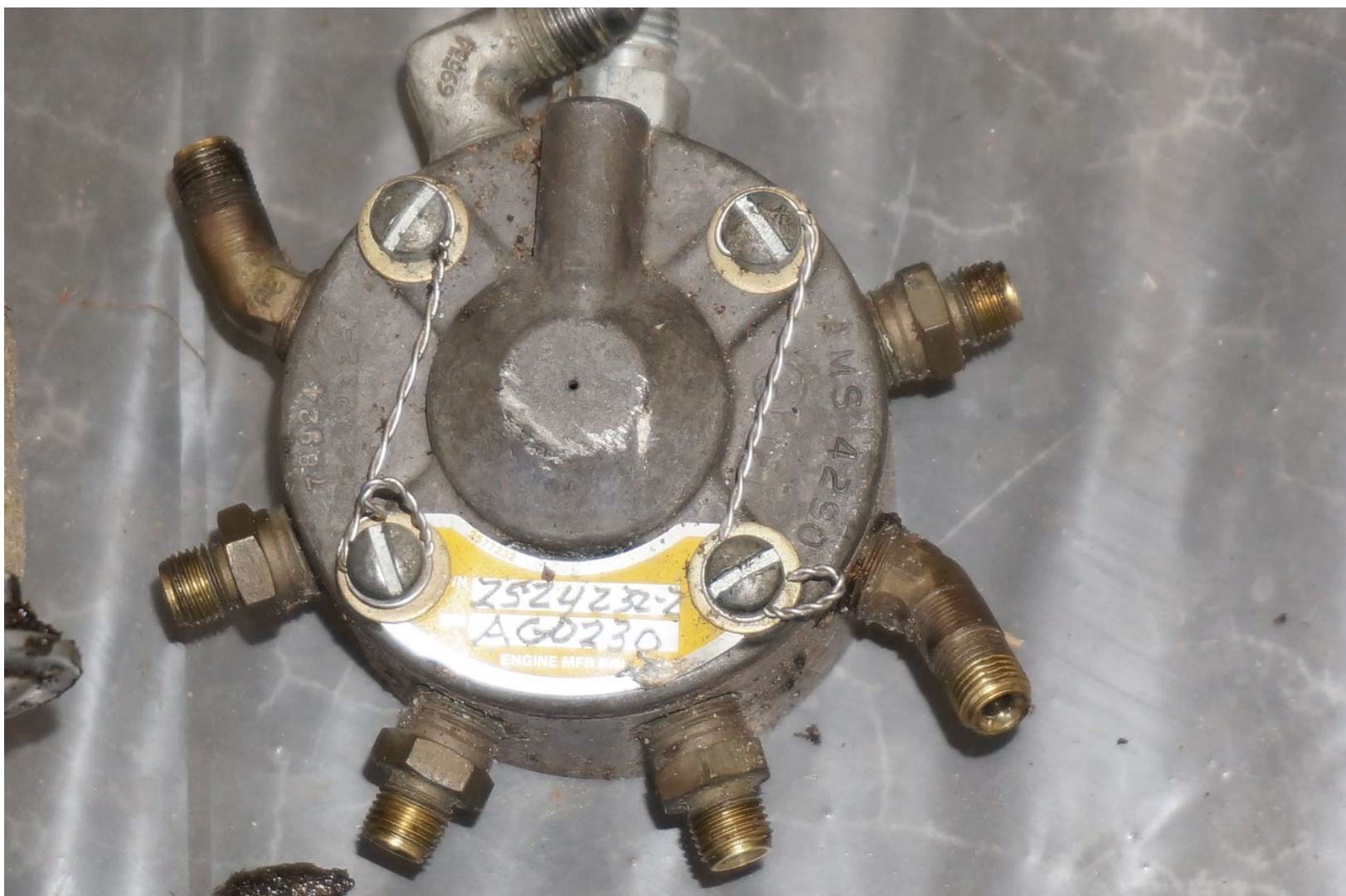
Photograph 15 - Fuel Distribution Manifold
