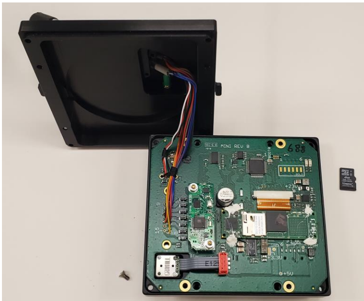
Figure 8. A microSD card was recovered from the inside of the GRT Avionics Mini EFIS. The microSD card is pictured to the right of the unit, after it had been removed.
