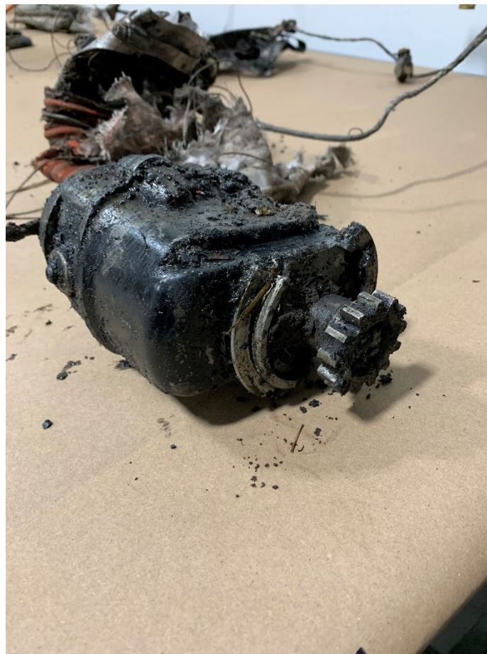
Figure 6 - Right-hand Magneto, Separated from Engine (NTSB)
