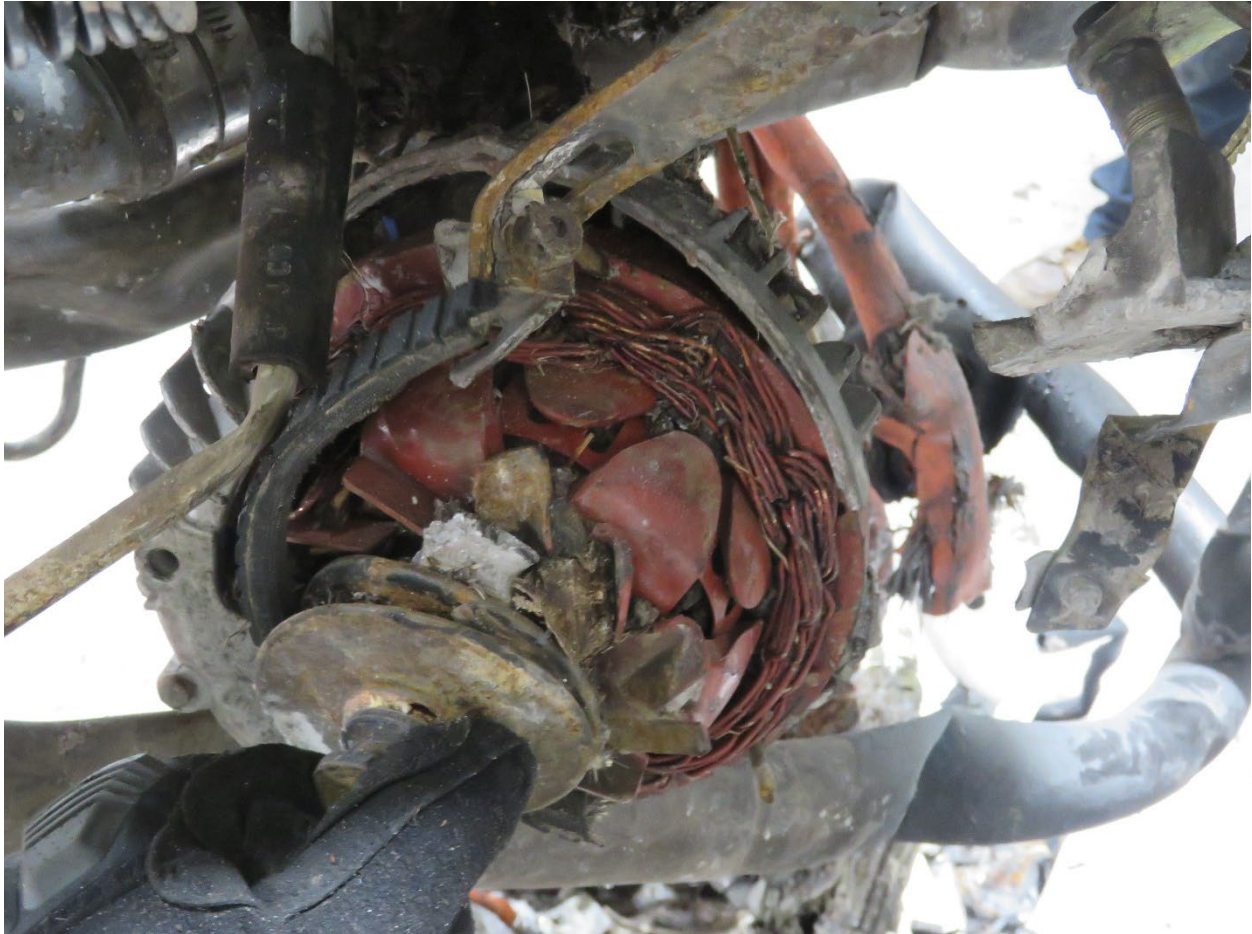
Figure 8 - Alternator, Damaged (Courtesy of Lycoming)
