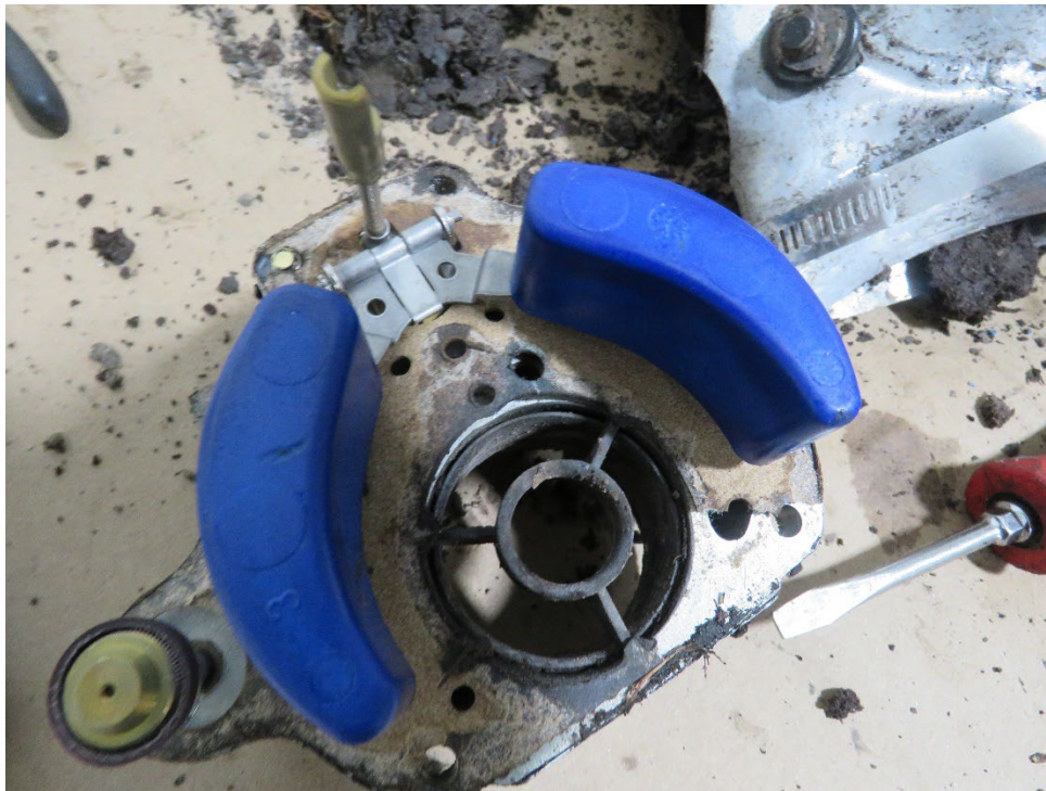
Figure 4 - Carburetor, Internal Floats (Courtesy of Lycoming)
