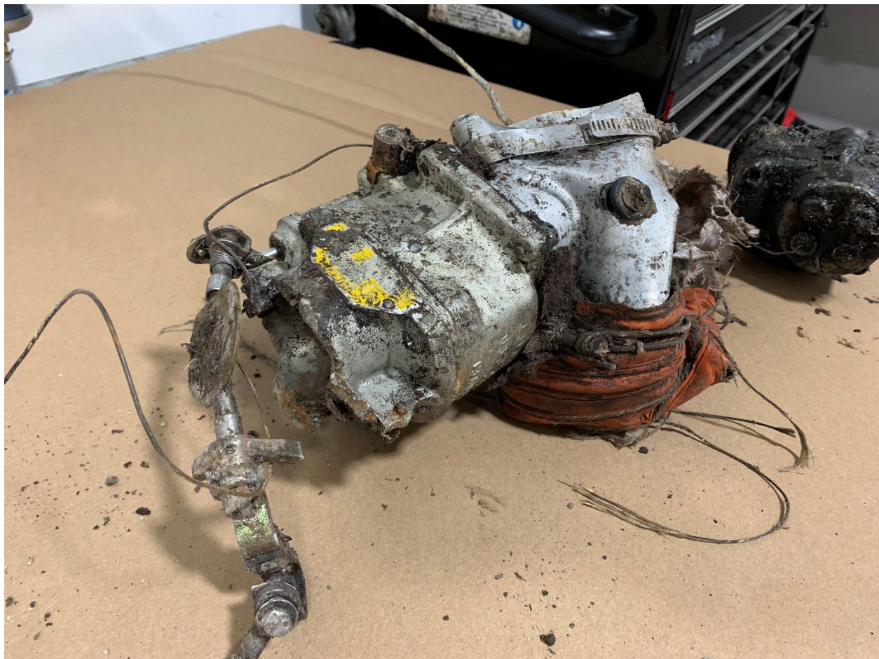
Figure 3 - Carburetor, Separated from Engine (NTSB)
