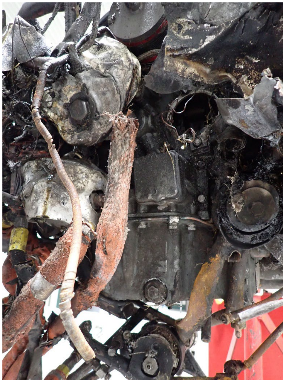
Photo 4 – Right Magneto Hold Down Nuts
