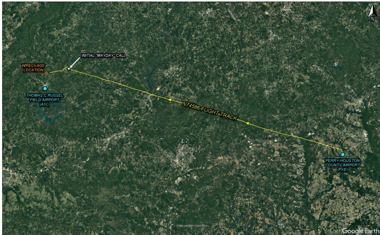
Figure 1. Overview of the entire accident flight track of N74586 overlaid onto satellite imagery.
