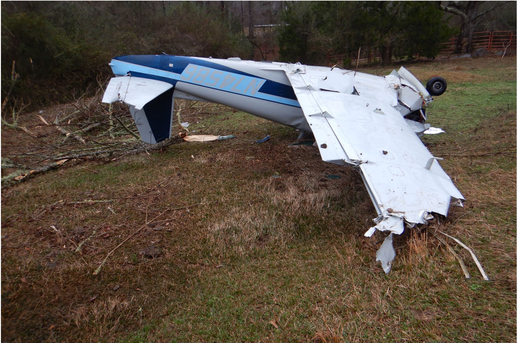
Photograph 3 - View of inverted airplane from left wing (note missing aileron and wingtip)
