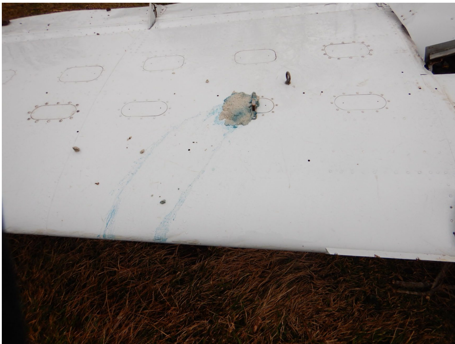
Photograph 10 - Fuel leakage from left wing fuel vent stopped with putty
