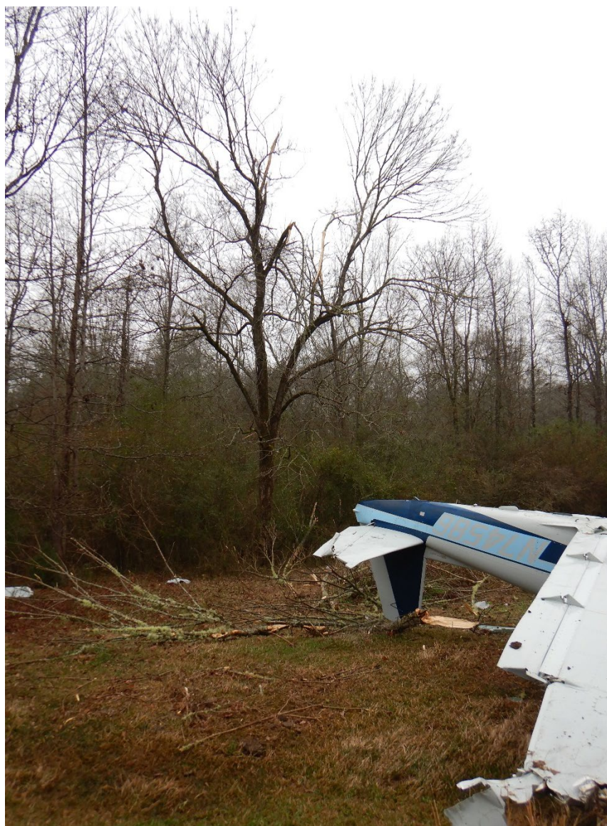
Photograph 5 - View of empennage, tree impact scars, and tree debris
