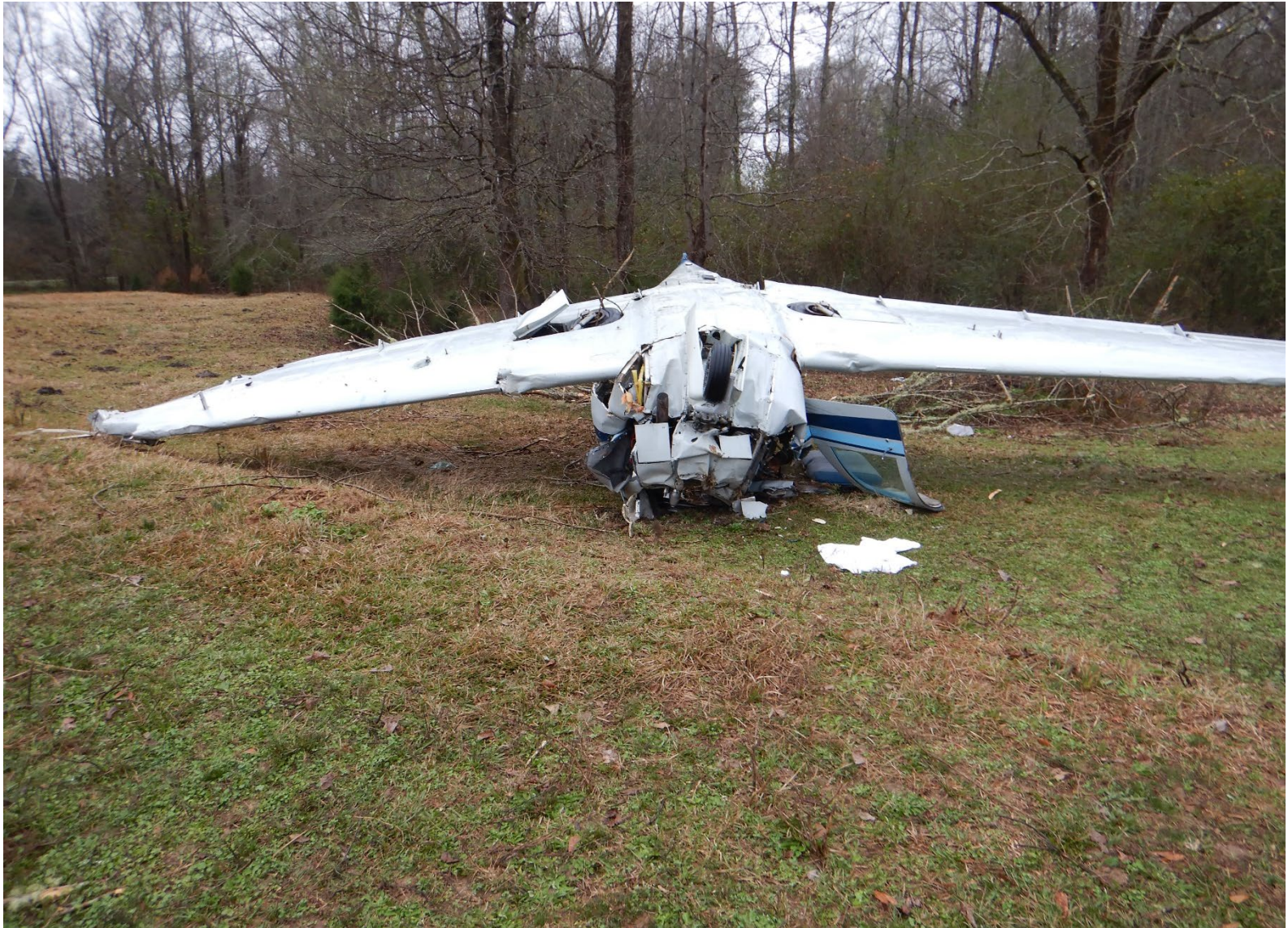
Photograph 4 - View of inverted airplane from front (note putty on left wing fuel vent to stop leakage)
