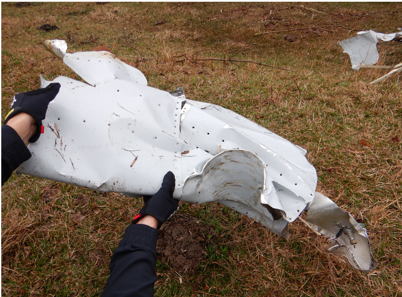
Photograph 9 - Left wing damage consistent with tree impact
