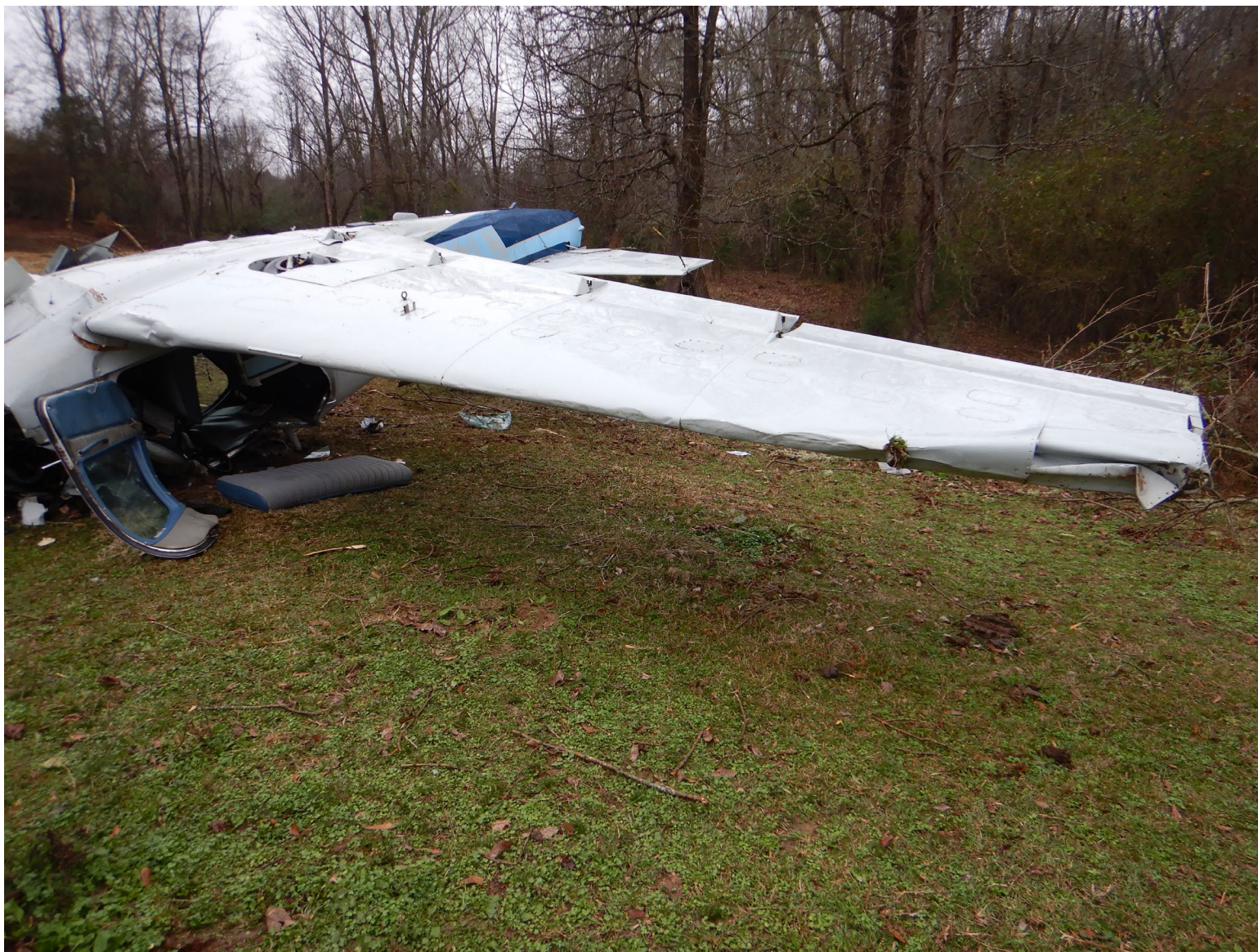
Photograph 12 - Right wing absent of any fuel staining
