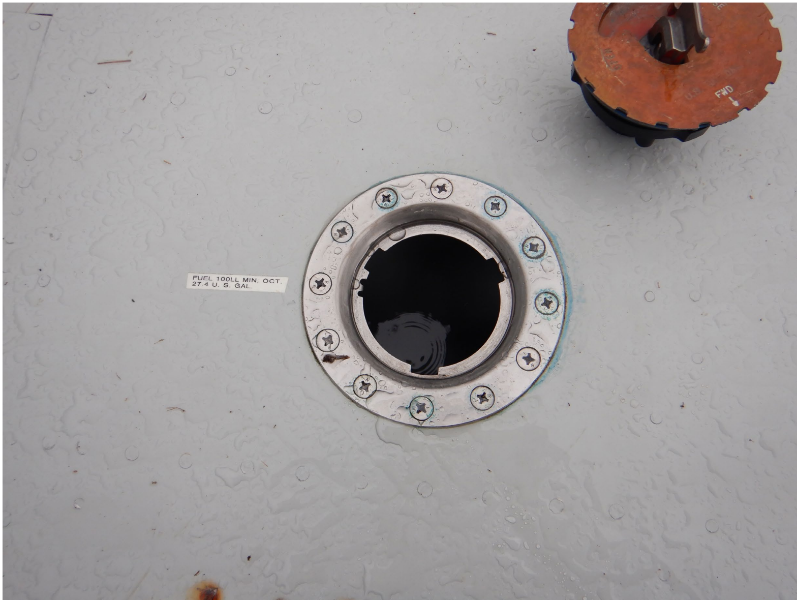
Photograph 11 - Left wing fuel bladder with visible fuel
