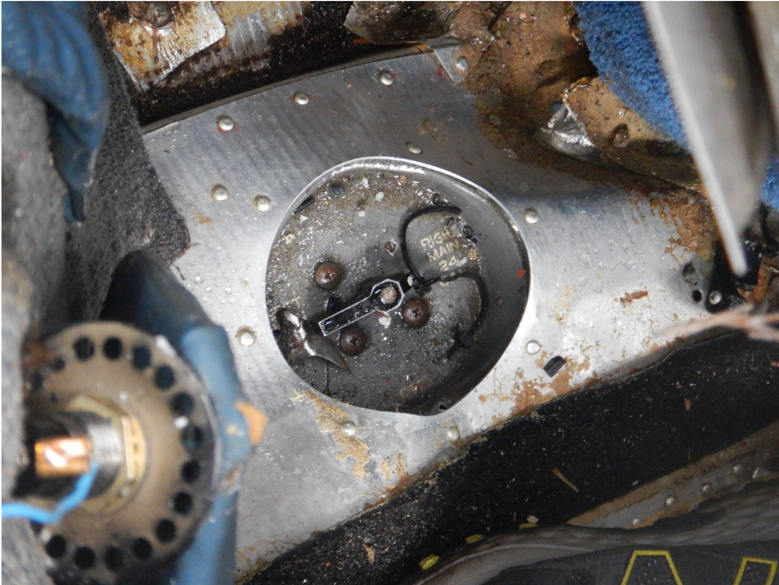
Photograph 14 - Fuel selector with right main tank selected
