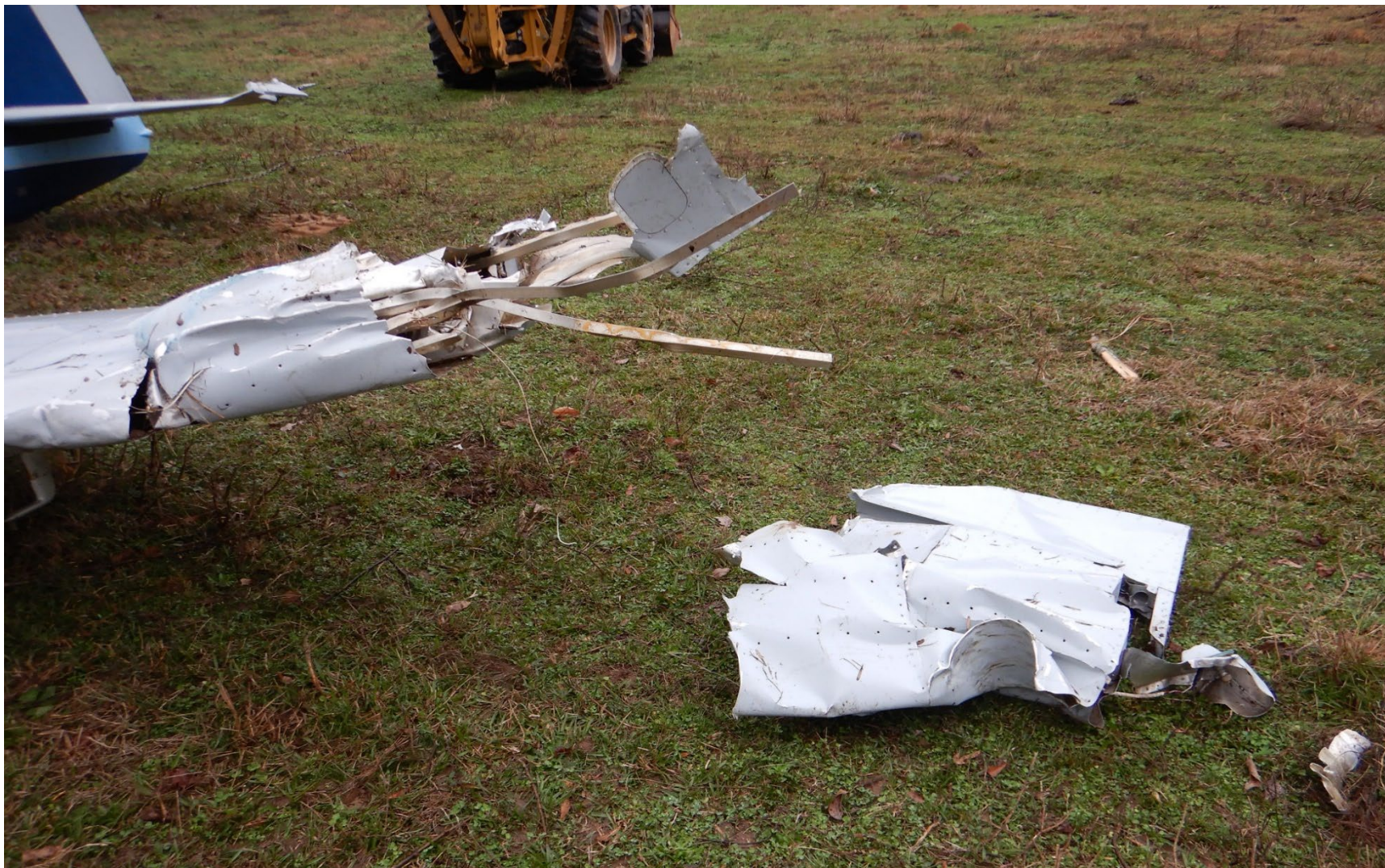
Photograph 8 - Left wing fracture with damage consistent with tree impact
