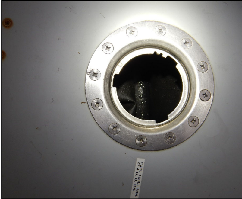
Photo 5 - Right wing fuel bladder with no fuel present.
