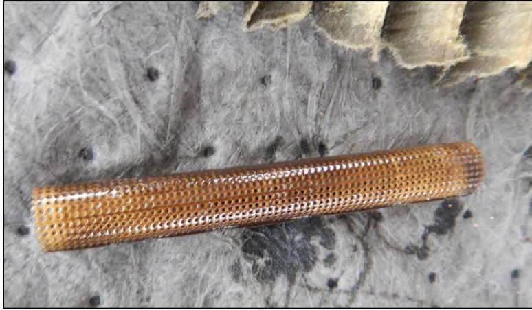
Photo 7 - Oil screen free from debris.
