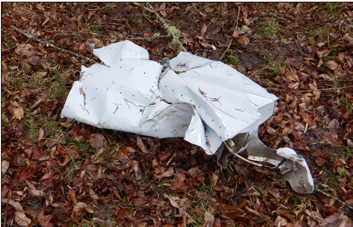
Photo 2- View of outermost left wing leading edge with damage consistent with tree impact.
