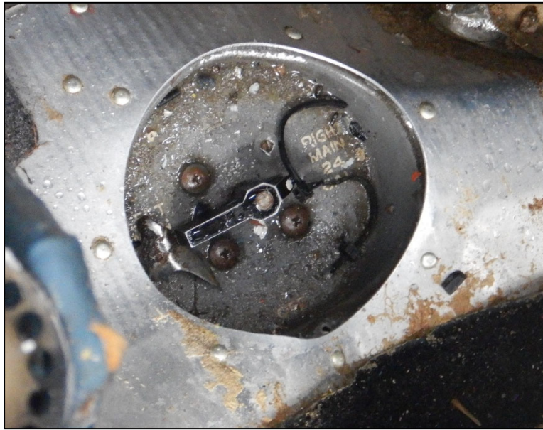
Photo 3 - Fuel selector selected to right main tank
