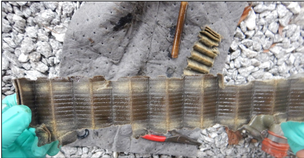
Photo 8 - Oil filter free of debris after removal from housing.
