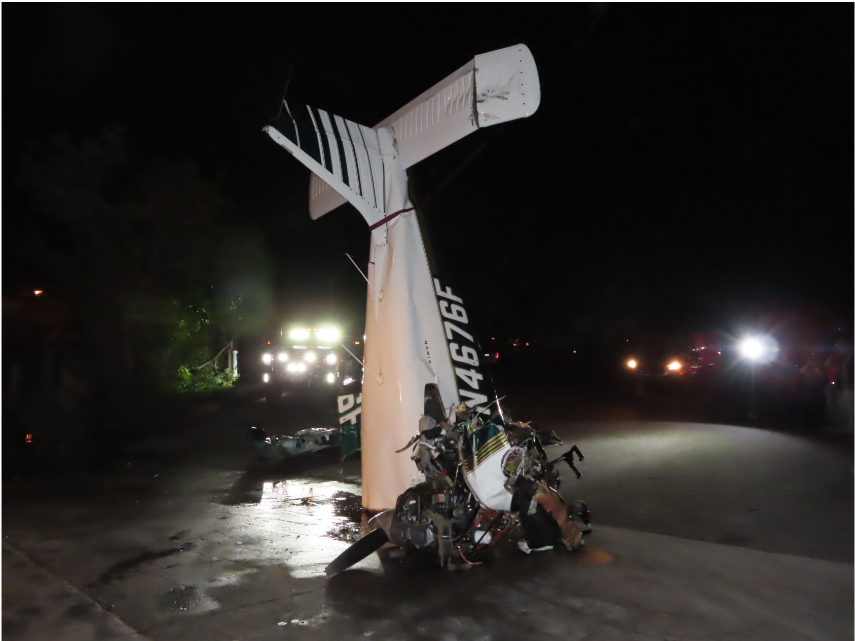
Photo 4 – View of Cabin, Empennage, and Tail Section at Recovery (Piper)
