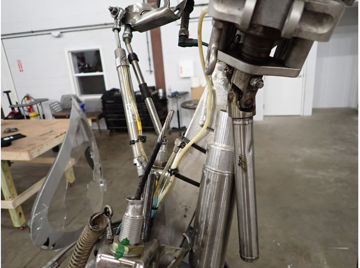
Photo 8: View of the mast head assembly.
