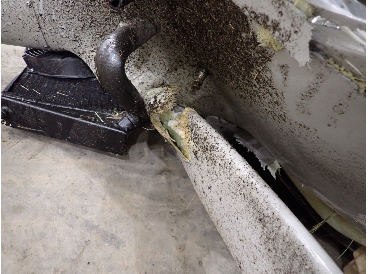
Photo 11: Twisting of left main landing gear.
