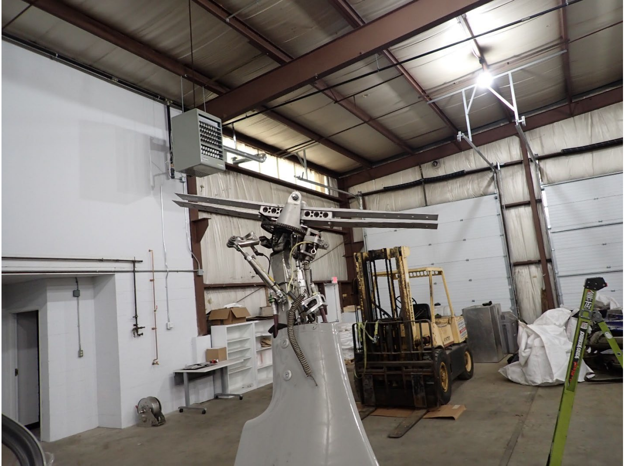
Photo 7: View of the rotor head attached to the mast with zip ties for examination.
