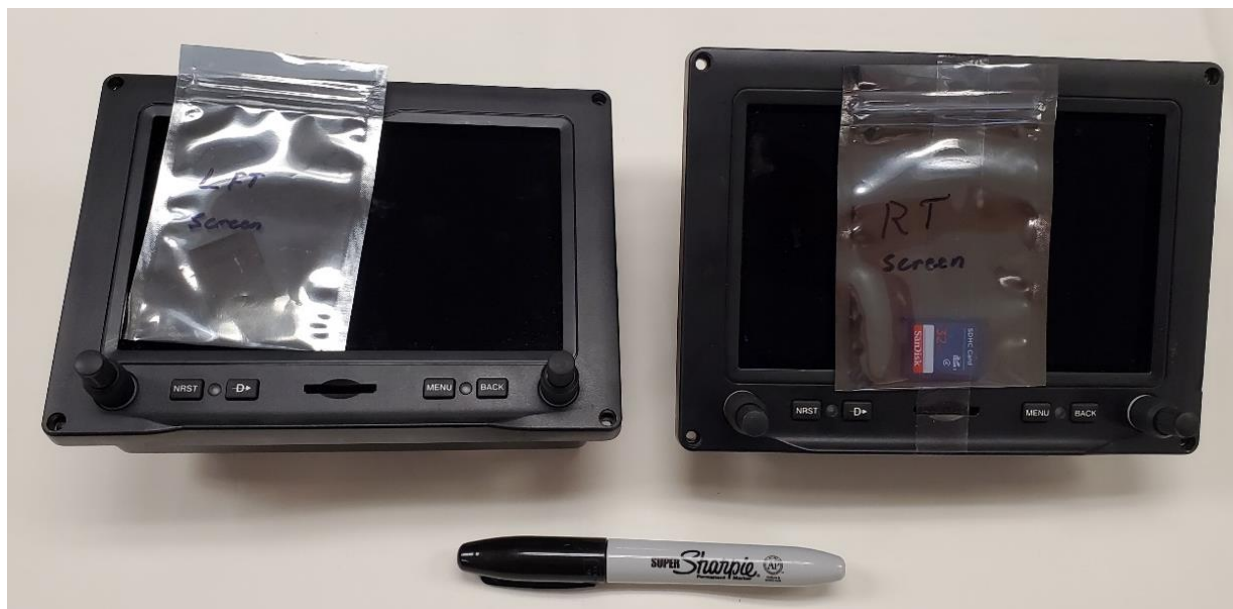
Figure 1. The two Garmin GDU 450 cockpit displays as received.
