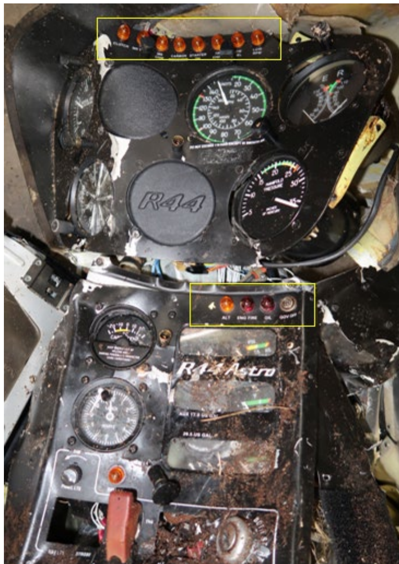
Figure 9. Caution and warning lights identified in yellow boxes.
