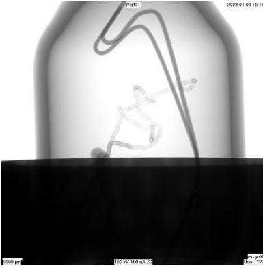
Figure 10. Radiograph of the alternator light.
