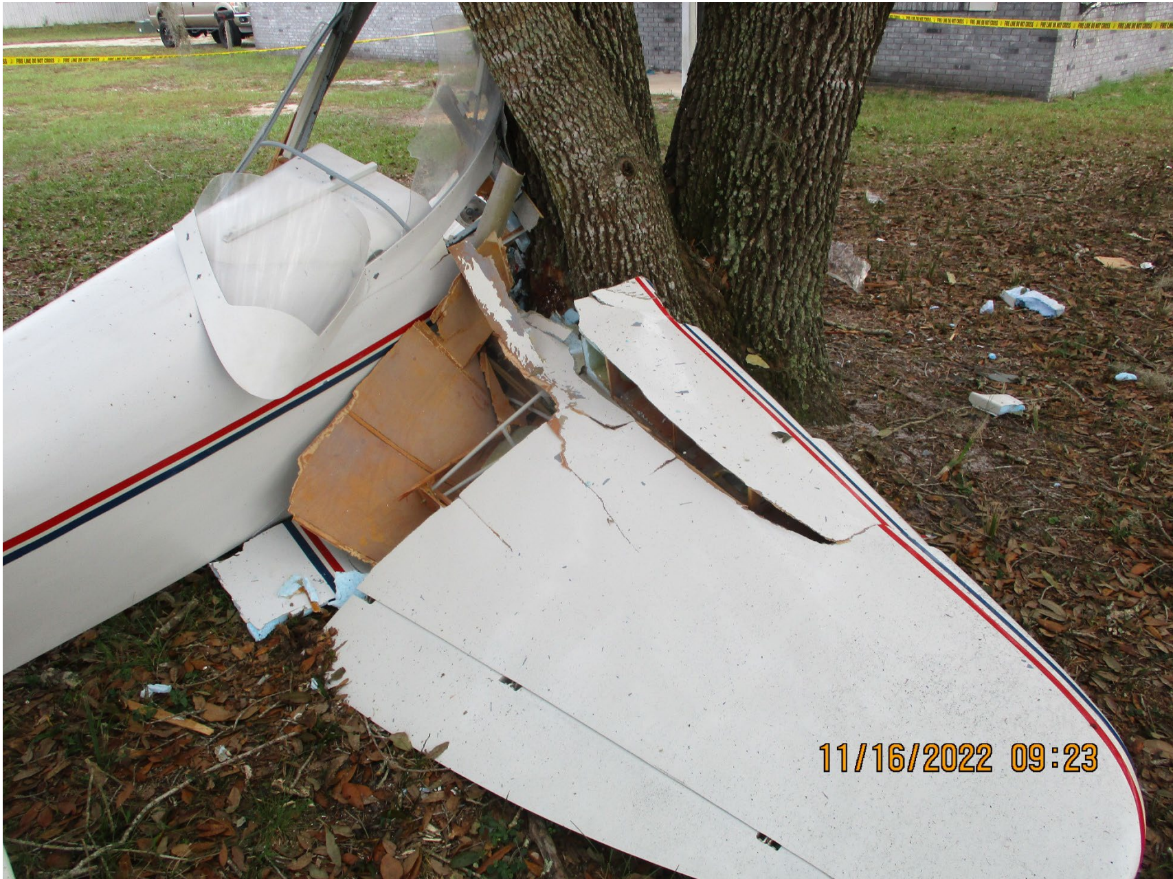
Photo 3 – Main wreckage, right wing view
