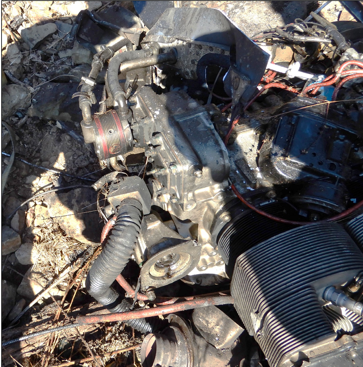
Photo 10: View of the vacuum pump attached to the engine, as found at the accident site.
