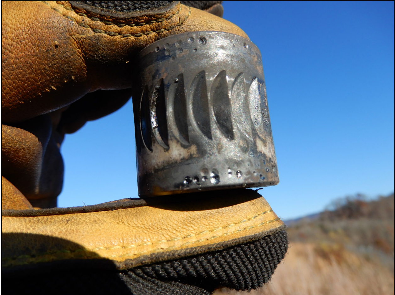
Photo 15: View of the attitude indicator gyro, as viewed during disassembly by the investigative team.
