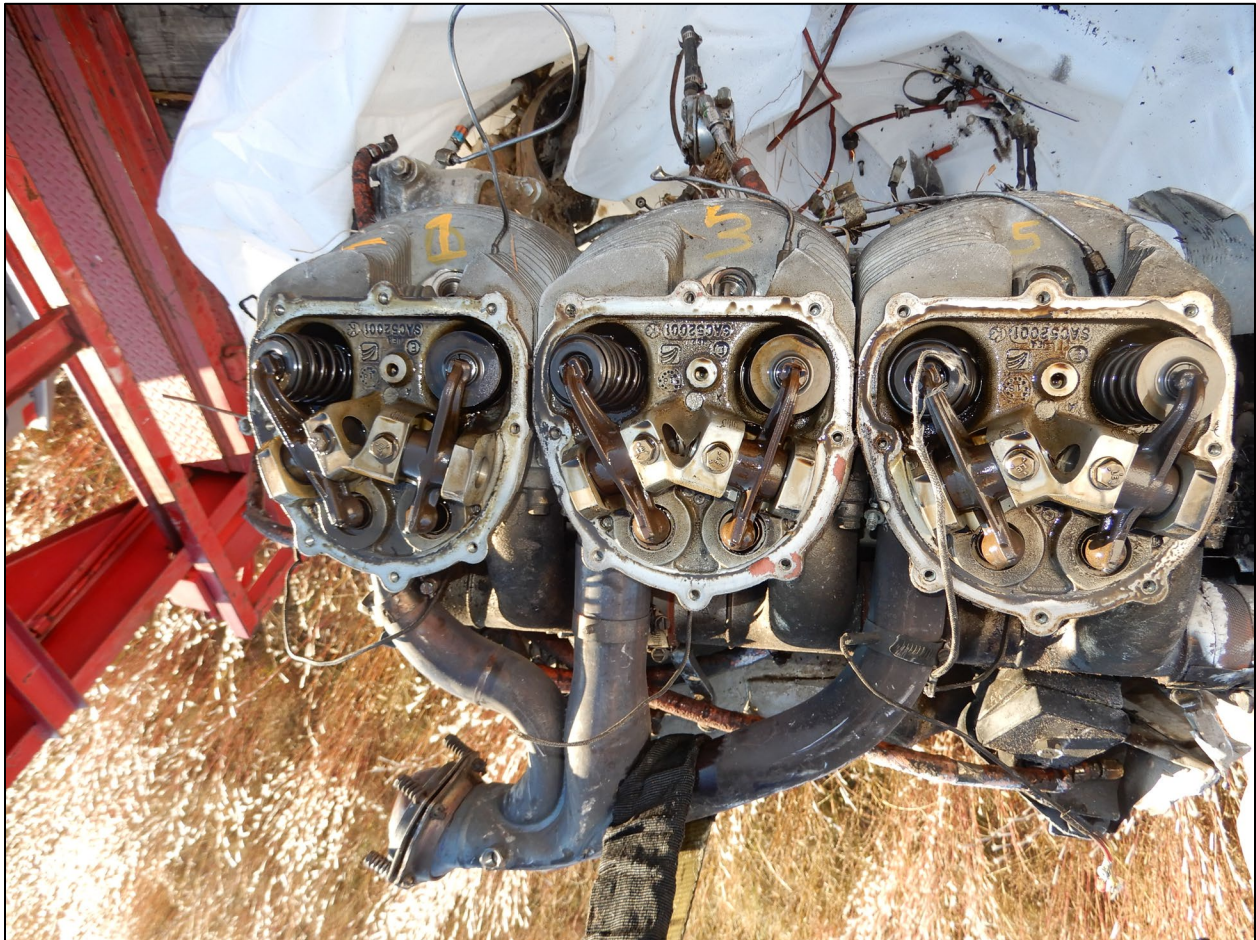
Photo 12: View of the Nos. 1, 3, and 5 cylinders partially disassembled by the investigative team.
