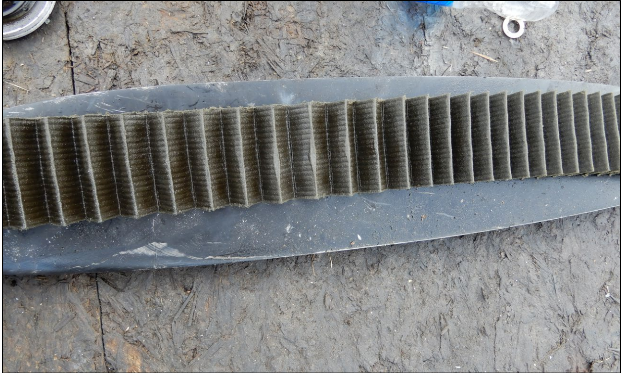
Photo 9: View of the engine oil filter as viewed during its removal and examination.
