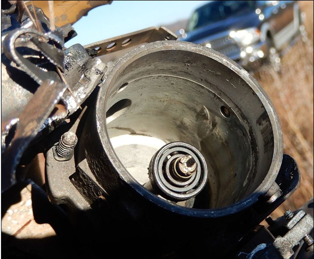
Photo 11: Internal view of the attitude indicator gyro housing. As viewed during its disassembly by the investigative team.
