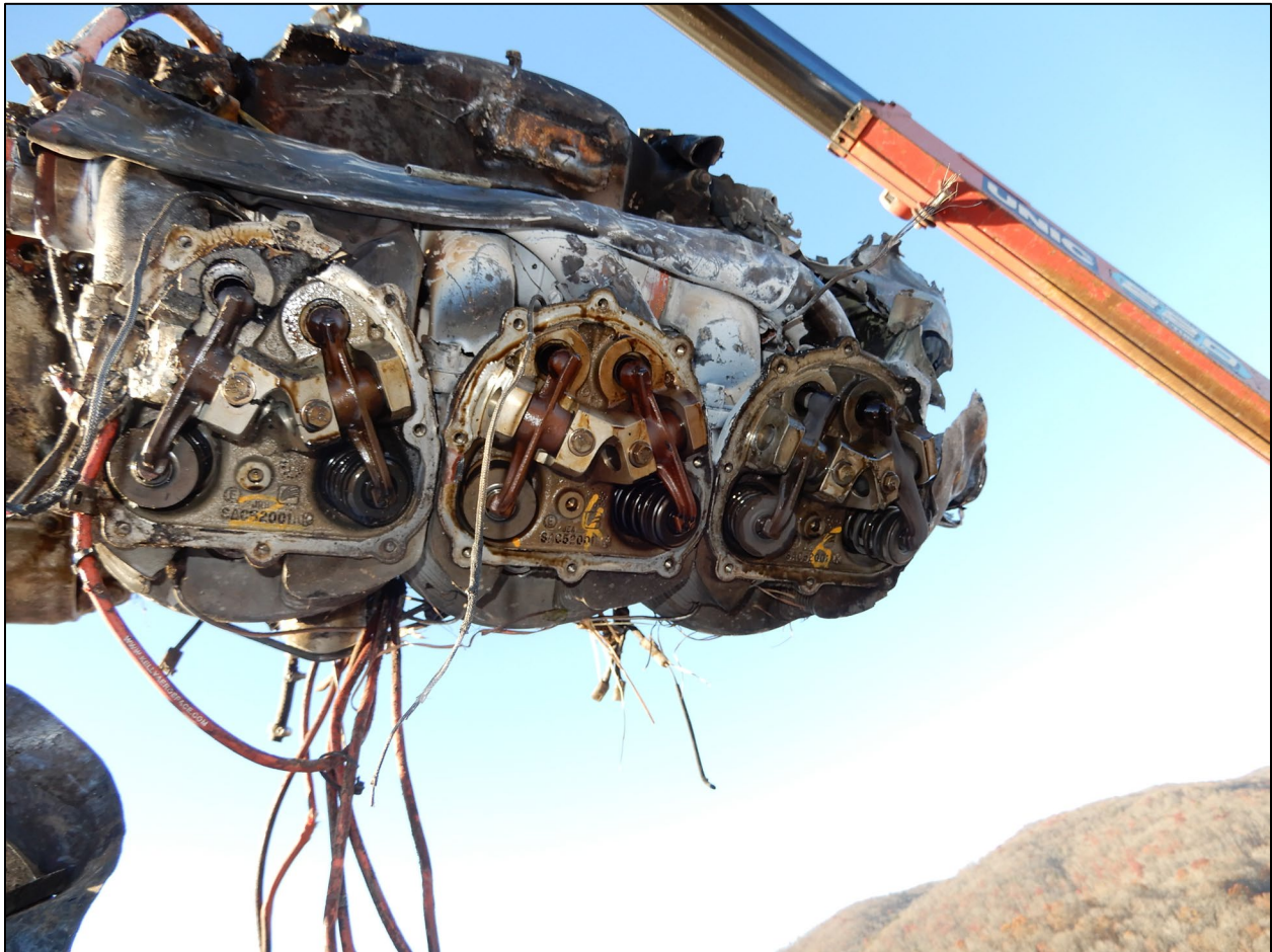
Photo 13: View of the Nos. 2, 4, and 6 cylinders partially disassembled by the investigative team.
