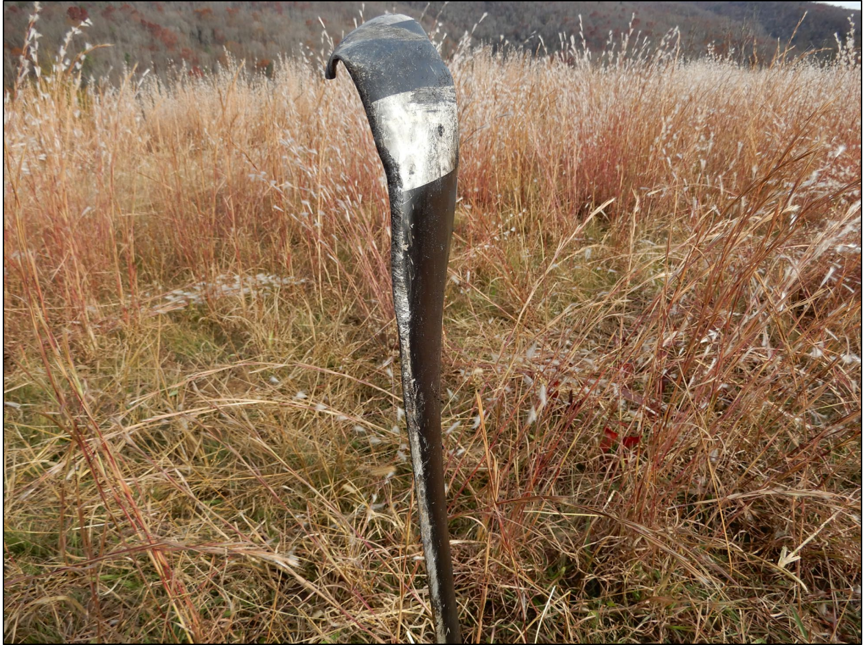
Photo 7: View of a propeller displaying tip curling and leading edge abrasions and gouging.
