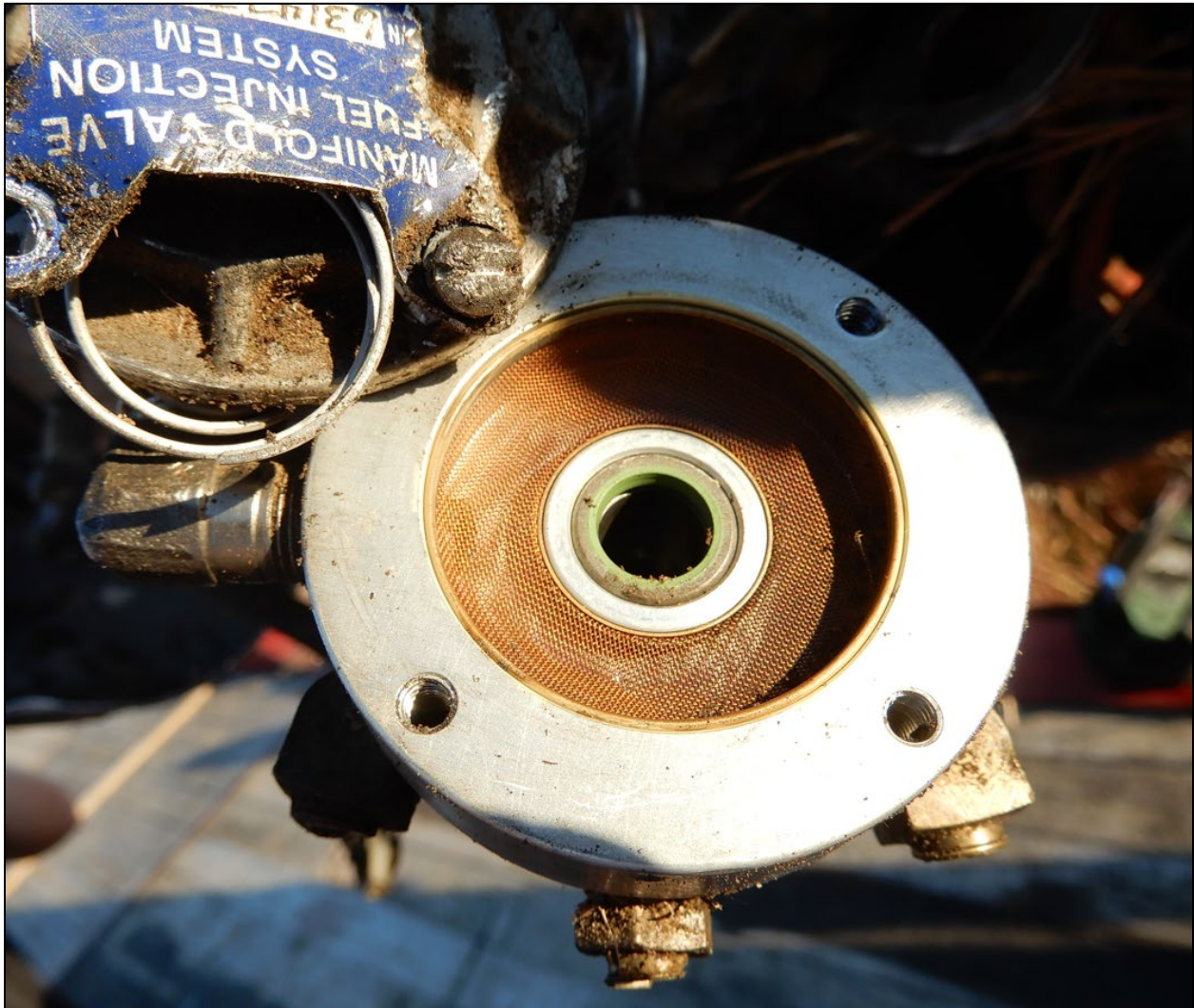
Photo 16: View of the fuel manifold filter screen, as viewed when disassembled by the investigative team.
