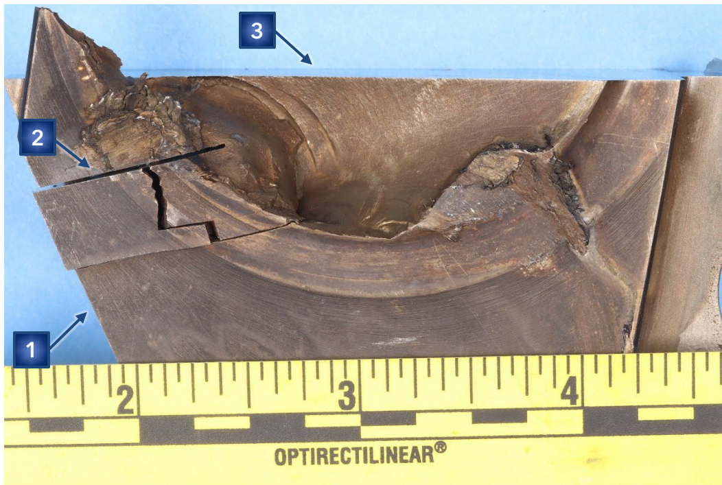
Figure 7. Crankshaft piece showing cuts made to separate unopened cracks and to facilitate SEM exam of the origin area. Numbered arrows point to saw cuts.
