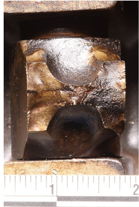
Figure 4. Lower end of the number 6 cylinder assembly (left image) with a trapped piston assembly and fractured connecting rod. The right image shows a closer view of the fracture surface on the number 6 connecting rod.
