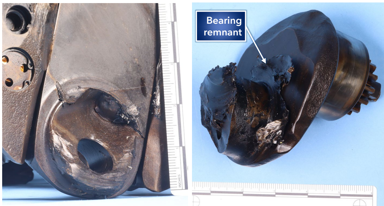
Figure 2. Mating sides of the crankshaft fracture at the number 6 connecting rod journal forward cheek showing the forward side in the left image and the aft side in the right image.
