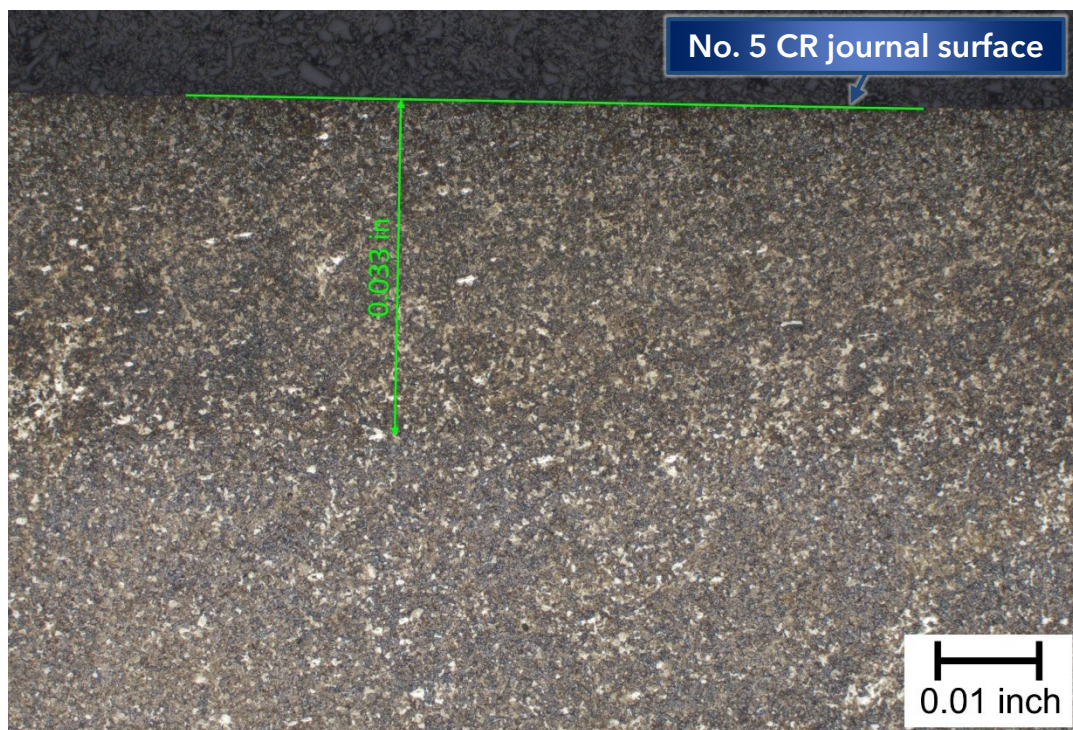
Figure 30. Nitride layer thickness at the number 5 connecting rod journal surface measured by optical means. Etched with Marble's reagent.
