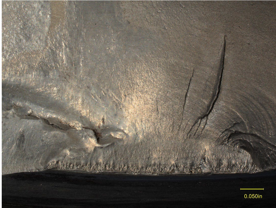
Figure 11. Close view of the origin area using a Keyence VHX-7000 in depth-up HDR mode.
