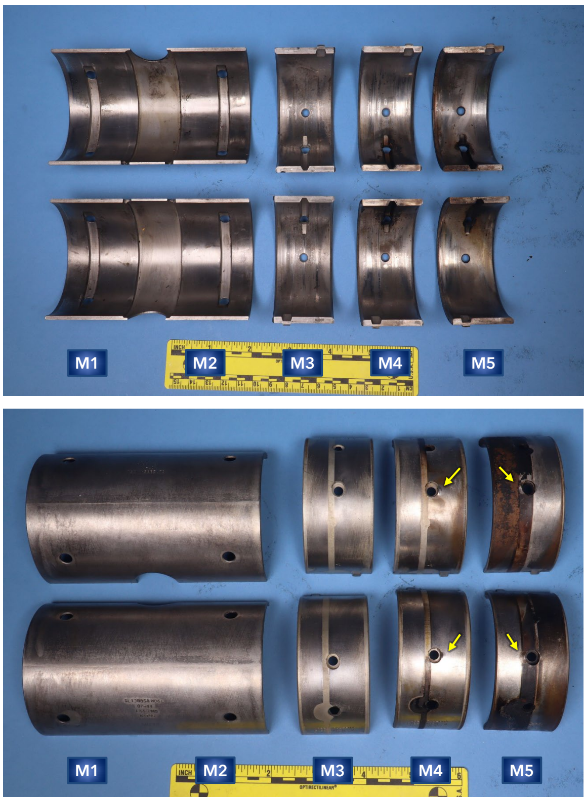
Figure 3. Views of the main bearing interior (upper image) and exterior (lower image) surfaces. Arrows in the lower image indicates elongation at the edges of the oil supply holes.
