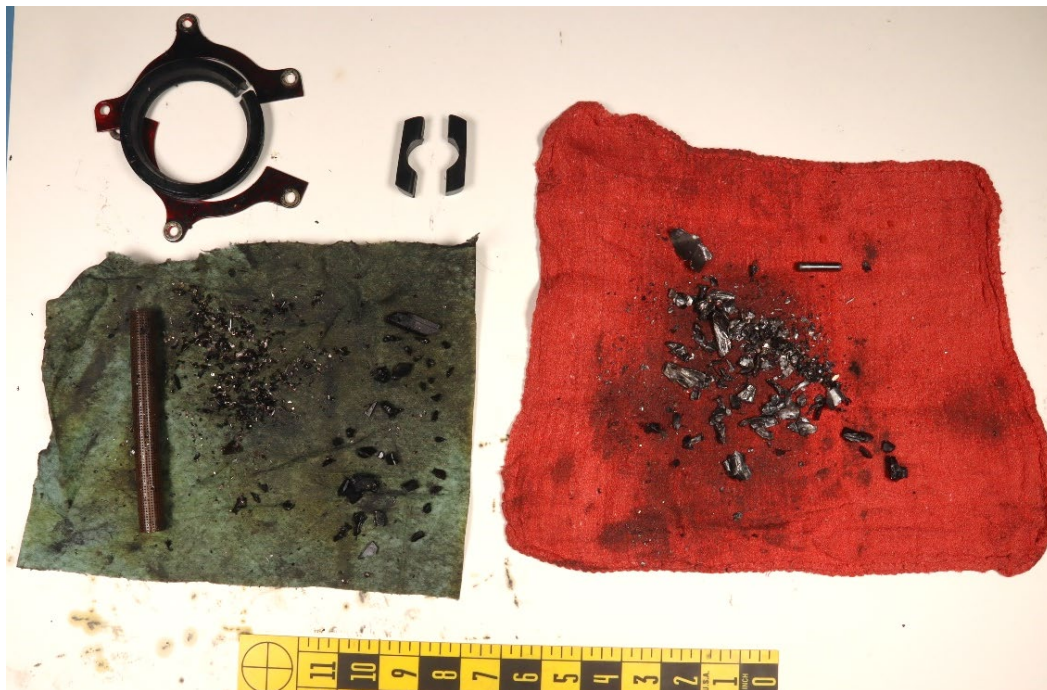
Figure 35. Oil screen and debris recovered from the oil screen (on the green cloth on the left) and debris recovered from the oil sump (on the red cloth on the right). The front seal and intact magneto bumpers are also shown above the green cloth.
