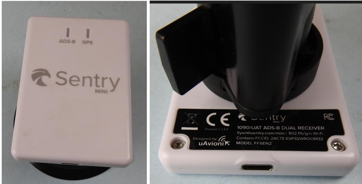
Figure 1. Front and back of the Sentry Mini ADS-B receiver as received.
