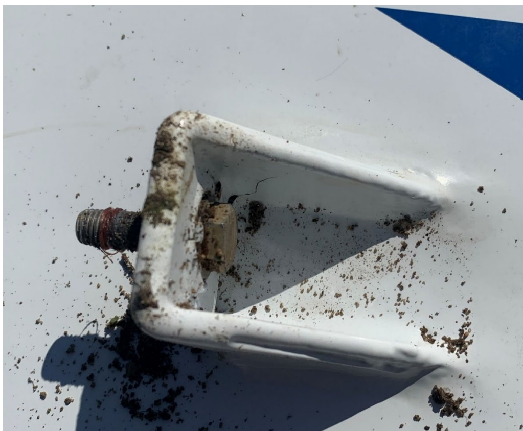
Figure 7. View of right wing strut attachment bolt as found.
