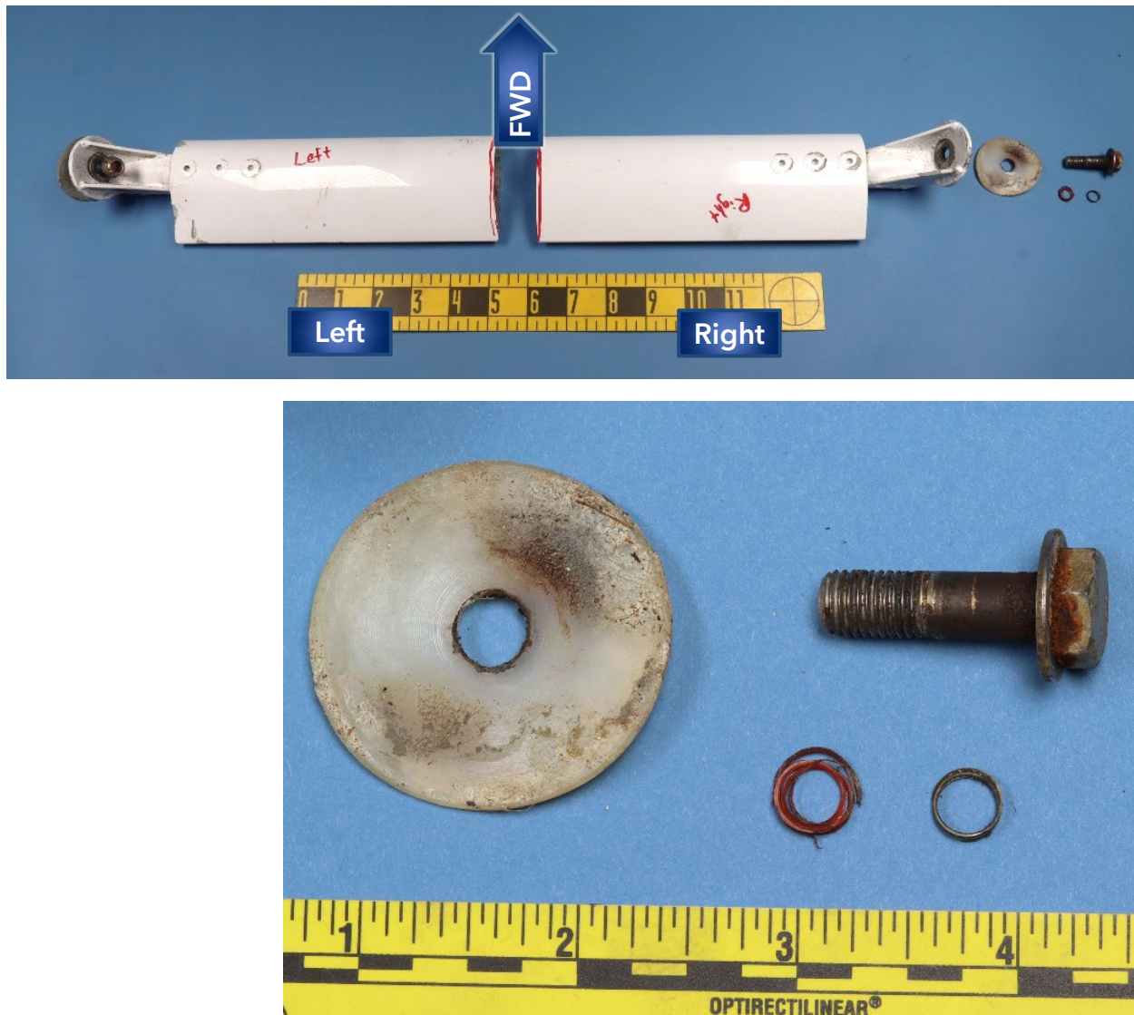
Figure 7. Outboard ends of the left and right wing struts with attachment hardware (upper image), and a closer view of the right wing strut outboard attachment hardware (lower image) as received for examination.
