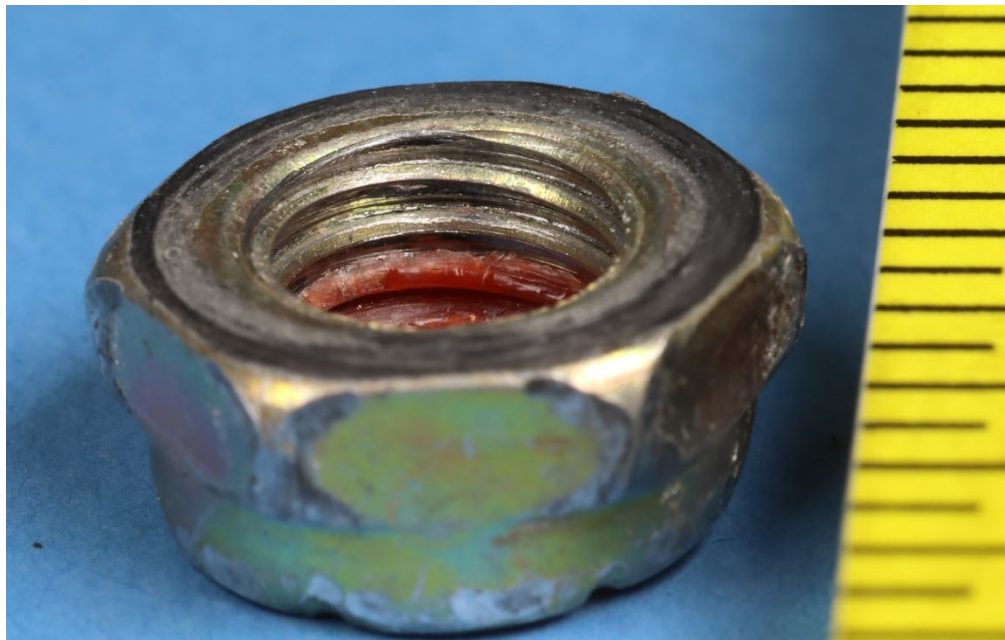
Figure 10. Macro photograph of the nut for the left wing strut outboard attachment showing 2 to 3 threads next to the red insert.
