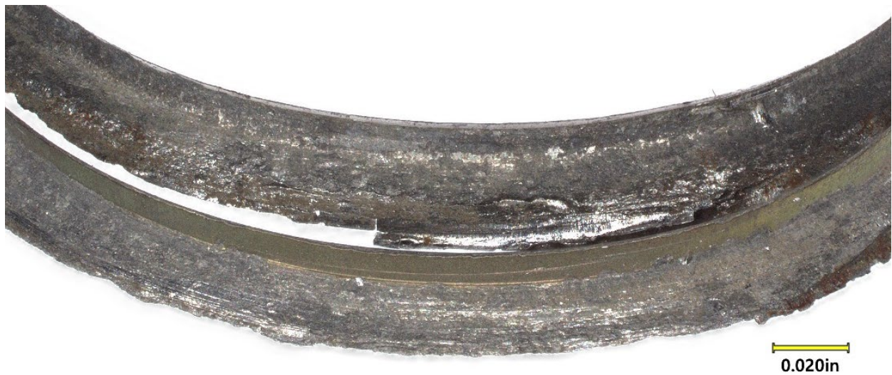
Figure 8. Fractured threads from the right wing strut outboard attachment nut after cleaning (upper image) as viewed looking at the bolt thread noncontact flanks of the nut threads. The lower image shows a close view of the bolt thread contact flanks on the nut thread piece with rough features consistent with repeated contact loading.
