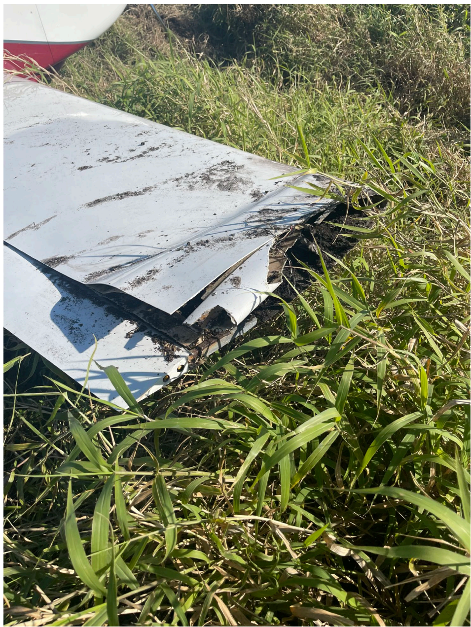
Photo 2 - Right Wing Damage (Pilot Photo)
