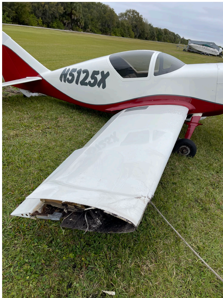
Photo 4 – Right Wing Damage (Pilot Photo)
