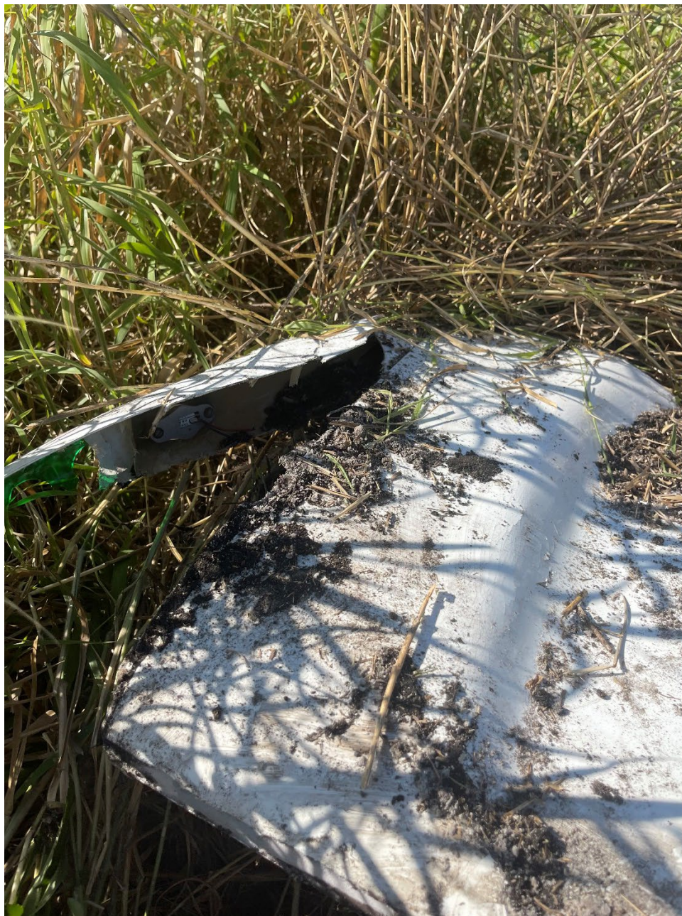
Photo 3 – Right Wing Damage (Pilot Photo)
